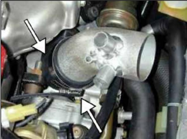
b. Install the supplied 1.75" to 2.25" reducing elbow onto the turbo inlet with the inlet pipe and hose clamps as shown.
