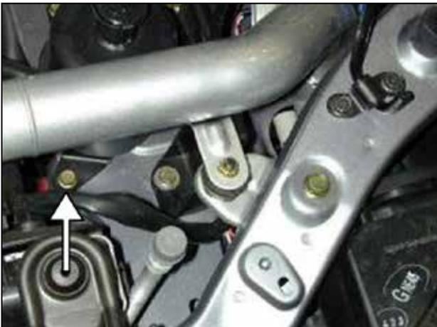
n. Remove the M6 bolt on the power steering reservoir bracket in preparation to install the AEM® heat shield. The M6 bolt will be reused in a later step.
