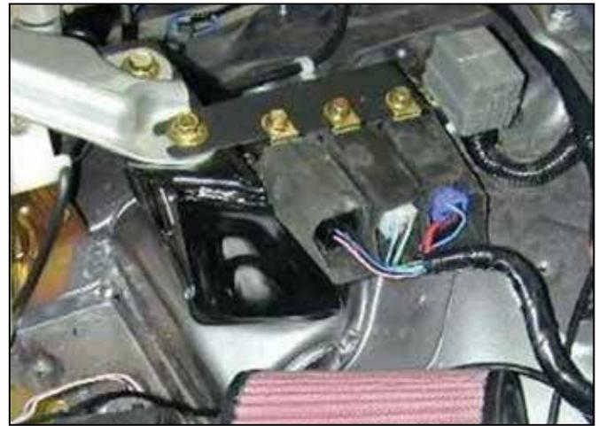
u. Attach the relays to relay bracket using the stock M6 nuts and bolts from the removal in step 2h as shown.
