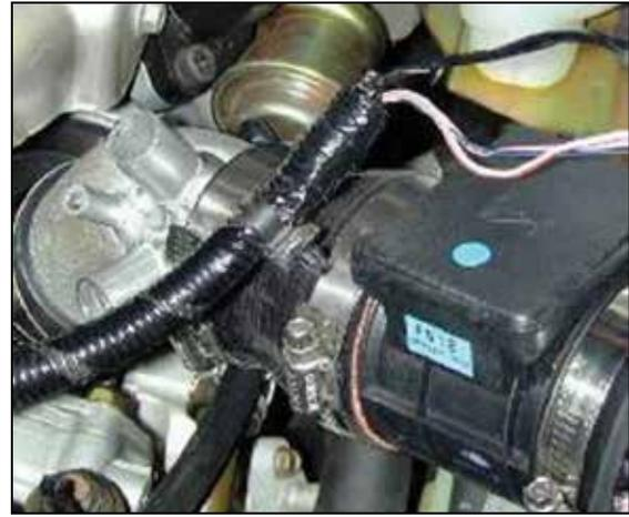
g. Remove the electrical tape as shown.
