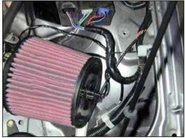
q. Install the air filter and tighten the hose clamp. Insert the IAT sensor into the hole in the end of the air filter. Attach the supplied 6" zip-tie to the IAT and relay harness as shown. Adjust the IAT harness so it does not contact the air filter.
