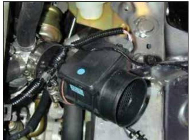
e. Install the MAF assembly from step 3c onto inlet pipe. The MAF bracket will install on to the rubber mount. Secure using the supplied M6 Nylok nut. Re-connect the MAF wiring harness to the MAF adapter assembly.
