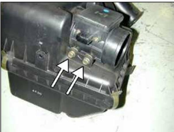
m. Remove the 2 10mm bolts holding the MAF sensor to the air box. Save the 10mm bolts for later use. Carefully slide the MAF sensor out of the air box.
