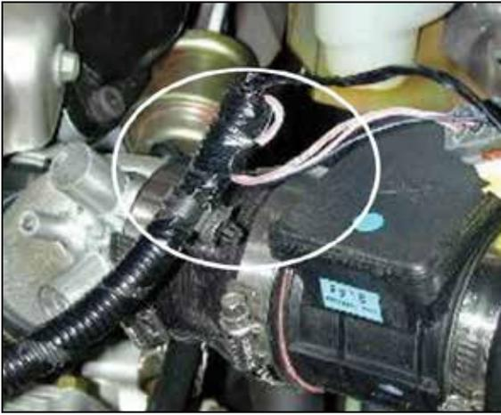
f. Cut the electrical tape holding the MAF sensor wires to the harness to free up additional length. BE CAREFUL AND ENSURE NO WIRES ARE CUT.
