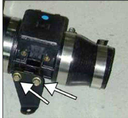
c. Assemble the supplied MAF bracket onto the MAF sensor as shown with the 2 M6 x 10 bolts removed in step 2I. Install the supplied 2.25" to 2.75" reducing coupler and hose clamps onto MAF sensor assembly as shown.
