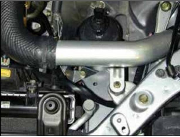
p. Align the heat shield over the hole on the power steering bracket. Install the M6 bolt removed in step 3n as shown. Check heat shield for clearance and tighten all 3 M6 bolts.
