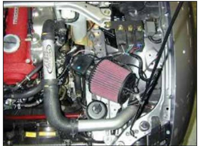
m. Install the supplied AEM® hot pipe using the front and rear stock elbow couplers removed in step 2j. Temporarily install the filter at this time. Check for clearance around the filter and tighten all hose clamps.
