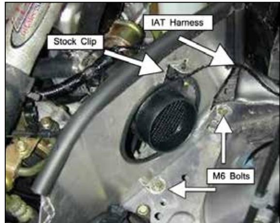
o. Remove the air filter. Install the heat shield using the 2 M6 x 15 bolts that were removed in step 2M. Do not fully tighten the bolts yet. Route the IAT sensor harness through the inlet opening as shown. Attach the stock clip on the harness to the tab on the heat shield as shown. Adjust the clips as needed so the harness is not in tension.
