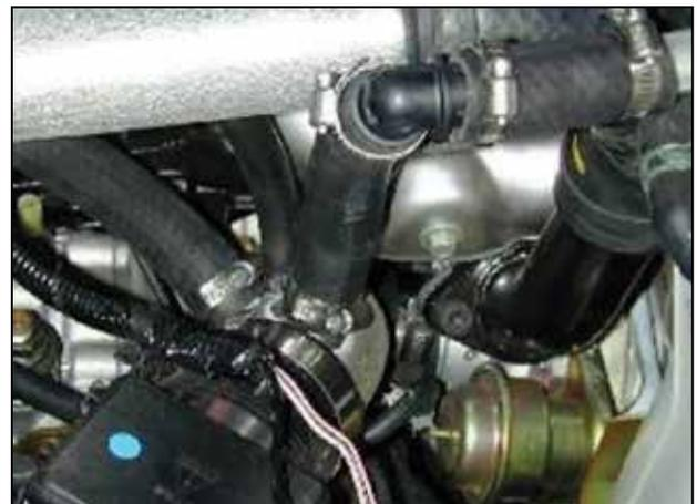
k. Install the supplied 3/4" and 5/16" hoses onto the inlet pipe as shown. Use the supplied spring clamps and screw clamps as shown.
