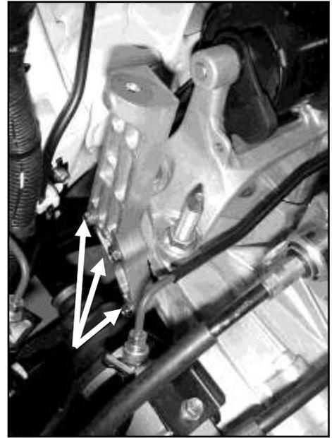
f. Loosen the three 10mm bolts, and remove the air filter box mount.
