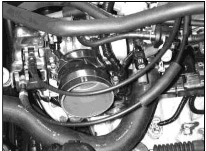
c. Install the included rubber reducer coupler onto the throttle body using the supplied No. 44 clamp, and place the No. 48 clamp over the large end of the coupler.
