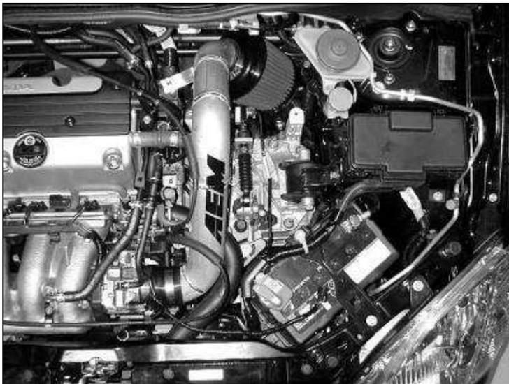
e. Install the intake pipe assembly, placing the reducer coupler over the throttle body. Also secure the bracket over the aluminum spacer with the included washer and serrated nut. Install the factory breather hoses over the nipples on the intake pipe.
