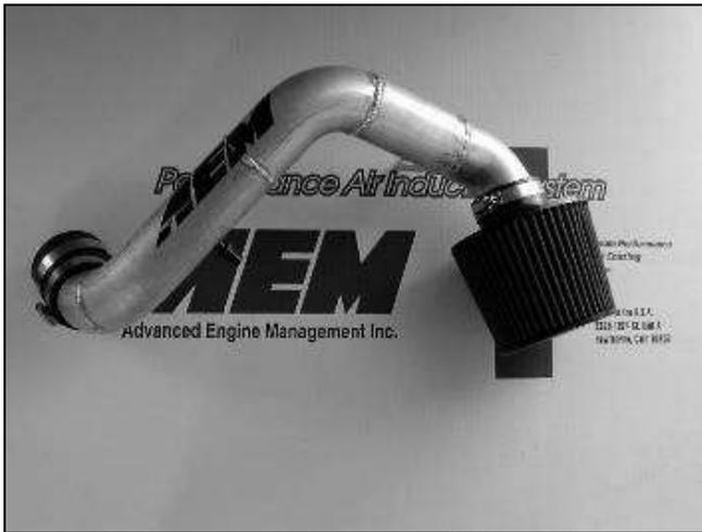
d. Install the air filter and reducer coupler onto the intake pipe using the supplied hose clamps, as shown.
