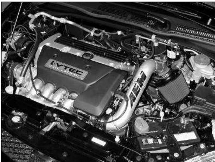
f. Install the intake cover, using the original bolts. Plug the IAT wiring harness back into the IAT sensor.
