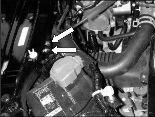
e. Loosen the two nuts securing the air tube, then remove it.
