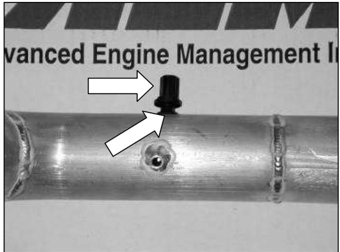
c. Install the included rubber grommet and the factory IAT sensor in the intake pipe.
