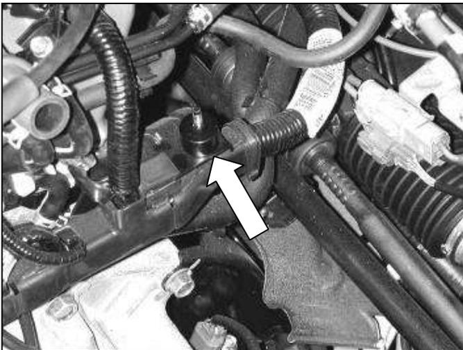
b. Install the included aluminum spacer on the factory air box mounting stud as shown.
