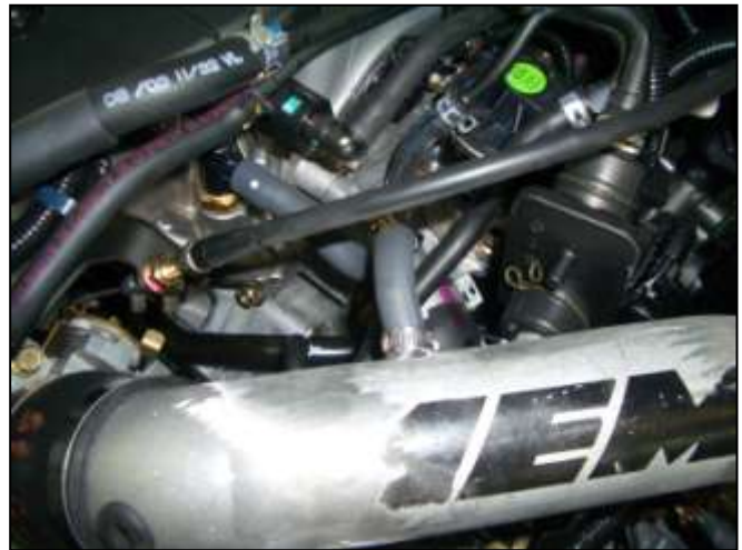
i. Install the small hose onto the AEM® intake system as shown. Use a \frac{3}{4} " hose clamp to secure it on the small nipple on the intake pipe.
