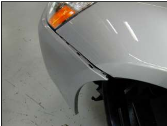
m. Unsnap the corner of the bumper cover as shown in the picture. This will help in removal of the resonator assembly.
