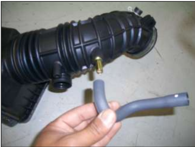
h. Remove the small hose from the factory intake system.
