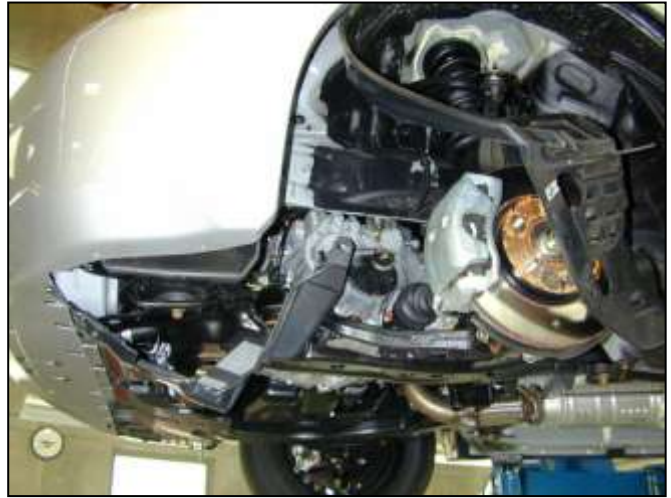
j. Tuck the splash guard out of the way behind the brake rotor.
