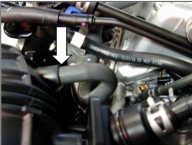
c. Remove breather hose from the inlet air tube
