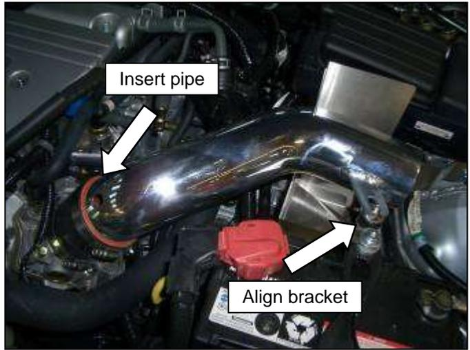
i. Insert the inlet pipe into the coupler. Align the inlet pipe with the rubber mount.
