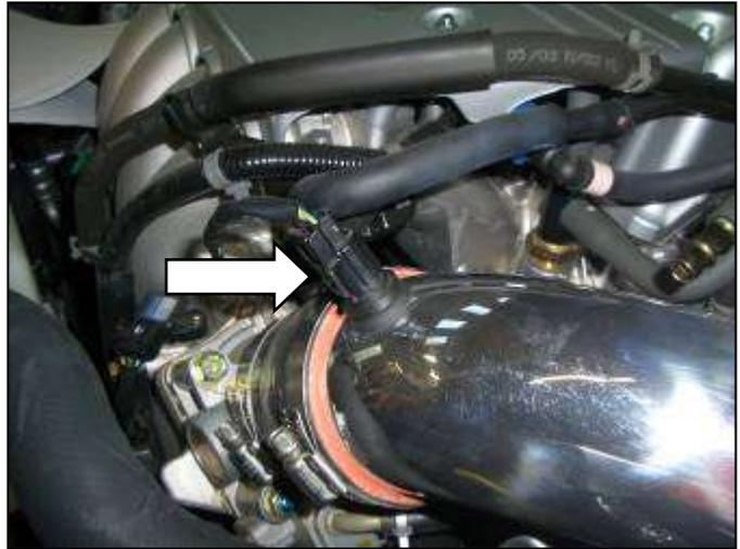
k. Insert Inlet Air Temperature (IAT) sensor.
