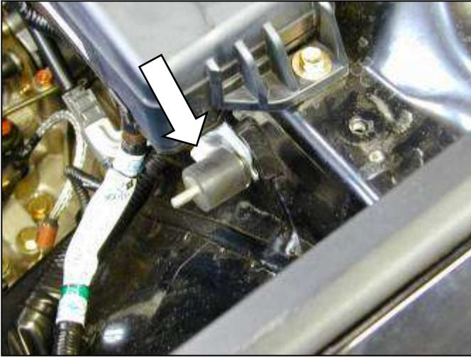
d. Insert 1" rubber mount toward the body. Tighten rubber mount to the bracket.
