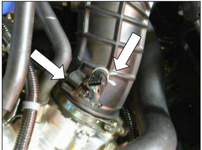
b. Squeeze the clamp holding the Inlet Air Temperature (IAT) sensor. Remove IAT sensor from inlet air tube. Remove wiring harness from the inlet air tube.
