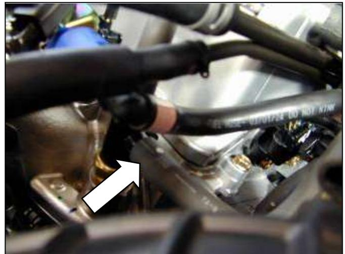
d. Disconnect the other end of the breather hose from step 2c. *Be careful not to damage the plastic nipple.*
