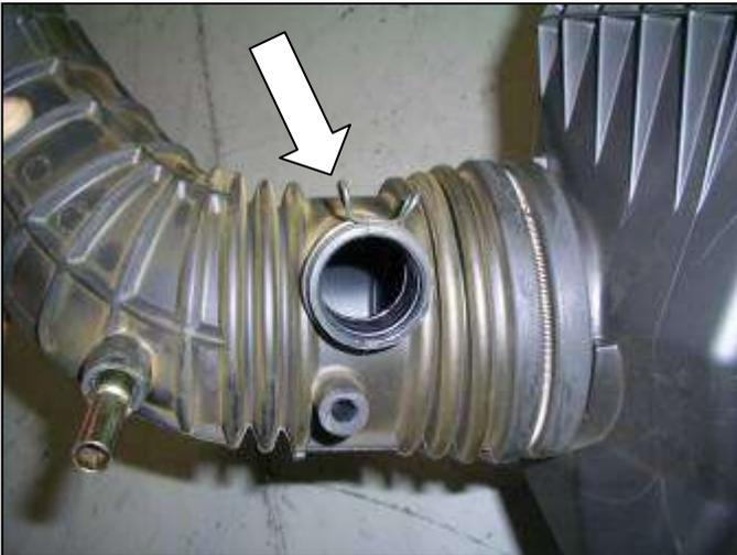
m. Remove the hose clamp from the stock inlet tube.
