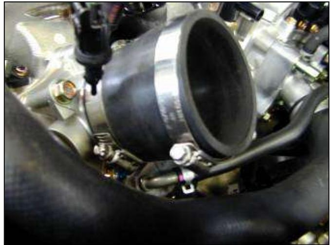
c. Attach reducer coupler with hose clamps as shown. Use the #44 hose clamp on the throttle body side and the #48 on the opposing side.
