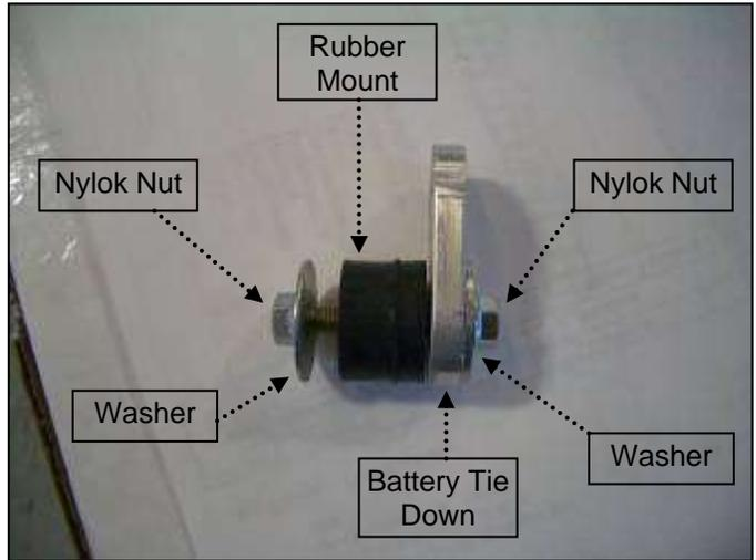
e. Assemble second rubber mount, 5/8". On one end attach fender washer and nylok nut, do not tighten. On the other end, attach the battery tie down, fender washer, nylok nut and then tighten hardware.
