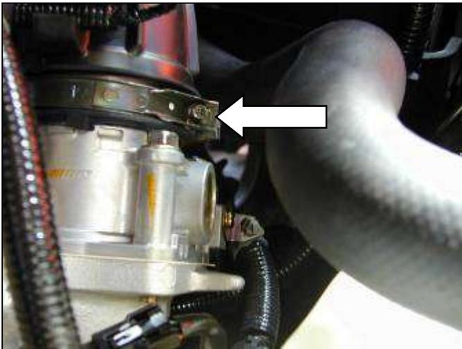
a. Loosen the hose clamp at the throttle body that secures the inlet tube.
