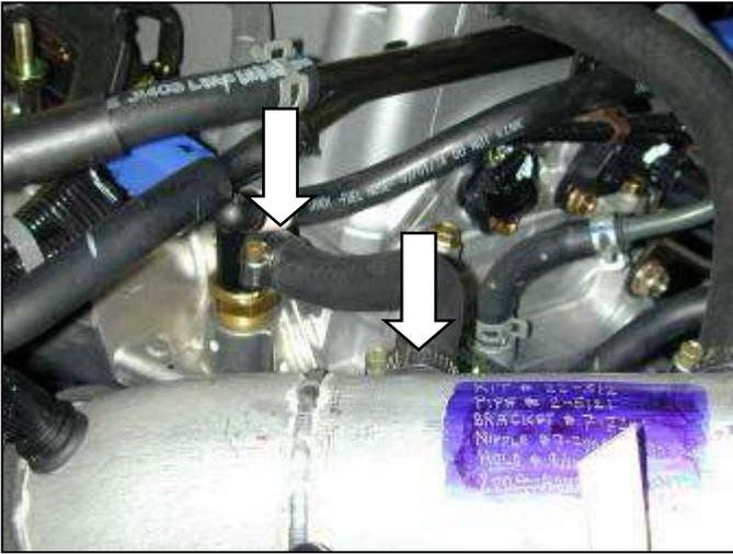
l. Attach breather hose to the crankcase and to the nipple perpendicular to the inlet pipe. Secure with hose clamps. Make sure the hose does not kink.
