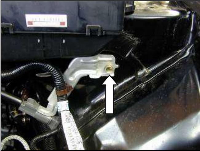
i. Remove bracket bolt. This bolt will be reused in the installation.
