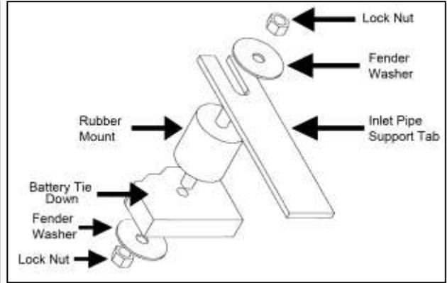
o. Secure inlet pipe to the rubber mount. Attach the air filter and secure.
