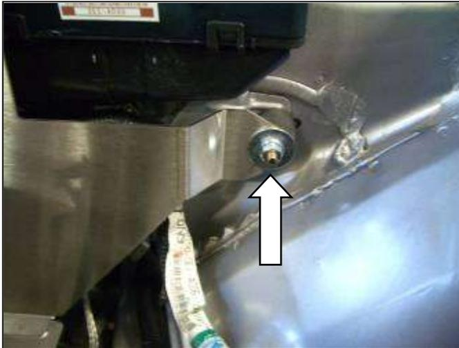
f. Insert the heat shield and attach to open rubber mount from step 3d. Attach a fender washer and nylok nut, tighten.
