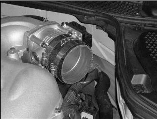
j. Install the coupler onto the throttle body. The 3" side attaches to the throttle body. Tighten the coupler to the throttle body with hose clamp no. 48.
