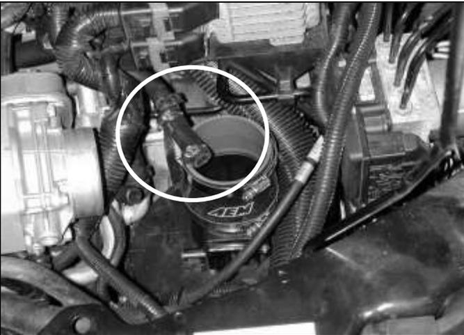
**h. Using the supplied 1/2" hose, attach the hose to the stock plastic barb fitting. Secure using the supplied 3/4" hose clamps.**
