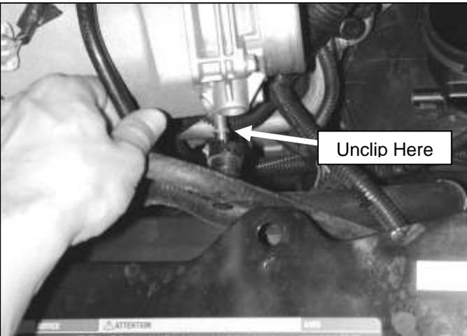
i. Unclip the idle air hose from the throttle body. Remove the four bolts securing the throttle body to the intake manifold.
