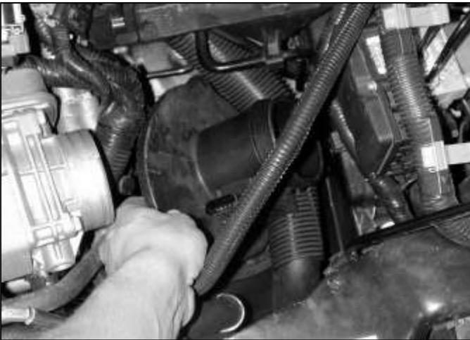
g. Remove the three screws securing the stock air box lid. Lift up on the lid and rotate it in order to separate the lid from the stock air filter.
