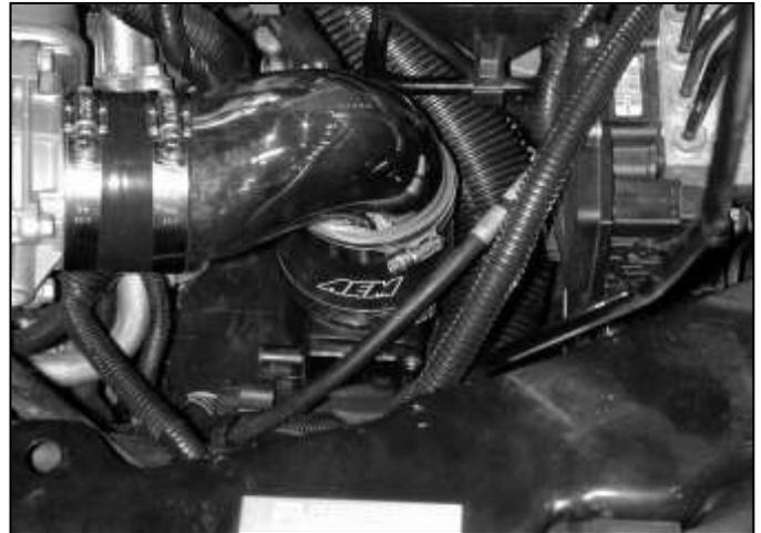
**i. Install the supplied 3" straight coupler onto the intake pipe end opposite the nipple. Place the nipple side of the intake pipe into the reducer coupler installed in step 3g. Rotate the pipe around to align the 3" coupler with the throttle body. Slide the coupler over the throttle body and secure using the three remaining #48 hose clamps.**
