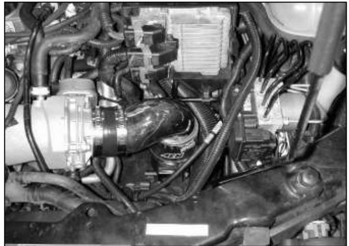
AEM<sup>®</sup> intake system installed
