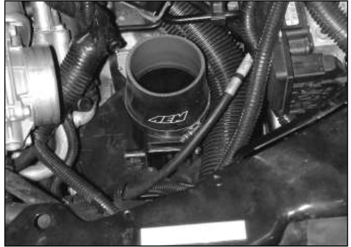
**g. Reinstall the three screws to secure the air box lid. Install the reducing couple onto the air box outlet tube. Secure the coupler using a #52 hose clamp as shown.**
