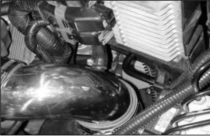
j. Install the 1/2" hose onto the AEM<sup>®</sup> intake pipe nipple and secure with the 3/4" hose clamp.
