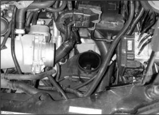
e. Loosen the hose clamps on the throttle body and the stock air filter housing. Remove the air inlet tube.
