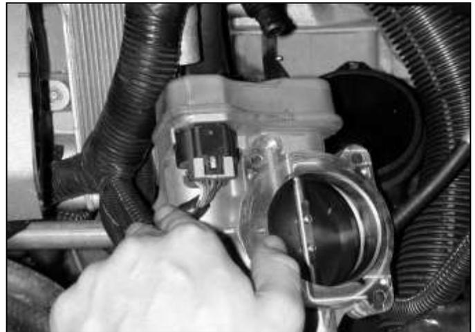
j. Unplug the throttle body wiring harness from the bottom side of the throttle body.
