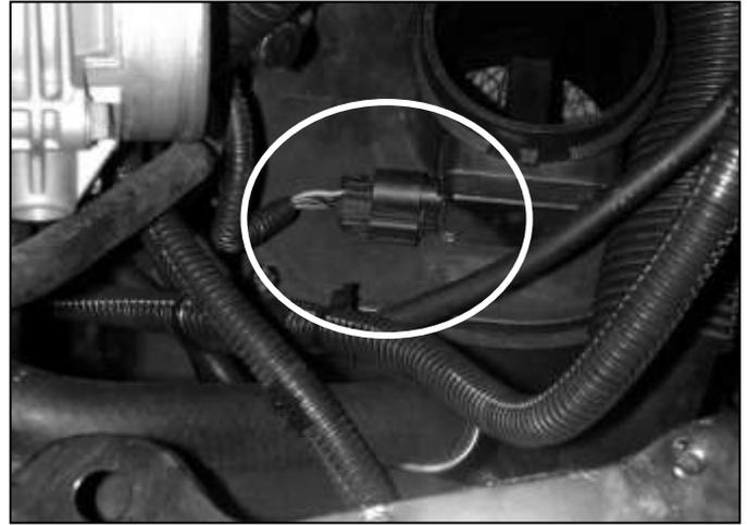
f. Unclip the Mass Air Flow (MAF) sensor wiring harness from the sensor.
