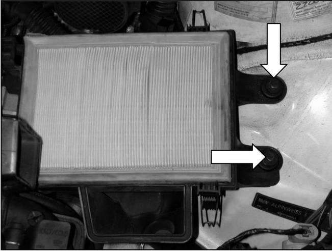
e. Loosen and remove the 2 bolts holding the bottom of the air box. Remove the air filter element and the lower half of the air box.
