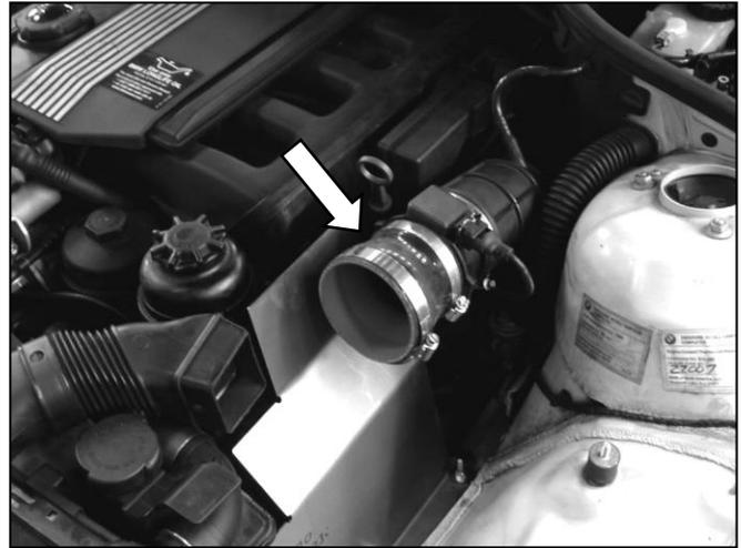
e. Attach the coupler and hose clamps to the MAF sensor as shown.
