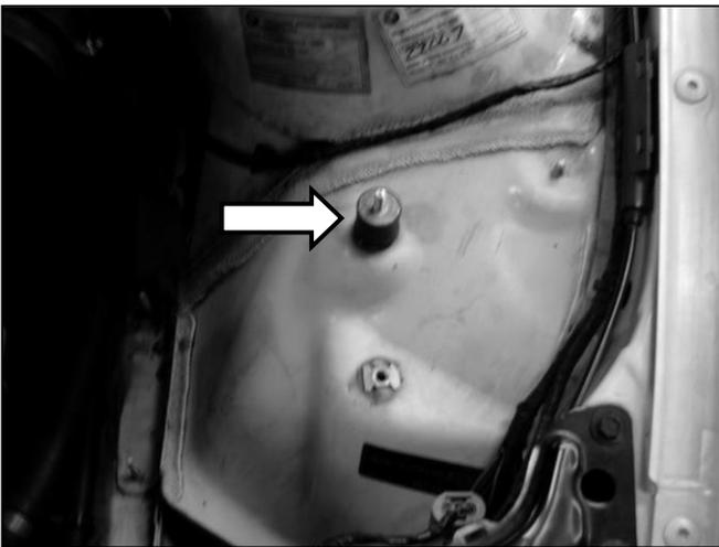
b. Insert the rubber mount as shown.
