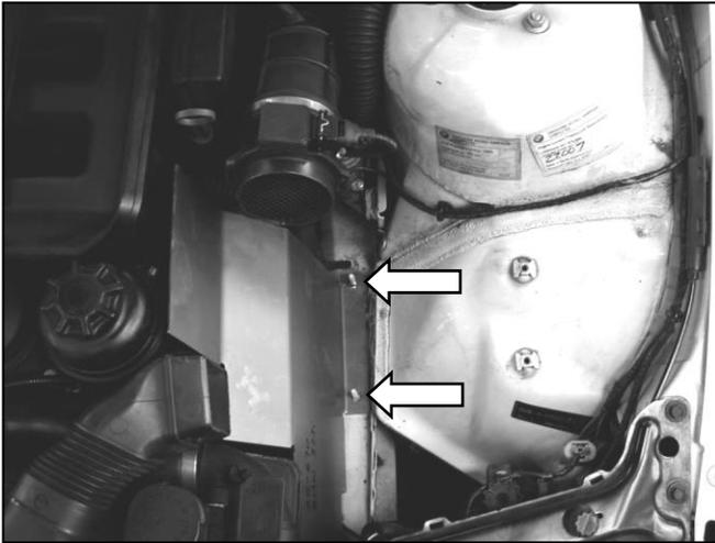
d. Insert the heat shield. Secure with washers and nylock nuts.
