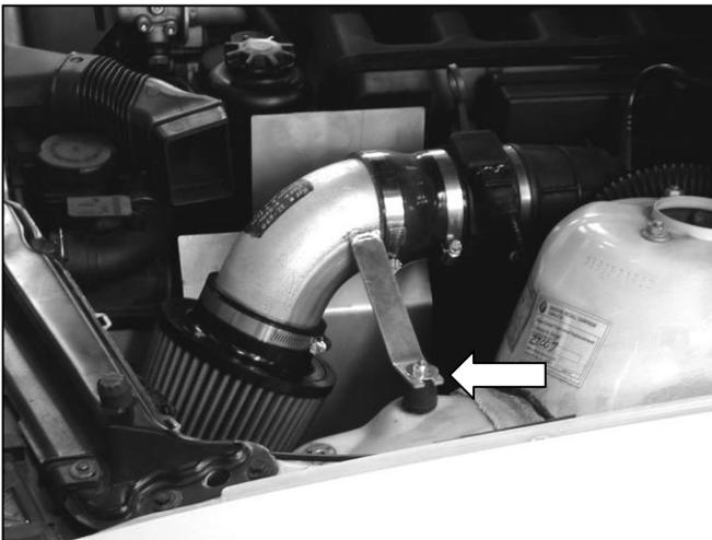
f. Attach the air filter to the inlet pipe. Then attach the assembly to the coupler that was installed on the MAF sensor in step 3e. Align the intake bracket with the rubber mount stud and secure with a washer and nylock nut. Refer to the diagram for proper installation. Ensure the air filter and intake pipe have adequate clearance. Once proper fitment is achieved secure all hardware.
