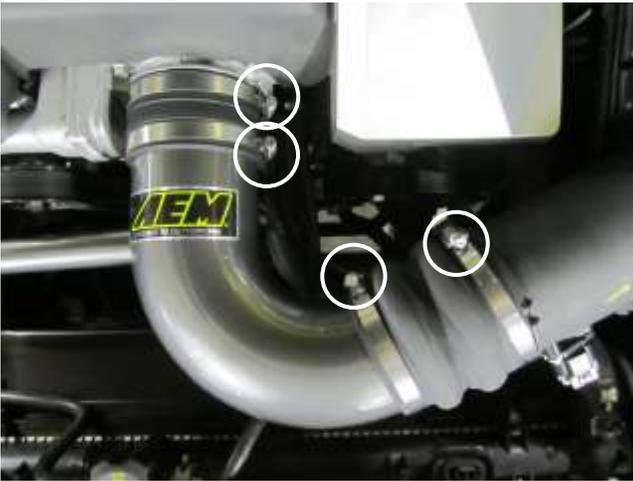
g. After proper intake tube orientation has been achieved, tighten all four hose clamps.
