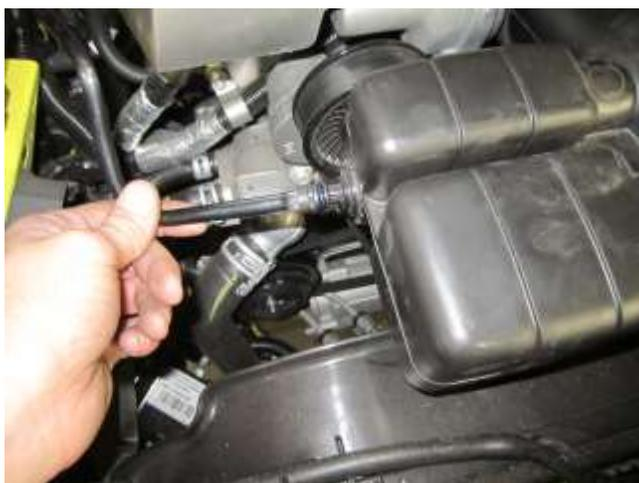
a. Disconnect the plastic breather pipe from the side of the factory intake resonator.
