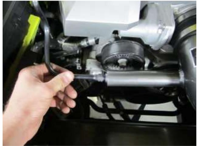
h. Install the plastic breather pipe that was disconnected in 2a. into the AEM intake.
