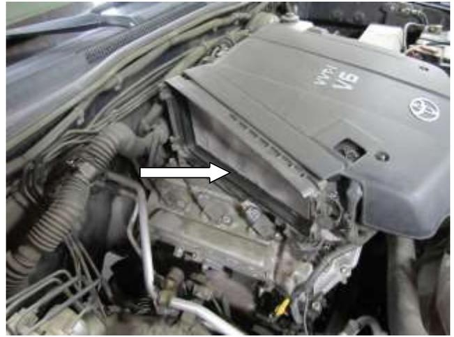
f. The hydrocarbon trap filter will remain in the air box; do not attempt to remove it. The hydrocarbon trap filter is an emission control device and should not be removed to retain legal status in California
