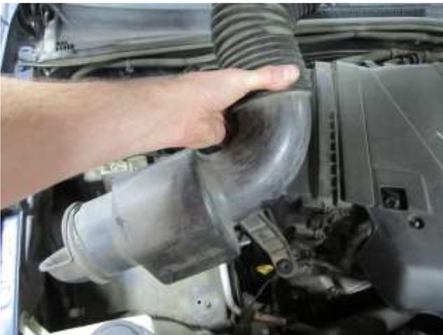
c. Pull the intake tube out of the fender and remove from the vehicle. **NOTE:** Do not discard your factory intake components.
