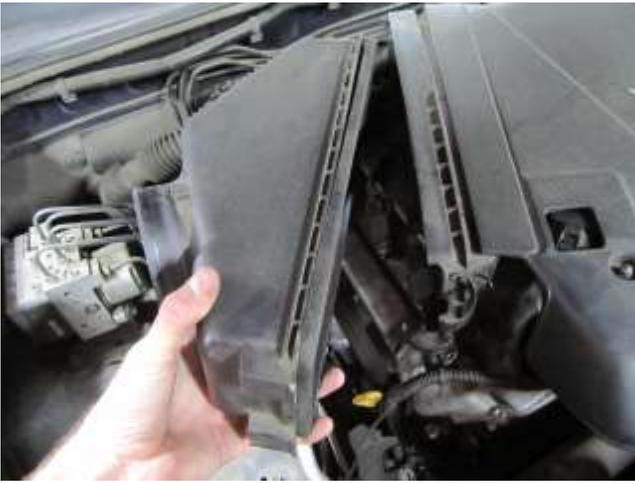
e. Remove the stock air box lid and the filter.
