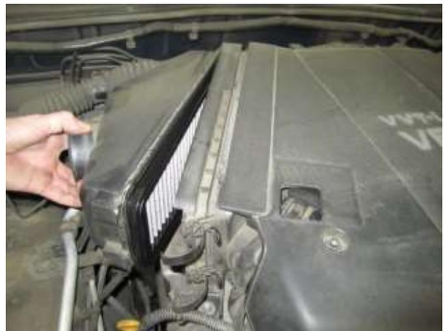
b. Re-install the AEM filter and air box lid to the air box base. Make sure that the back of the lid is correctly hinged.
