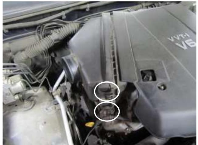
d. Unclip the two stock air box clamps.
