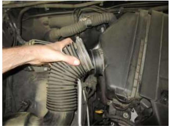
b. Detach the intake tube from the air box.
