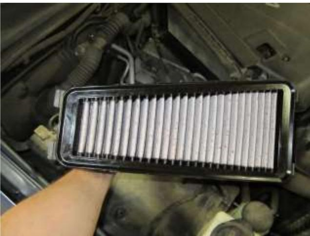
a. Install the AEM filter into the air box lid.
