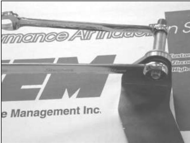
c. Install the factory mounting stud from step 3b on the supplied engine mount bracket, using the nylock nut and washer provided.
