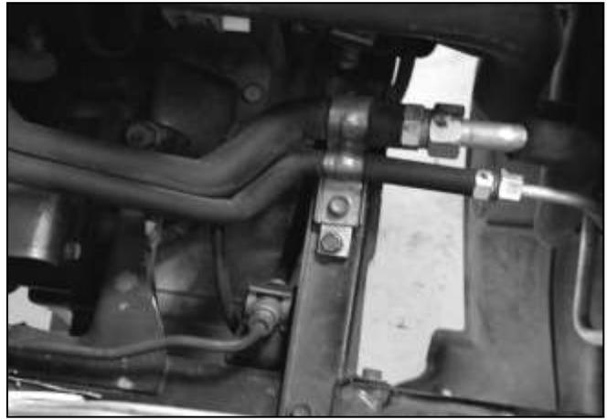
h. Reinstall the A/C line bracket to the spacer. Do not over tighten or threads will be stripped from the spacer.
