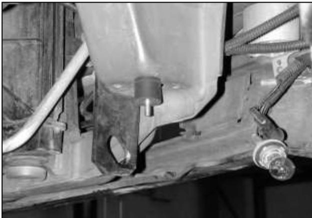
b. Install the rubber mount in the hole on the underside of the frame next to the frame hook as shown in the picture.
