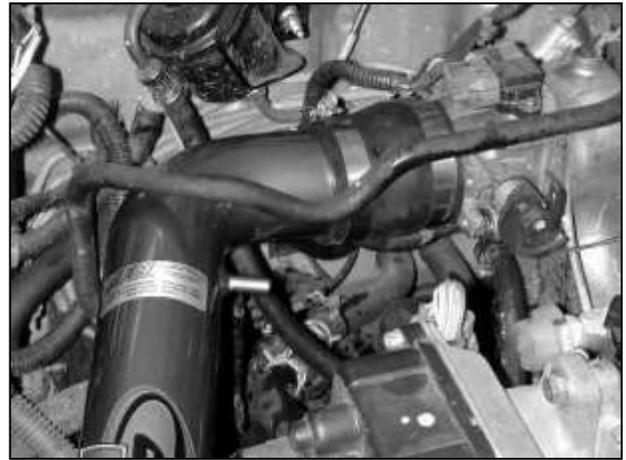
g. Install the 3/8" hose from the valve cover vent to the nipple on the intake pipe. Secure it in place with 3/4" hose clamps.
