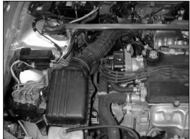
b. Remove the stock air box system by loosening the hose clamp around the throttle body and removing the two air box mounting bolts.
