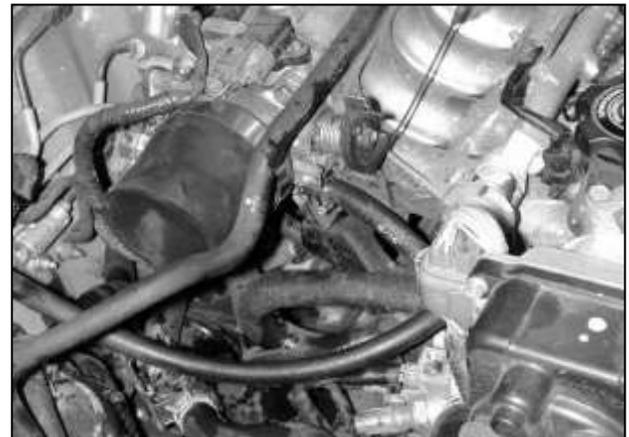
c. Insert the 2.5" x 3.0" coupler onto the throttle body (this is a tight fit). Slide the two #44 hose clamps over the end of the coupler.
