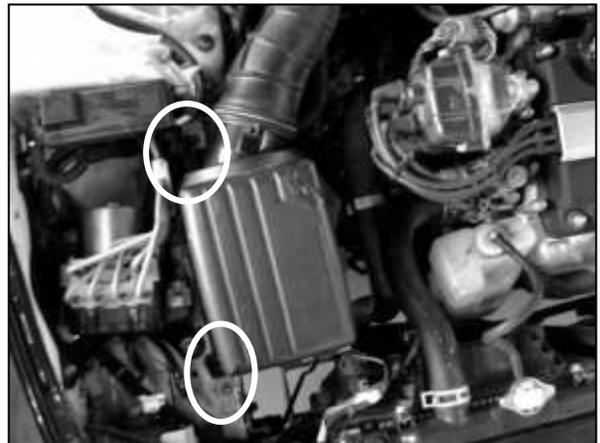
b. Remove the stock air box and intake system by loosening the hose clamp around the throttle body and removing the two airbox mounting bolts.
