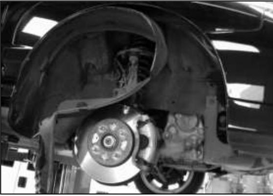
c. Remove the passenger side wheel. Partially remove the splash guard and tuck it out of the way.
