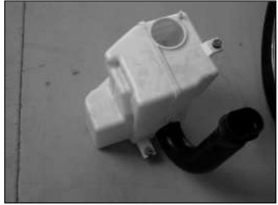
d. Remove the resonator from the cavity behind the front bumper.
