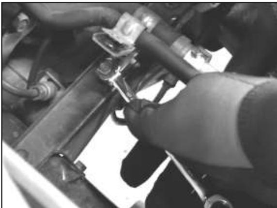
i. Using the M6 x 15mm bolt from the AEM® kit, bolt the spacer to the bracket.
