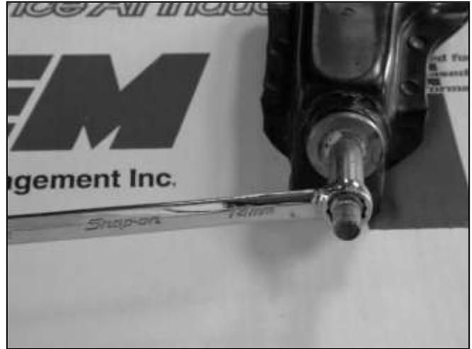
b. Using a 14 mm wrench, remove the mounting stud from the factory engine mount assembly. It may be necessary hold the bracket in a vice to do this.
