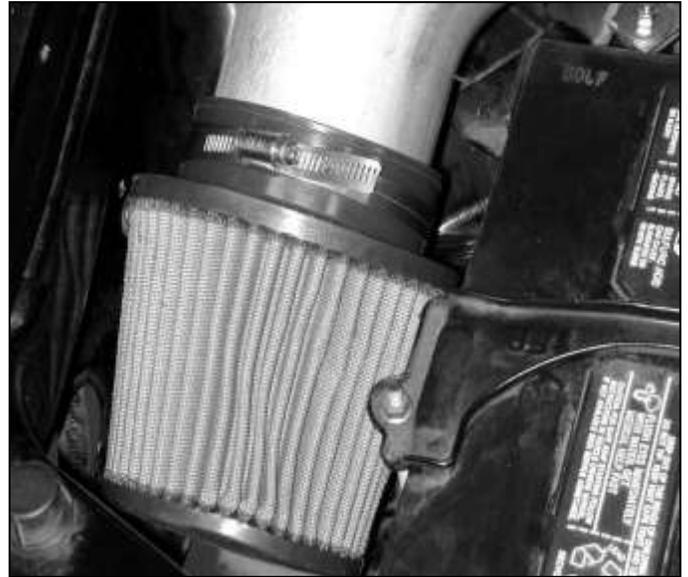
g. Slide the inlet pipe support over the rubber mount. Use the supplied washer and lock nut and assemble as shown. Do not tighten until the intake is properly fitted and is not touching anything in the engine bay. Next install the AEM® air filter onto the end of the inlet tube. Push the filter over the inlet pipe until it mates to the step inside the filter inlet. Install the supplied #64 hose clamp to secure the filter onto the inlet pipe. Tighten the hose clamp after this is done.
