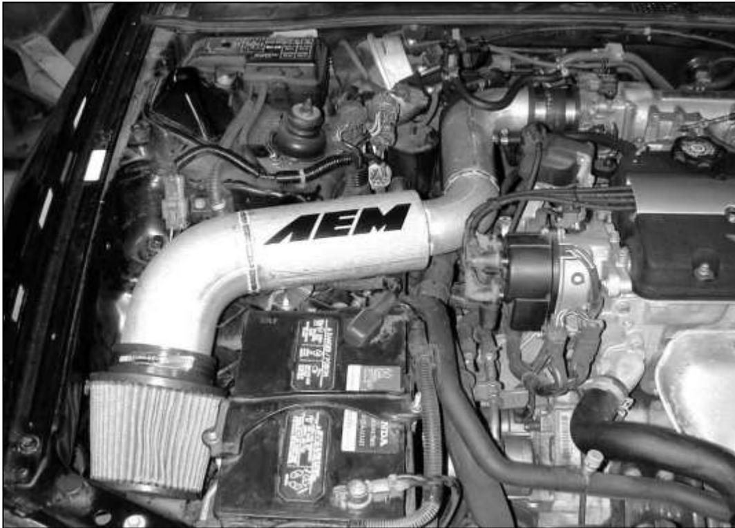
h. Check that the filter is not touching any part of the vehicle. Position the inlet pipe for best fitment. Be sure that the pipe or any other component is not in contact with any part of the vehicle. Tighten the hose clamps at the throttle body. Tighten the nut on the rubber mount. Check for proper hood clearance. Re-adjust pipe if necessary.
