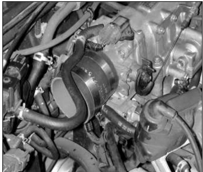
c. Install the 2.75" hose on to the throttle body using both #44 hose clamps. Check to see that the inside of the AEM® inlet pipe and air filter are clean and free from any foreign objects and/or obstructions.
