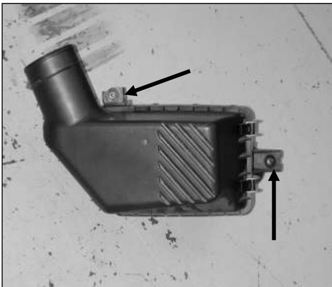
d. Unbolt the two bolts holding the air filter housing to the chassis. Lift and remove the air filter housing.
