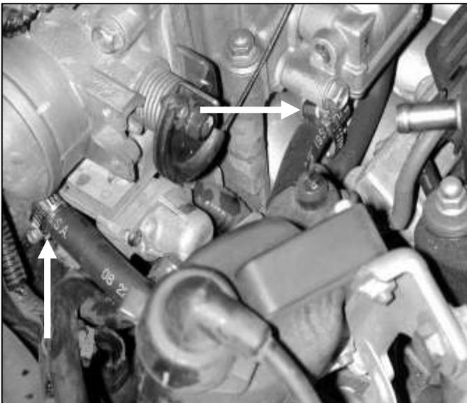
b. Connect the new supplied water bypass hose and  $\frac{3}{4}$ " hose clamps to the throttle body and the intake manifold where the factory water bypass hose was disconnected earlier.
