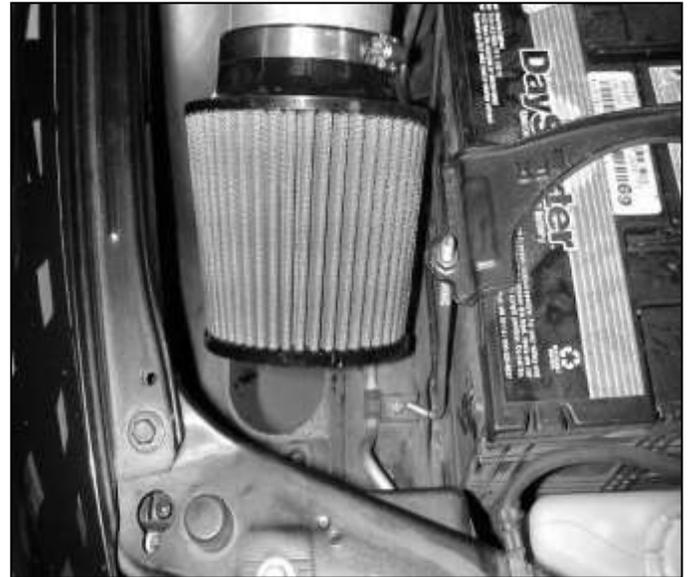
h. Remove the original 5/32" breather line that was between the stock intake pipe and the hard plastic breather line. Install the supplied longer 5/32" vacuum hose and attach it to the nipple on the backside of the intake pipe.
