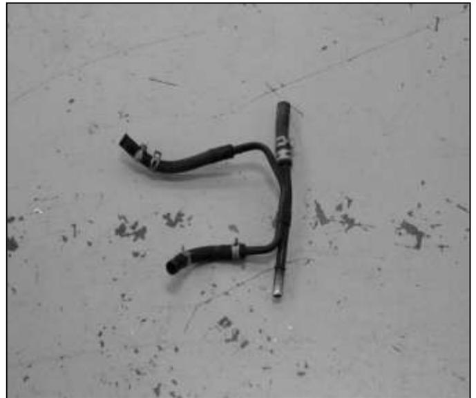
b. Disconnect the breather tube from the OE air inlet tube. On 92-96 models, remove the small breather tube from the top of the OE air inlet tube. The tube is inserted into a rubber boss on the inlet tube. Loosen the hose clamp holding the air inlet tube to the throttle body. Remove the air inlet tube by sliding it off the throttle body and pulling it off the air filter housing.
