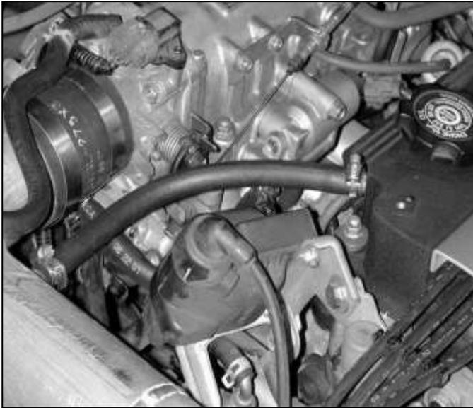
f. Install the supplied 3/8" breather hose from the nipple on the intake pipe to the nipple on the valve cover. Use the supplied 3/4" hose clamps on the AEM® intake pipe nipple and on the valve cover nipple. Install the small rubber vacuum line plug on the manifold where the vacuum line from the IAC solenoid valve was removed.
