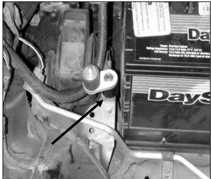
d. The intake mount assembly consists of; (1) aluminum spacer, (1) mount re-locator, (1) rubber soft mount, (1) M6 x 40 bolt, (1) washer, and (1) nylok nut. These should be assembled as shown above.
