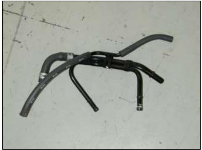
c. **CAUTION: Ensure the engine is completely cool before removing the coolant hose, or hot coolant will escape from the cooling system and cause injury or damage. Be sure to capture any lost coolant in a clean container.**
