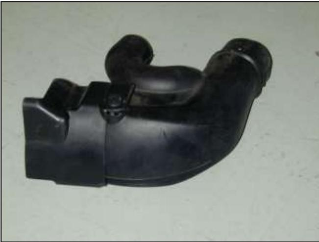
f. Remove the intake air duct in front of the air filter housing by simply pulling up on it.
