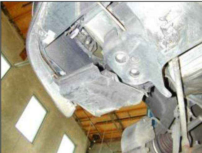
d. Raise the front of the vehicle with a jack. Refer to your owner's manual for proper jack and jack stand placement to properly support vehicle. Support your vehicle using properly rated jack stands before wheel removal or while working under the vehicle. **NEVER WORK UNDER A VEHICLE WITHOUT USING JACK STANDS.** Remove the front passenger side wheel. Unbolt the plastic shield from the inner fender and front bumper.
