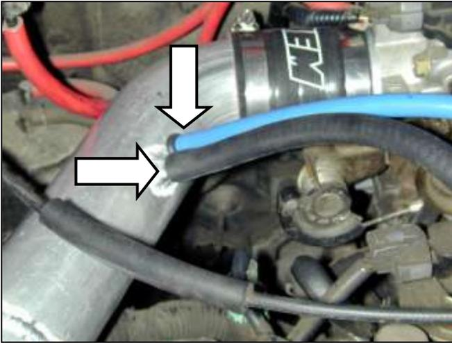
f. Install the supplied grommet into the vacuum line hole in the AEM® intake pipe for 94-95 VTEC equipped models. Insert the plastic connector into the vacuum hose then insert the other end of the plastic connector into the grommet. Install the supplied 5/8" breather hose from the nipple on the intake pipe to the nipple on the valve cover. Use the supplied 1" hose clamps on the AEM® intake pipe nipple and on the valve cover nipple. These hoses were removed in step 2b.
