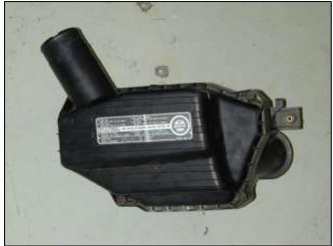
g. Unscrew the two bolts securing the air filter housing and pull the housing out of the car.
