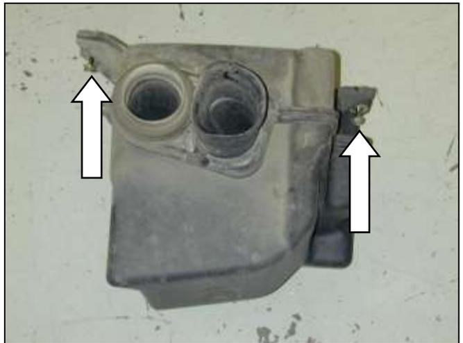
e. Unbolt the two bolts holding the air resonator box in place and lower it out of the bottom of the vehicle.
