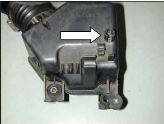
h. Unplug the two breather hoses that attached the tube connecting the air filter housing to the throttle body. Loosen the hose clamp on the throttle body and slide the tube out and up. Be sure to disconnect the vacuum lines connected to the air chamber under the main tube.
