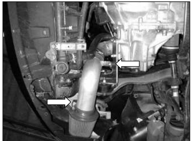
e. Install the lower intake pipe using the included coupler and hose clamps. Secure the bracket to the rubber mount using the supplied nylock nut and washer, as shown. Install the air filter and secure it with the supplied clamp.
