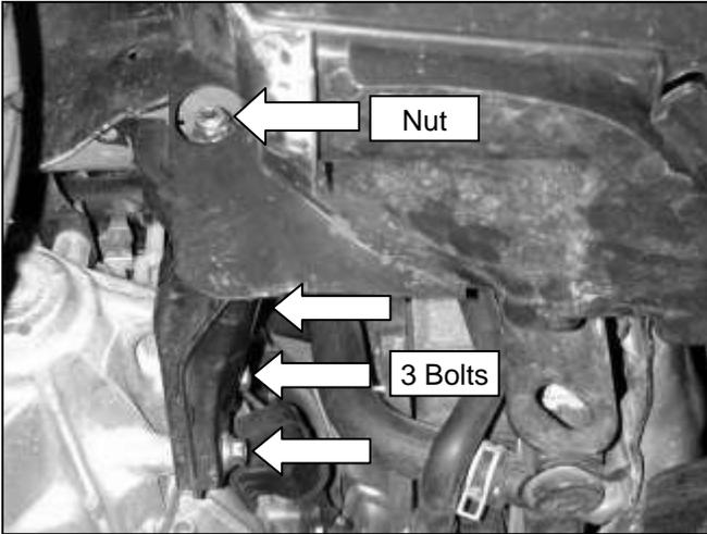
a. Remove the engine mount nut, then loosen the three bolts, and remove the mount.
