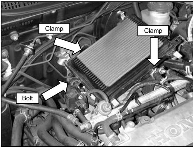
c. Loosen the bolt, breather clamp and the hose clamp securing the air filter assembly to the throttle body and remove it.
