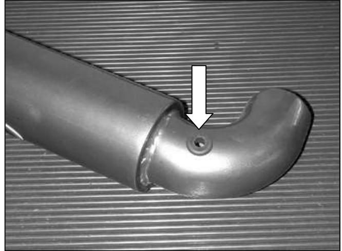
c. Install the rubber grommet in the 5/8" hole in the upper intake pipe.
