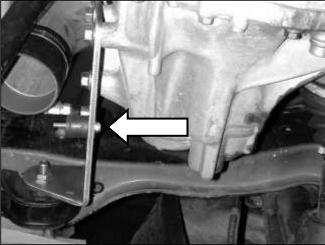
b. Install the supplied rubber mount using the included nylock nut and washer.
