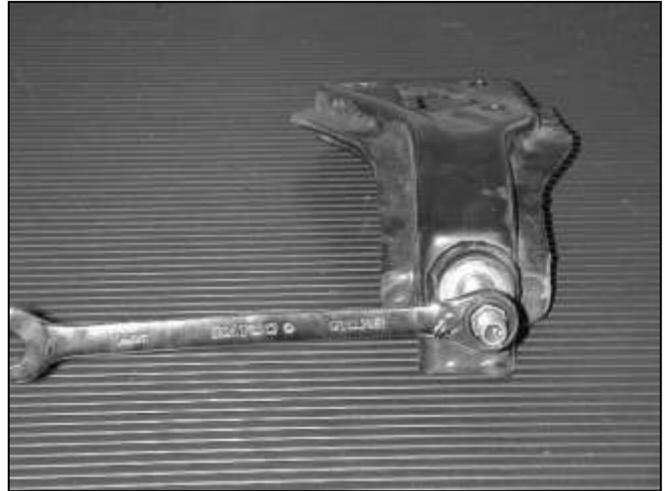
b. Using a 14mm wrench, remove the mounting stud from the factory engine mount assembly.
