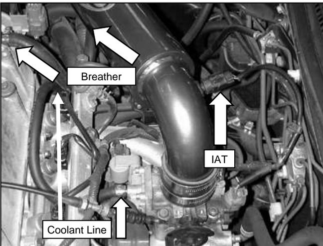
d. Using the supplied coupler and clamps, install the upper intake pipe. Install the intake air temp sensor, and the cam cover breather line onto the nipple, and secure it with the included clamp. Install the coolant line, and secure it with the included clamps.
