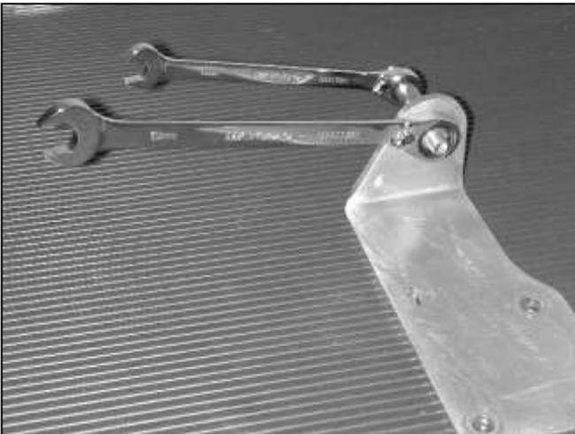
c. Install the factory mounting stud from step b on the supplied engine mount bracket, using the supplied Nylock nut and washer.
