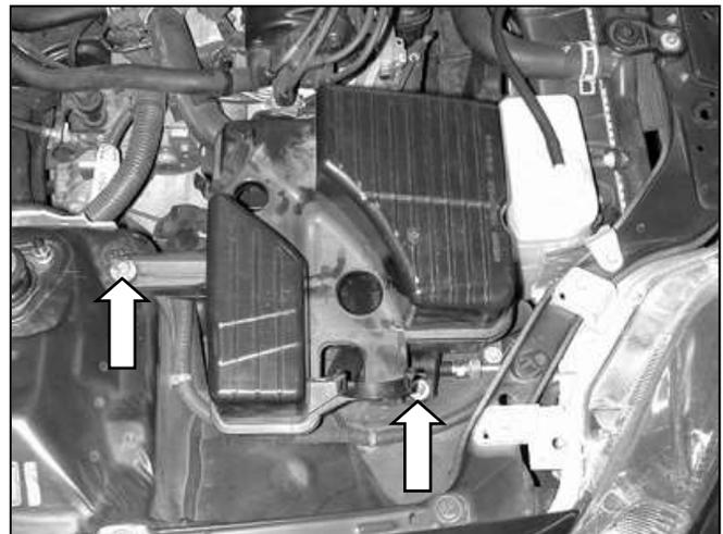
b. Loosen the bolts holding the resonator box to the frame rail, and remove it.
