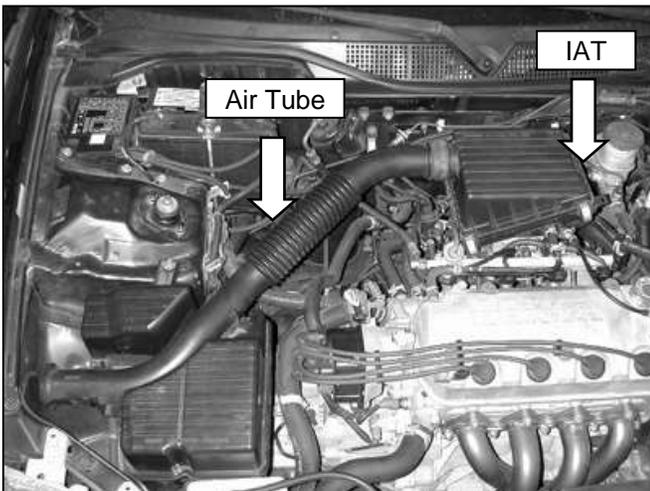
a. Remove the intake air temp sensor (IAT) from the air filter lid, then remove the air tube and filter lid from the vehicle.
