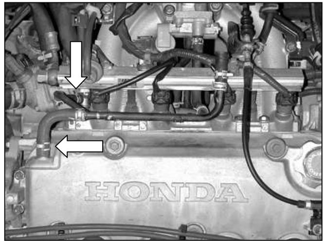
d. Remove the clamps as shown, and remove the metal breather pipe assembly.
