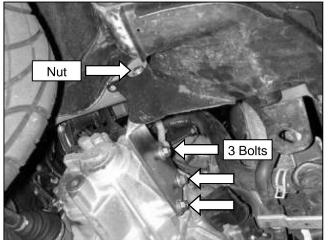
d. Using the supplied bolts and the factory washers, install the AEM<sup>®</sup> engine mount on the transmission, torque bolts to 61 ft-lb. Then replace the factory washer and nut on the mounting stud.
