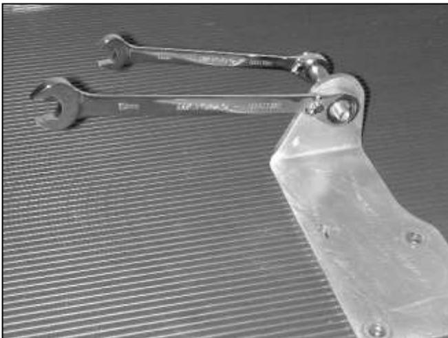
c. Install the factory mounting stud from step 3b on the supplied engine mount bracket, using the supplied nylock nut and washer.
