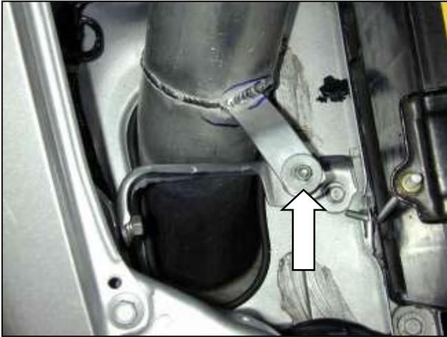
h. Install the washer and then the nylok nut on top of the intake bracket. Do not tighten the nut all the way down.
