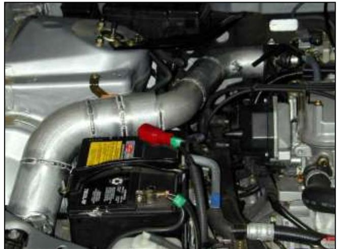
k. Position the intake system for best fitment. Be sure that the pipe or any other component is not in contact with any part of the vehicle. Tighten the hose clamps at the throttle body and silicone coupler. Tighten the nut on the mounting bracket. Re-adjust the intake pipe if necessary.
