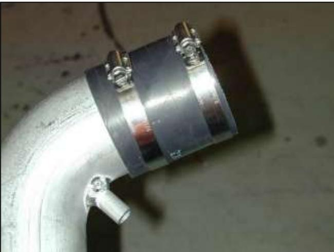
b. Ensure the inside of the AEM intake pipe and air filter are clean and free from any foreign objects and/or obstructions. Install the 2.50"-2.75" reinforced reducer over the throttle body end of the intake pipe using the 2.5" and 2.75" hose clamps as shown.
