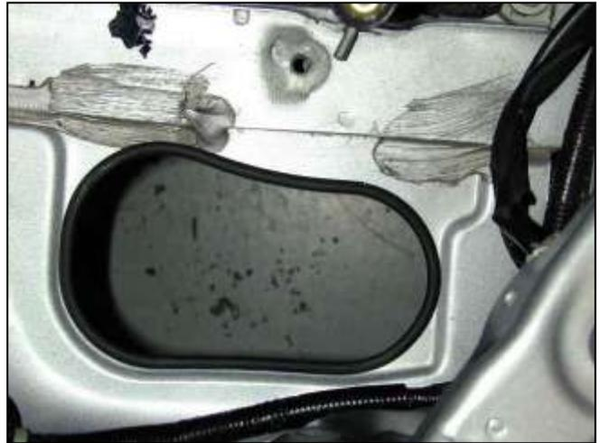
c. Install the rubber edge trim around the edge of the hole that passes through the engine bay.
