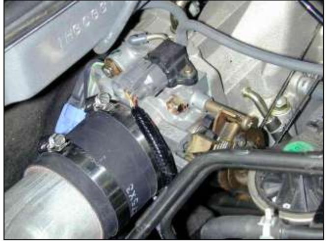
e. Place the reducer coupler over the throttle body but do not tighten the hose clamp completely.
