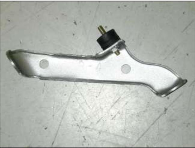
f. Using the previously removed stock air-filter housing bracket, thread the supplied rubber mount in the hole where the air-filter housing was bolted.
