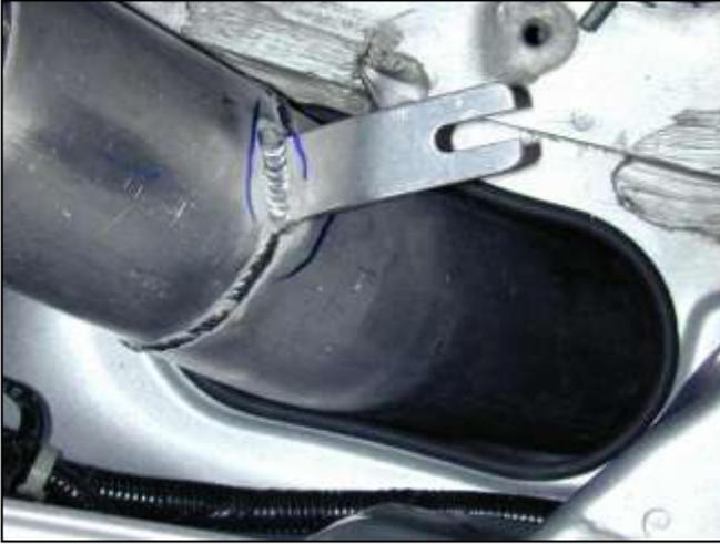
d. Slide the large diameter end of the AEM® intake pipe through the hole in the engine bay. Then slip the smaller end under the strut tower brace. Be sure to use rags to prevent the intake pipe from getting scratched.
