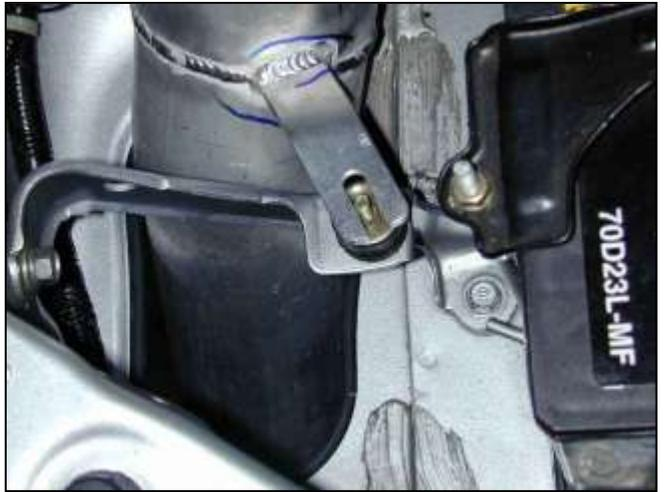
g. Install the air filter housing bracket in its original location with the rubber mount attached.
