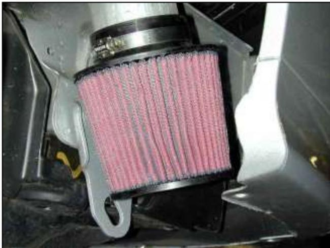
j. Install the AEM® air filter on to the end of the inlet tube. Push the air filter over the inlet pipe up to the stop in the filter. Install one hose clamp to secure the filter onto the inlet pipe. Once proper fitment is achieved, tighten the hose clamp.
