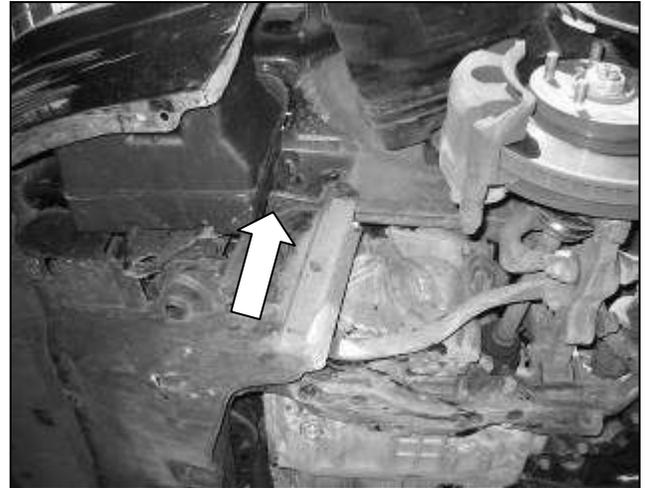
d. Remove the plastic clips holding the lower splash shield and fender liner on. Remove the two bolts holding the intake resonator in place, then lower the resonator out from the bottom of the vehicle.
