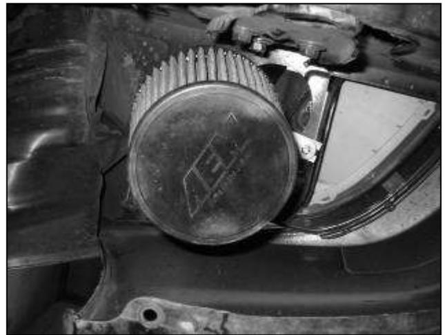
g. Install the AEM<sup>®</sup> air filter onto the end of the intake pipe. Push the air filter onto the intake pipe until the stop in the air filter is reached. Once proper fitment and clearance is achieved, secure the air filter to the intake pipe with the supplied hose clamp.
