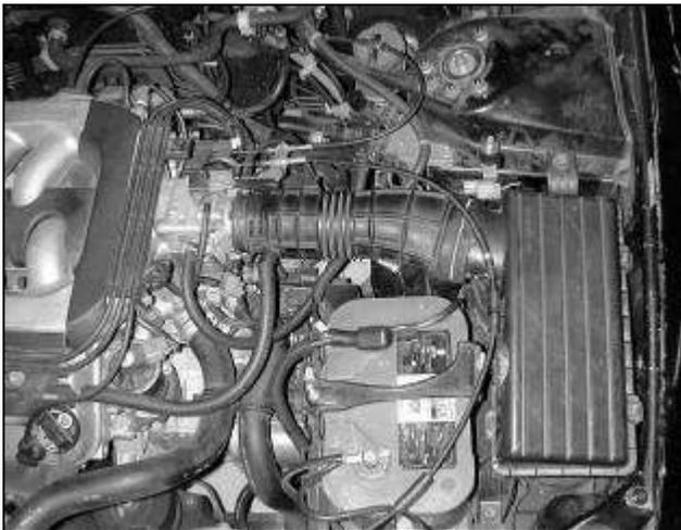
a. Factory airbox system installed.
