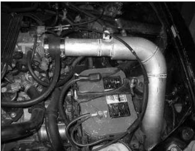
AEM<sup>®</sup> intake system installed
