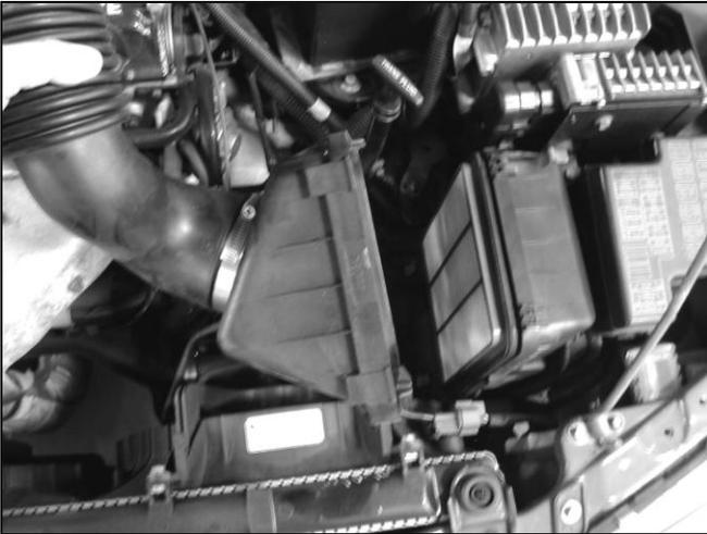
c. Unclip the air filter box and remove the intake tube from the engine bay. Remove the air filter.
