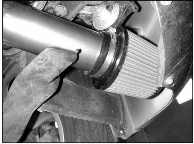
k. Install the air filter on the end of the intake pipe. Ensure the splash guard is properly installed and allows clearance for the intake pipe.
