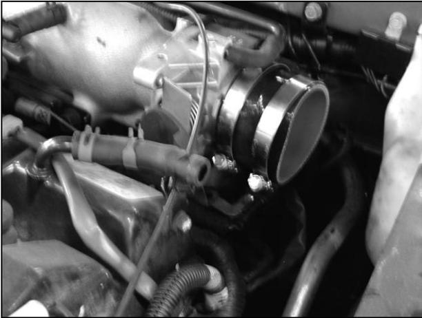
d. Install the silicone coupler on the throttle body. Place the hose clamps in place but do not tighten them.
