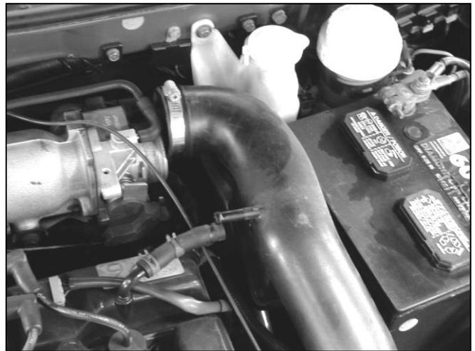
b. Disconnect the intake tube from the throttle body.
