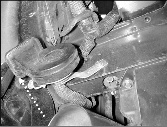
j. Rotate the horn bracket forward out of the way of the intake pipe.
