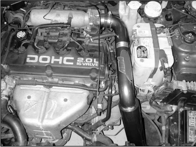
h. Position the intake pipe in the engine bay so that no part of it touches the vehicle.
