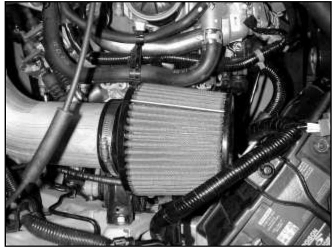
g. Install the AEM® filter on to the end of the inlet tube. Push the air filter over the inlet pipe until the "stop" in the air filter is reached. Install one hose clamp to secure the filter onto the inlet pipe. Once fitment is checked, you can either push the filter onto the inlet pipe more or less depending on clearances. Tighten the hose clamp after this is done.
