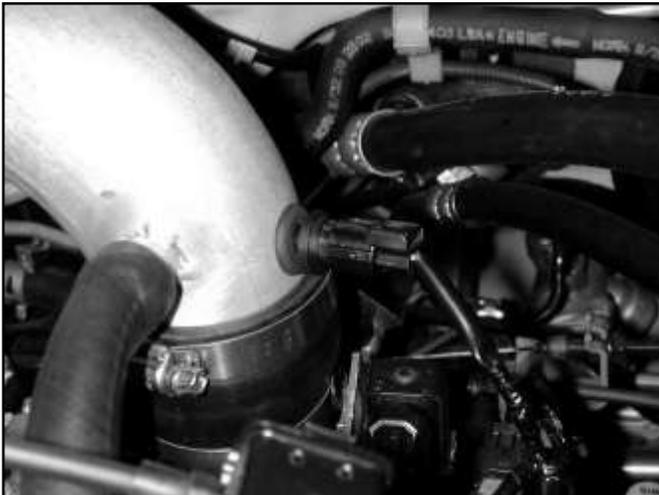
f. Install the supplied grommet into the IAT sensor hole in the AEM® intake pipe. Install the IAT sensor into the grommet and plug in the IAT sensor connector. Install the supplied 5/8" breather hose from the nipple on the intake pipe to the nipple on the valve cover. Use the supplied 1" hose clamp on the AEM® intake pipe nipple and the original hose clamp on the valve cover nipple.
