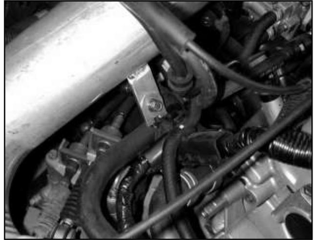
e. Thread supplied washer and bolt through the inlet pipe mounting tab into the factory intake resonator mounting bracket. Do not tighten.
