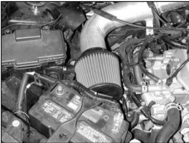
h. Ensure that the air filter is not touching any part of the vehicle. Position the inlet pipe for best fitment. Be sure that the pipe or any other component is not in contact with any part of the vehicle. Tighten the hose clamps at the throttle body and reducer coupling. Tighten the bolt on the intake resonator mounting bracket. Check for proper hood clearance. Re-adjust pipes if necessary.
