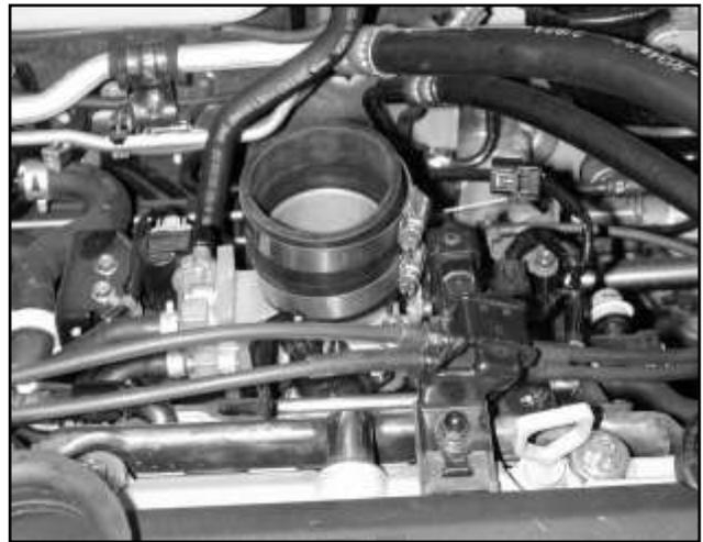
c. Install the 2.5" - 2.75" hose on to the throttle body using the 2.5" and 2.75" hose clamps. Check to see that the inside of the AEM® inlet pipe and air filter are clean and free from any foreign objects and/or obstructions.
