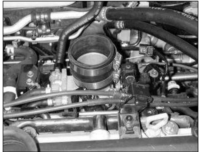
c. Install the 2.5" - 2.75" hose on to the throttle body using the 2.5" and hose clamps. Check to see that the inside of the AEM® inlet pipe and air filter are clean and free from any foreign objects and/or obstructions.
