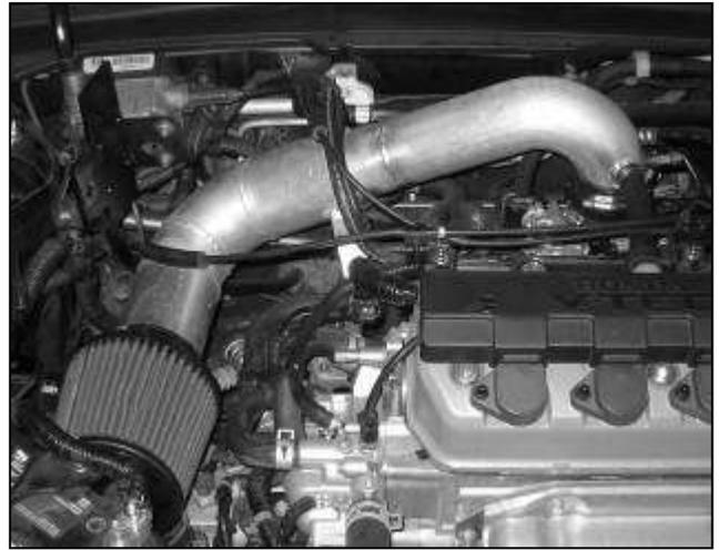
h. Check that the air filter is not touching any part of the vehicle. Position the inlet pipe for best fitment. Be sure that the intake pipe or any other component is not in contact with any part of the vehicle. Tighten the hose clamps at the throttle body and reducer coupling. Tighten the bolt on the intake resonator mounting bracket. Check for proper hood clearance. Re-adjust pipes if necessary.
