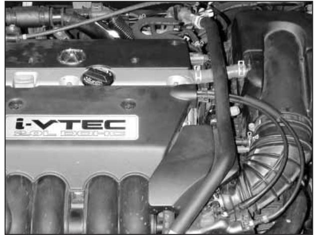
b. Make note there is one breather hose, one vacuum hose, and one intake air temperature (IAT) sensor.
