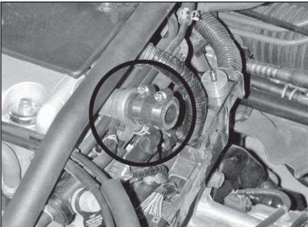
d. Replace the factory breather hose with the supplied breather hose. Use the supplied 1 1/4" hose clamps to secure the breather hose in place.
