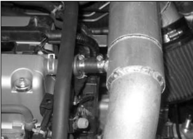
h. Slide the supplied breather hose onto the AEM® intake pipe and use the 1-1/16" hose clamps to secure. This hose should be trimmed to fit properly.
