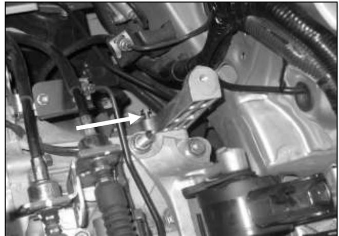
l. Remove the three bolts holding the stock air intake bracket to the transmission.
