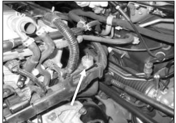
e. Install the aluminum spacer onto the mounting stud where the stock intake mounted.
