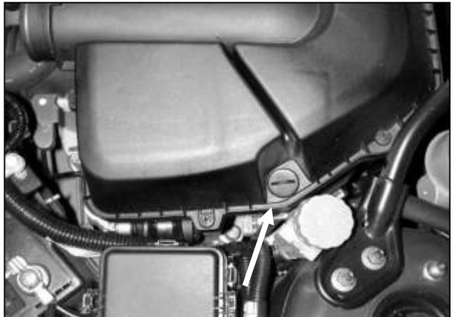
h. Remove the rubber plug from the filter box. Then remove the bolt under the plug.
