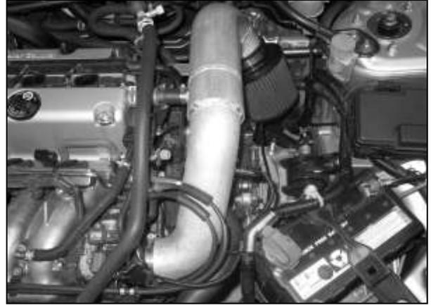
k. Check that the filter is not touching any part of the vehicle. Position the inlet pipe for best fitment. Be sure that the pipe or any other component is not in contact with any part of the vehicle. Tighten the hose clamps at the throttle body and silicone coupling. Tighten the nut on the mounting bracket.
