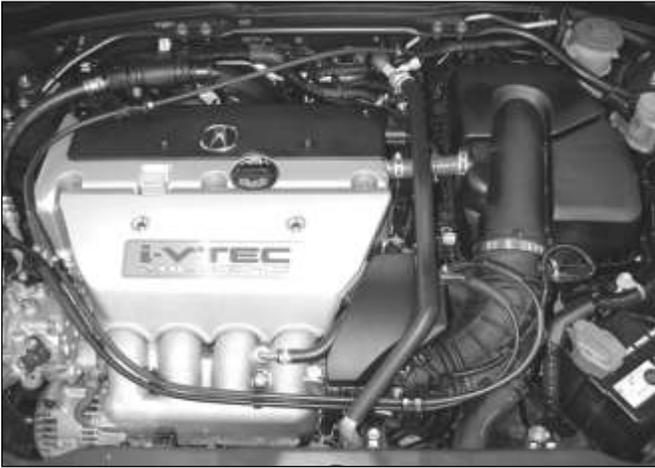
a. Factory air box configuration. Make note that there is one breather hose, one vacuum hose, and one Intake air temperature (IAT) sensor.
