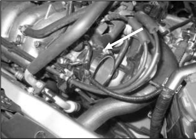
b. Install the 3" hose on to the throttle body using the #48 hose clamps. Check to see that the inside of the AEM® intake pipe and air filter are clean and free from any foreign objects and/or obstructions.
