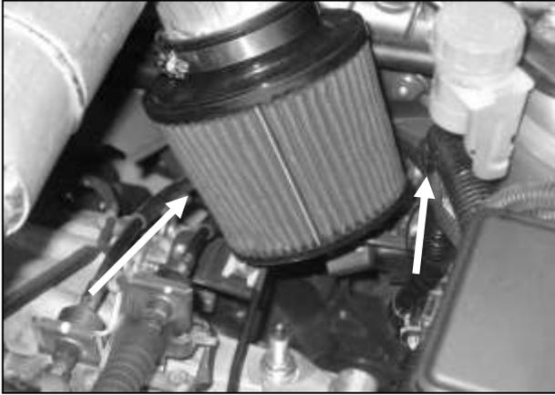
j. Install the AEM<sup>®</sup> air filter onto the end of the inlet tube. Push the air filter over the inlet pipe until the stop in the filter is reached. Then install the #56 hose clamp to secure the filter onto the inlet pipe. Once proper fitment is confirmed, tighten the hose clamp.
