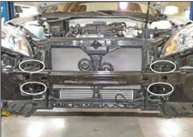
u. Remove the bumper support by removing 6 M8 bolts, and 2 M6 nuts.
