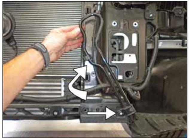
x. Rotate the power steering cooler as shown and retighten the M6 bolt to hold it in place temporarily.
