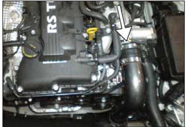
ag. Install one of the straight couplers onto the throttle body using 2 #44 clamps and install the left charge pipe as shown. Secure it to the rubber mount using the supplied fender washer and M6 nut. Plug in the boost sensor.
