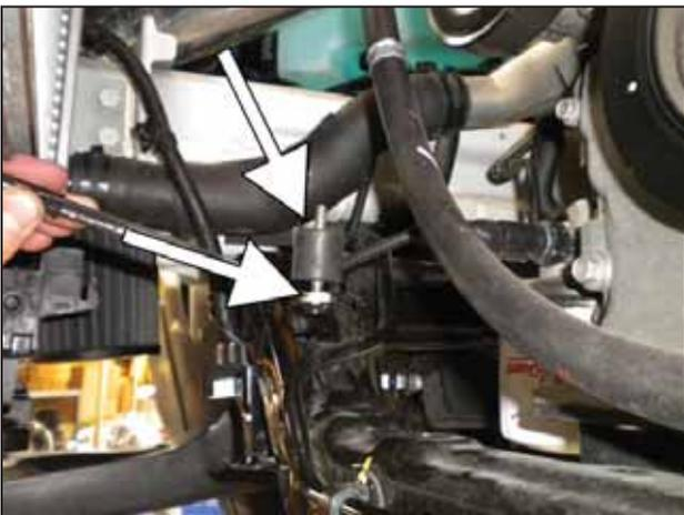
j. Install the other M6 rubber mount as shown with the small aluminum spacer under it. Hand tighten the rubber mount.
