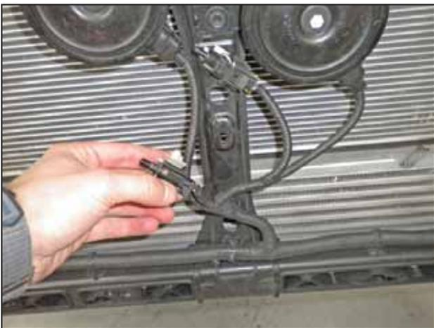
y. Unclip the ambient air temp sensor from the vertical support.
