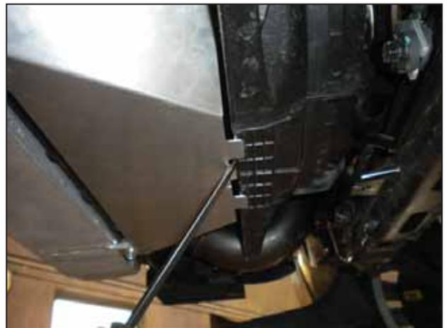
am. From under the car, manipulate the fan shroud and intercooler shroud so that the tabs snap into position.
