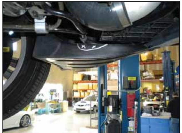
as. Check for clearance of the power steering cooler lines to the fender liner. Gently bend the lines and / or trim the fender liner as needed.
