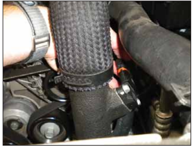
f. Unplug the boost pressure sensor located on the left charge pipe near the throttle body.
