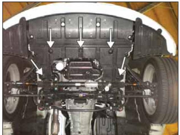
ay. Install the second under tray using the 5 M6 screws removed in step 2(o).
