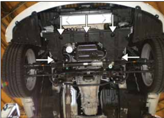
o. Remove the second under tray by removing 5 M6 bolts.
