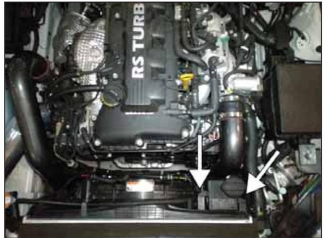
aq. Install the coolant reservoir using the two self-tapping screws removed in step 2(b). Connect the overflow hose and ensure clearance between the reservoir and left charge pipe; readjust the pipe if necessary.
