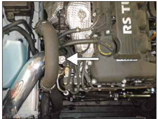
h. Remove the M8 bolt securing the right charge pipe to the bracket above the power steering pump.
