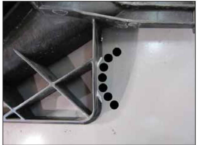
ak. After trimming, the fan shroud should look as shown.
