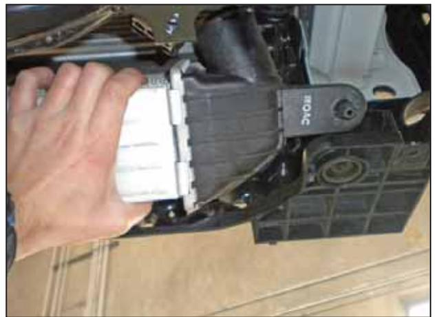
ab. Lift up on the intercooler and rotate the bottom of it out towards the rear of the car. Then lower and remove the intercooler. It may be helpful to support the radiator from the top using clamps during this step.
