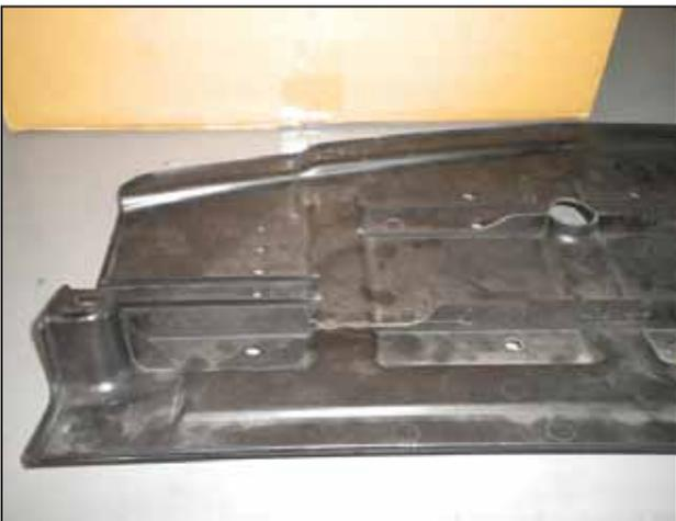
ax. Install the trimmed under tray using only the two outer mounts and two of the bolts removed in step 2(n). Check for clearance in the trimmed areas and modify if necessary.
