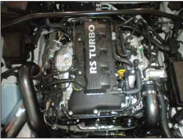
ah. Take some time to align the charge pipes for best fit. There should be about  $\frac{1}{4}$ " minimum clearance between the pipes and other components in the engine bay.
