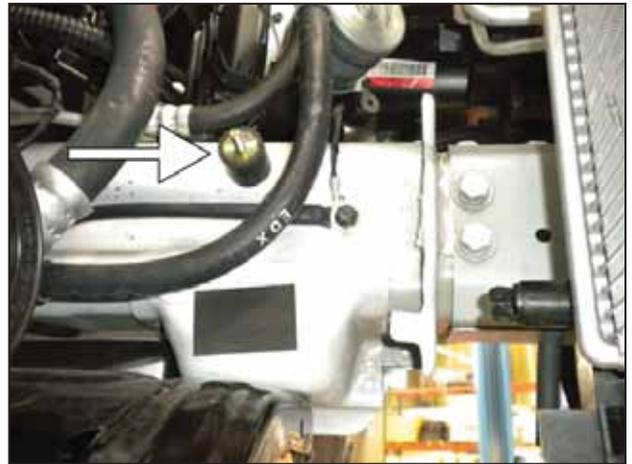
i. Install one of the supplied M6 rubber mounts into the vacant bolt hole from the previous step. Hand tighten the rubber mount.
