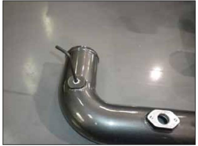
ae. If not using water injection, install the supplied 1/8" NPT plug into the water injection bung on the left charge pipe. Use some Teflon tape or thread sealant. If using an AEM® water injection system, install the injector using Teflon tape or sealant and follow the instructions provided with the water injection kit.
