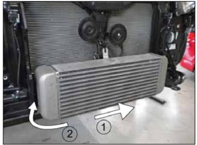
m. With the left neck in position, tip the top of the intercooler back and guide the right neck into position. The intercooler will have to be pushed all the way to the left side of the car for the right neck to slip past the opening.
