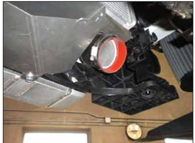
ac. Install one of the straight couplers on the intercooler as shown using 2 #44 clamps. Apply some silicone spray to the inside of the coupler to help with installation.
