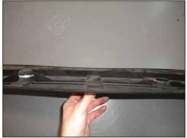
au. Two inner mounts and one reinforcement rib of the front under tray need some minor trimming.
