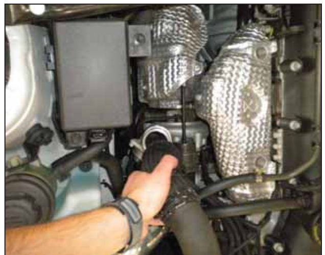
j. Pull the right charge pipe up and off of the compressor outlet.
