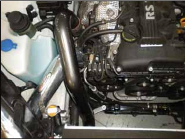
ad. Install the right charge pipe as shown. Line up the lower end of the pipe, and press the upper end down into the coupler on the compressor outlet. Secure it to the rubber mount with the supplied fender washer and M6 nut.
