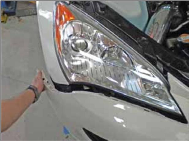
s. Carefully pull out and up on the outside edges of the bumper cover to release it from the clips under the fender and headlight. Take care not to damage the bumper cover.
