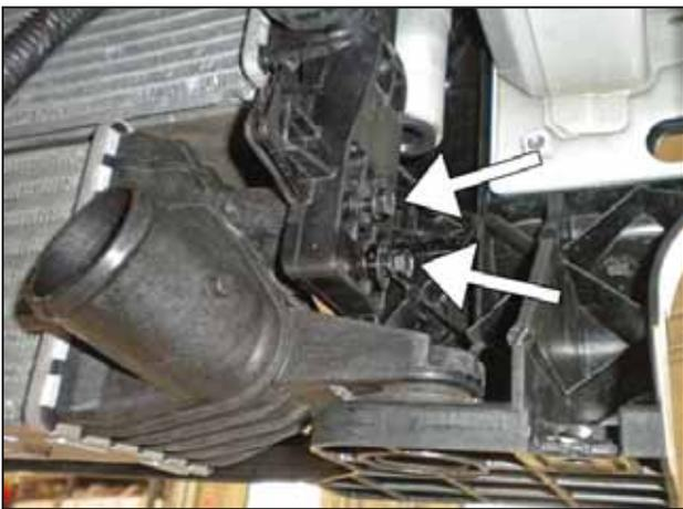
aa. From underneath the car, remove 2 M6 bolts from each side of the intercooler.
