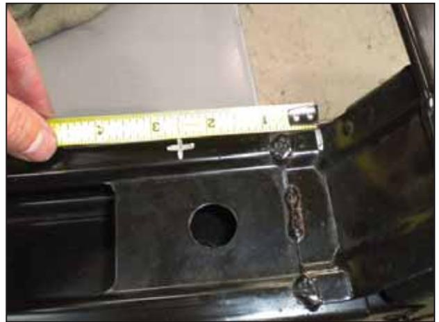
w. Measure 2.5" from the corner of the mount as shown. Mark and drill a 3/8" diameter hole. Deburr and paint the edges of the hole to prevent rust.
