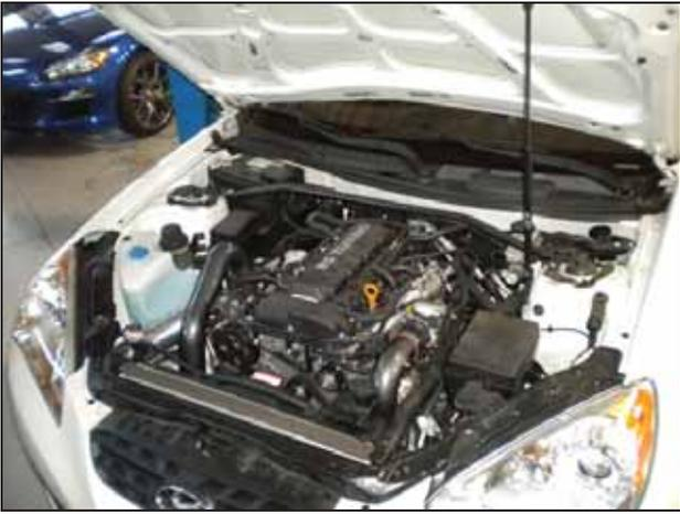
az. Make a final check for clearance between all components, and re-adjust if necessary. Be sure that all fasteners are tight including hose clamps and rubber mounts, and that the electric fan is plugged in before starting the vehicle.
