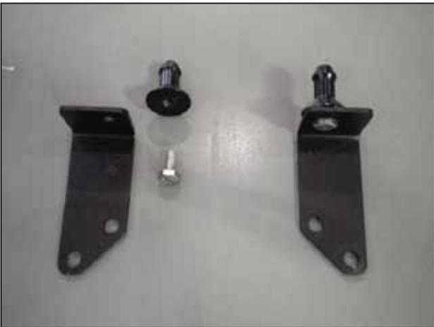
d. Assemble the supplied radiator support brackets as shown using one short M6 bolt and one aluminum nipple for each.
