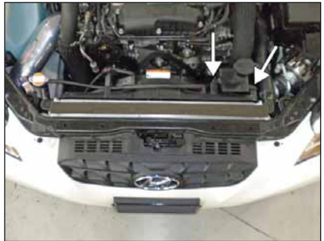
b. Remove the coolant reservoir by removing 2 self tapping screws and disconnecting the hose.
