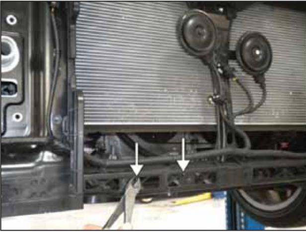
f. Using a pair of flush-cuts or similar tool, trim off the two plastic nubs on the front of the lower cross member.
