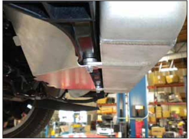
u. For best fit, push the intercooler toward the right side of the car. When the alignment of the shroud and the intercooler looks good tighten all three bolts.
