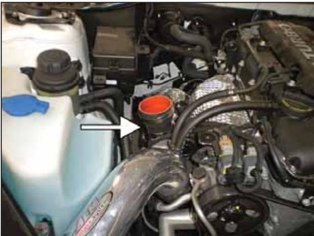
ab. Install the reducer coupler as shown with a #36 and #44 clamp.
