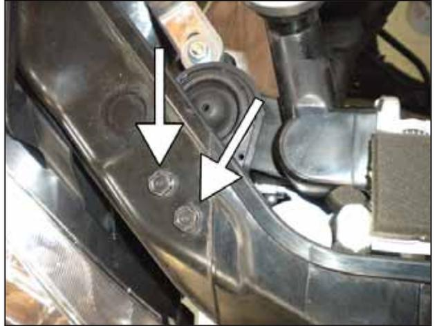
c. Reinstall both upper radiator brackets removed in step 2d.
