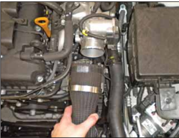
g. Pull the left charge pipe off of the throttle body.
