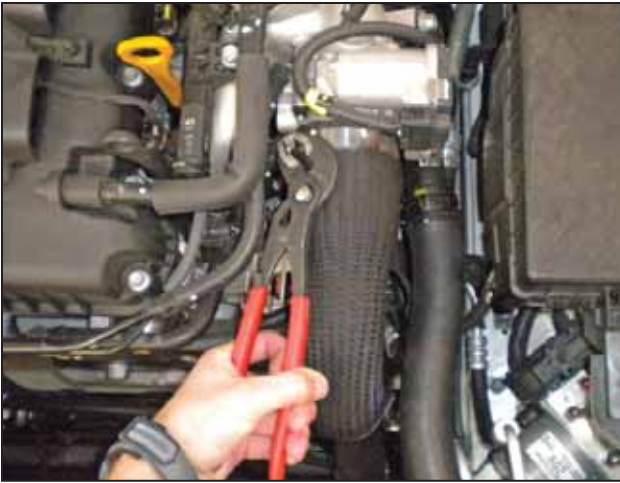
e. Use pliers to remove the “tamper resistant” hose clamp at the throttle body.
