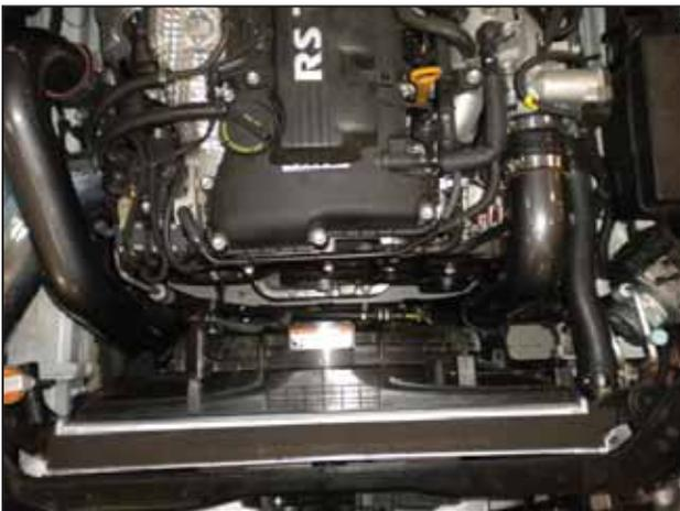
al. Lower the electric fan and shroud into place. Guide the lower tabs on the fan into the mounts on the radiator from underneath.
