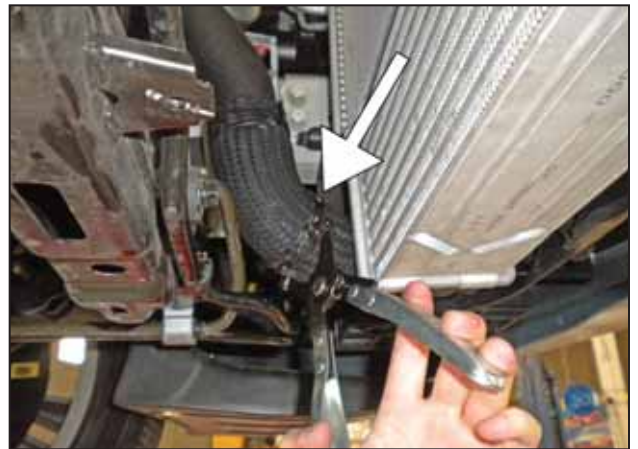
p. Use pliers to squeeze the spring clamp and slide it back on the charge pipe. Do this on both charge pipes.
