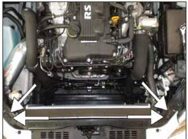
d. Remove the upper radiator mounts by removing 2 M6 bolts on each mount.
