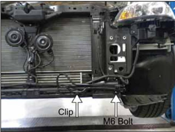
w. Unclip the plastic clip holding the power steering cooler in place. Also loosen the M6 bolt.
