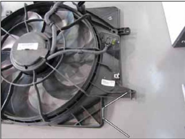
aj. On the right lower corner of the electric fan shroud, mark and trim the area shown for clearance with the charge pipe.
