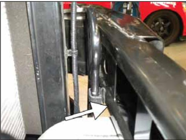
v. On the back of the bumper near the left mount, a hole needs to be drilled for mounting the power steering cooler.
