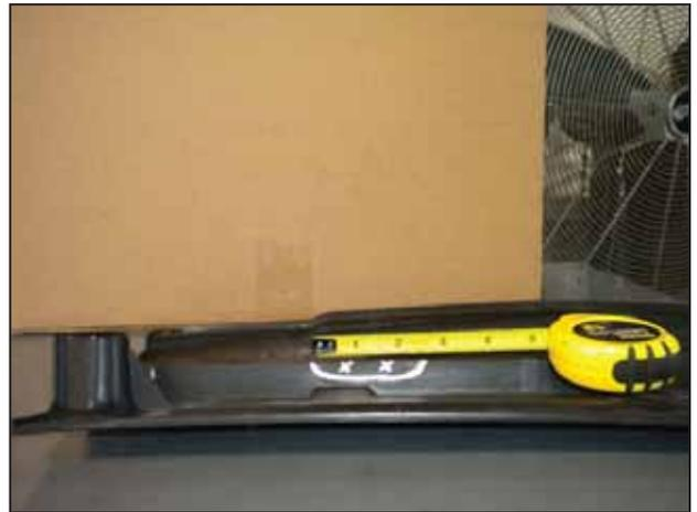
aw. Mark the reinforcement rib on the left side as shown, and trim.
