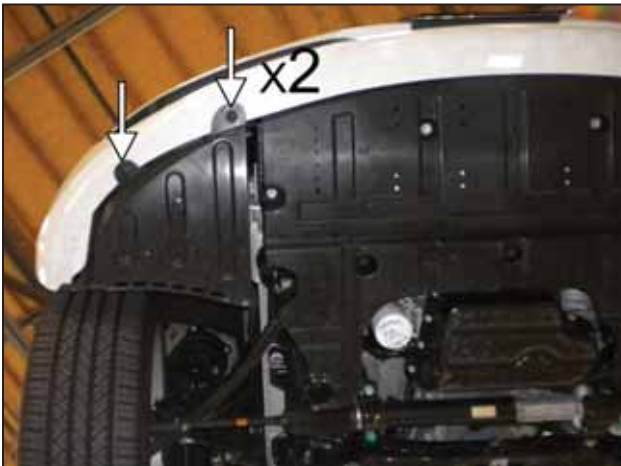
m. From underneath the car, remove 4 clips. Two clips from each side of the vehicle.
