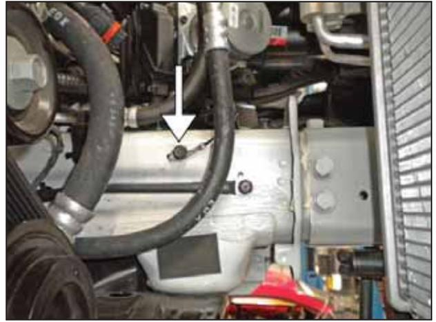
g. On the side of the left frame rail, locate the two M6 bolts used for attaching ground wires. Remove the ground wire from the top bolt location.
