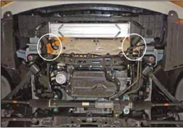
q. Slide the charge pipes off of the intercooler and remove them from the car.
