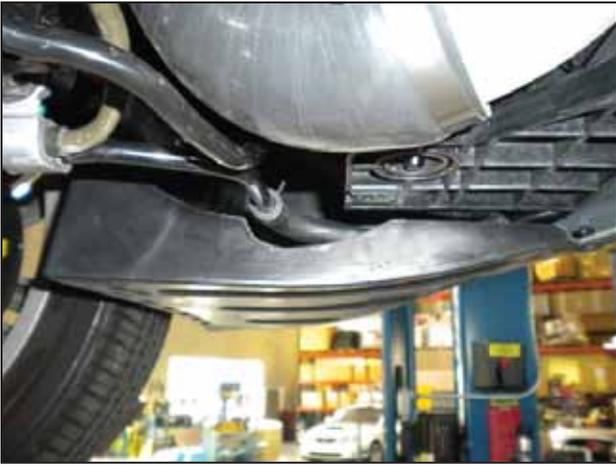
at. Some minor trimming of the fender liner as shown may be necessary to clear the power steering lines.
