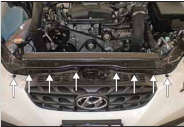
k. Remove the 8 plastic clips securing the front of the bumper cover.
