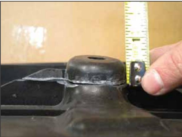
av. Mark the mounts as shown, and remove about 1/2" from the mounts.
