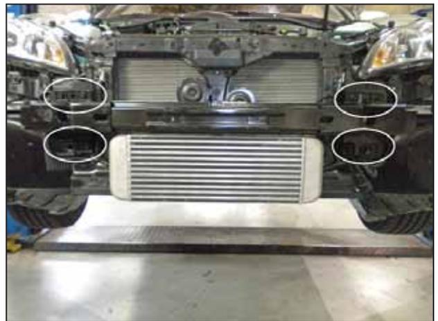
y. Attach the bumper support with the 6 M8 bolts and 2 M6 nuts removed in step 2(u).
