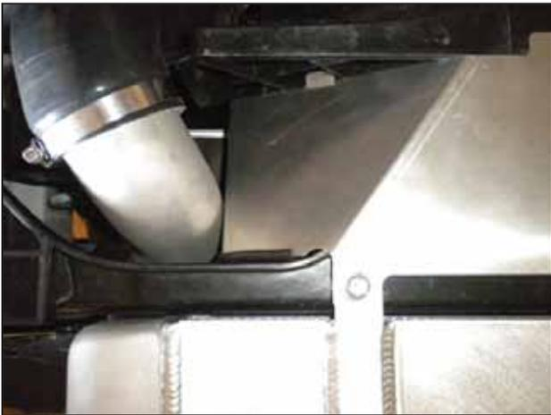
ap. Once the tabs are in position, secure the fan with the two M6 bolts removed in step 2(c). **Plug in the fan** and secure the wiring.
