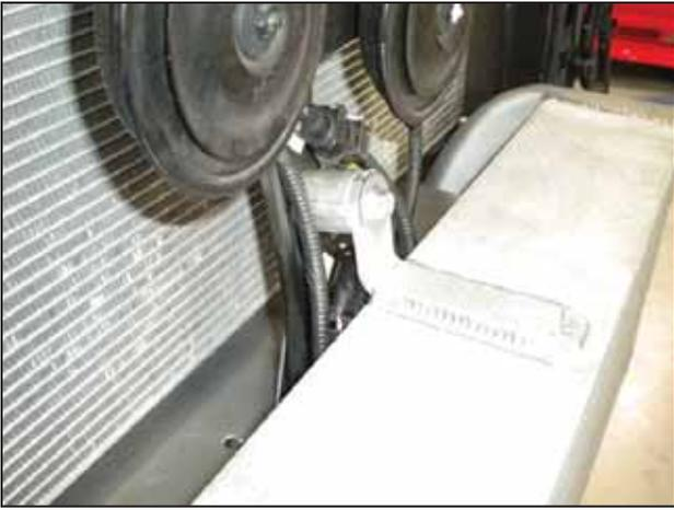
t. Run the top mounting bolt in and push the shroud toward the front of the car to reduce the gap between the intercooler and the shroud.
