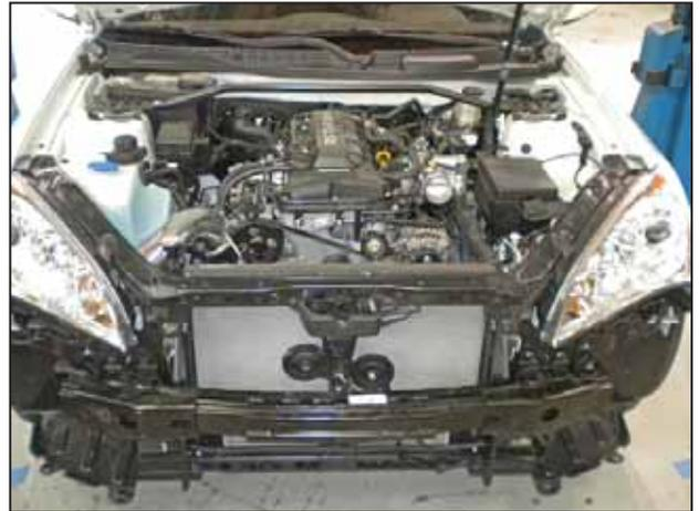
t. Remove the bumper cover and set it aside in a safe location.
