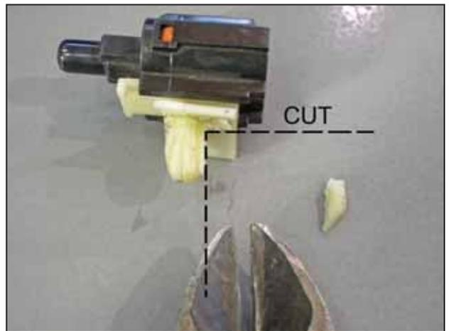
z. Use flush cuts to trim off the "key" on the clip so that the sensor can be rotated slightly. Then reinstall the sensor.
