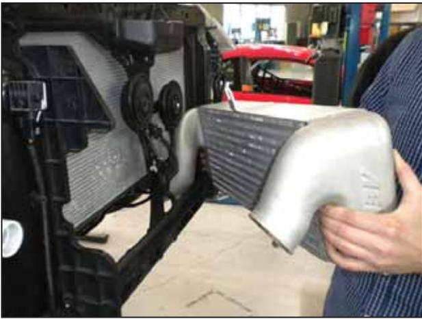
l. Inspect the end tanks of the intercooler and remove any packaging material that may obstruct the inlet and outlet. Begin the installation of the AEM® intercooler as shown. Guide the left intercooler neck into position, then lower the intercooler down, so that the left lower bracket slides under the cross member.
