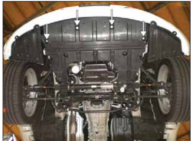
n. Remove the front under tray by removing 4 M6 bolts.
