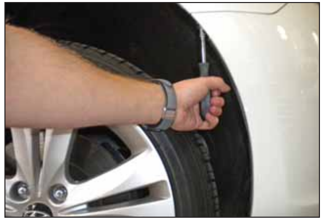
l. Remove one self tapping screw from each side of the bumper cover.
