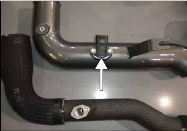
af. Transfer the boost sensor from the OEM charge pipe to the AEM® charge pipe. Attach using the same OEM bolts.
