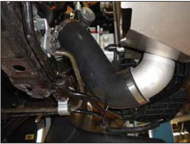
z. Install the lower coupler using two #44 clamps as shown.
