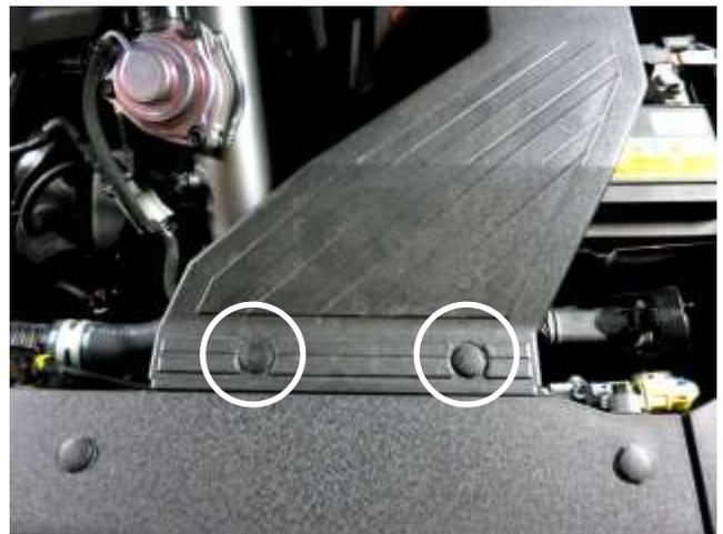
p. Install the stock scoop back into the vehicle with the clips removed in step 2a.
