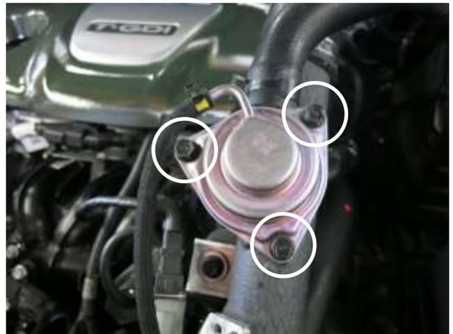
d. Remove the 3 bolts securing the recirculation valve to the stock intercooler pipe, then move the valve to the side of the engine compartment. Note: Do not lose the O-ring under the valve.
