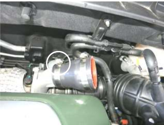
g. Install the provided coupler and hose clamps onto the turbo compressor outlet. Tighten the hose clamp circled at this time to 30 in-lbs.
