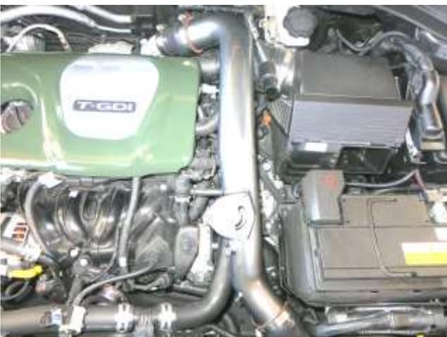
i. Install the AEM upper intercooler pipe into the previously installed couplers. Note: Using warm soapy water may help installation and alignment.
