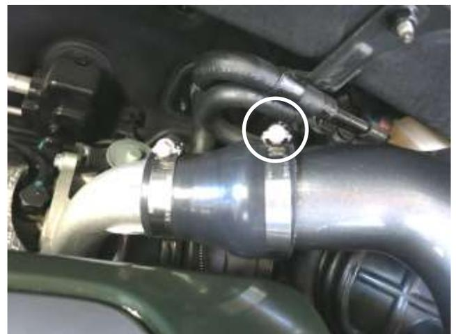
j. Once the AEM intercooler pipe is properly aligned. Tighten the hose clamp circled to 30 in-lbs.
