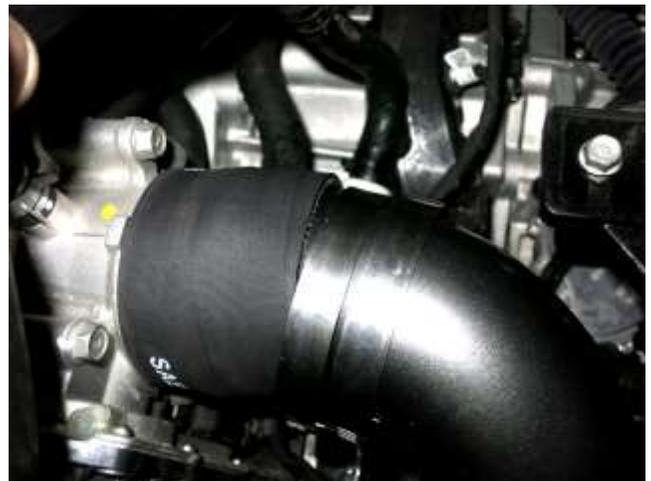
d. Install the provided coupler into the throttle body and install the AEM lower intercooler pipe into the coupler along with hose clamps. Note: Warm soapy water will help with installation.
