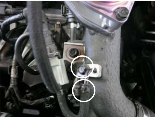
c. Remove the M6 bolt securing the electrical connector. Squeeze on the spring clamp and remove the vacuum hose from the nipple. These will be reused in step 3I & 3m.
