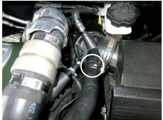
b. Squeeze the spring clamp and work the clamp back off of the turbo recirculation valve hose. Disconnect the hose from the stock intake arm.
