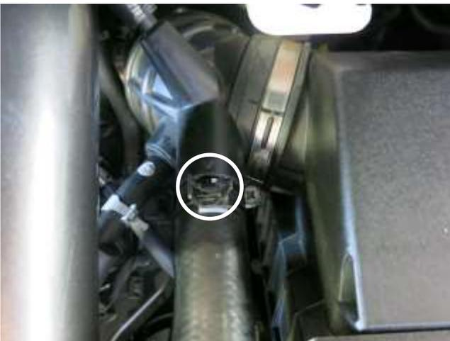
o. Slide the BOV hose back onto the stock intake tube and secure with the stock spring clamp that was removed in step 2b. Note: Soapy water will help with installation.
