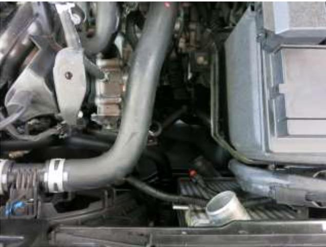
m. Remove the lower intercooler pipe from the vehicle.
