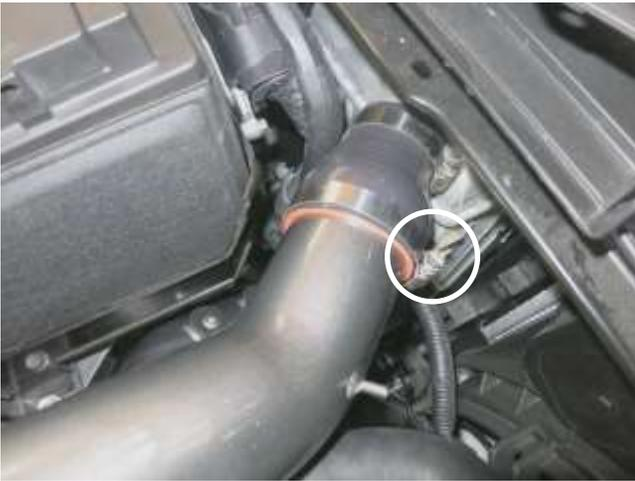
k. Tighten hose clamp circled at the intercooler to 30 in-lbs
