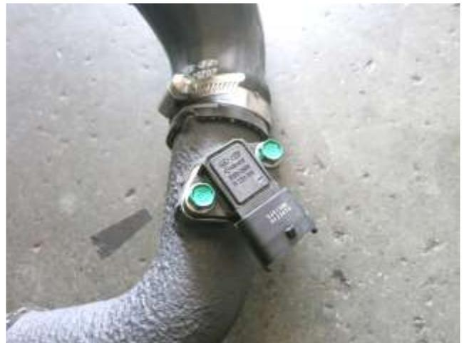
n. Remove the two M6 bolts securing the pressure sensor to the lower intercooler pipe. These bolts will not be reused.
