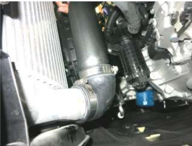
c. Install the AEM intercooler pipe into the coupler. Tighten hose clamp once upper part of tube is aligned to 30 in-lbs.
