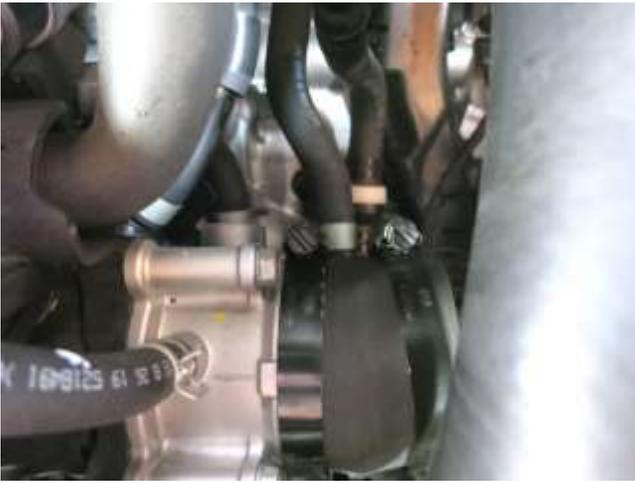
e. After installing the coupler and hose clamps onto the throttle body, make sure the tube is aligned and tighten all the hose clamps at the throttle body and lower intercooler outlet to 30 in-lbs.
