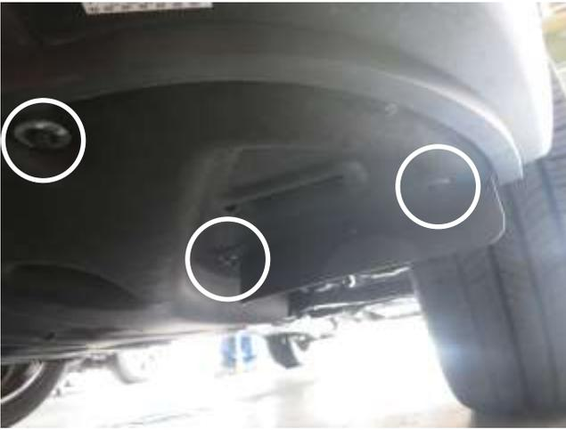
k. Remove the 3 bolts that secure the drivers side splash shield, then lower it down.
