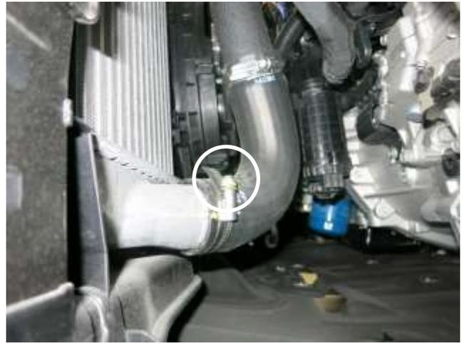
l. Loosen the hose clamp at the lower intercooler outlet from under the vehicle. Note: A hose clamp cap that covers the slot may be present. You can pry it off with a screwdriver or pliers.
