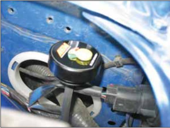
d. Attach one end of 5/32" hose to elbow on filter, and the other end to the filter minder nipple. Trim excess hose.
