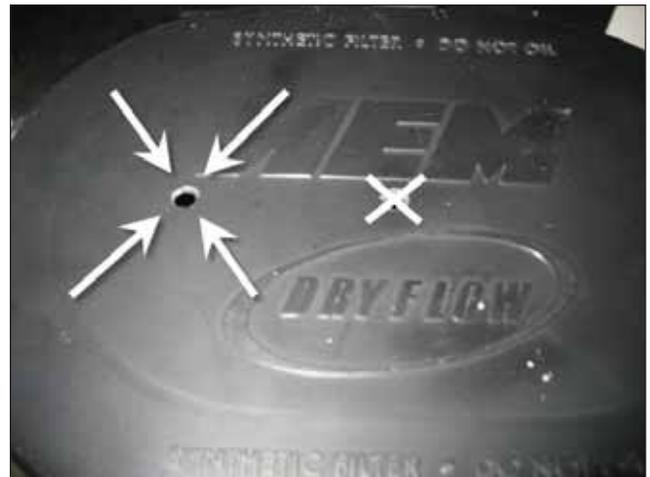
b. Drill 15/64" hole in lid of filter in the specified location.
