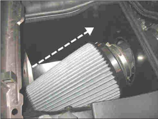
e. Reinstall the air filter onto vehicle. Proceed to step 3.
