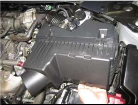
K. Lift up on the bottom of the air box to disengage but do not remove from engine bay.
