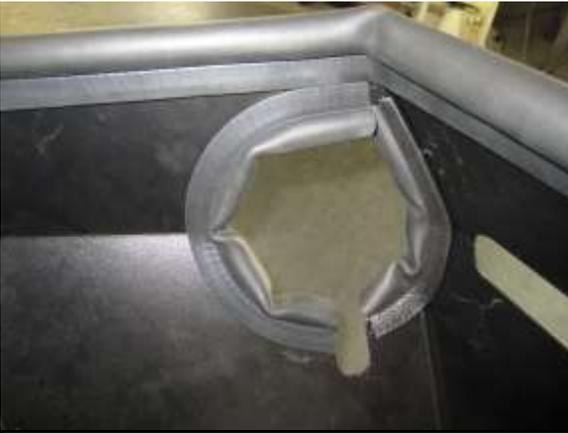
I. Install the rubber edge trim (#16 and 17) around the intake tube opening in the heat shield (#11).
