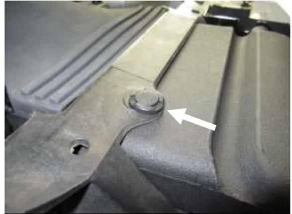
Y. Install the OEM clip as shown.
