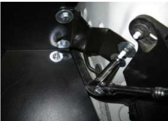
P. Once the heat shield is properly positioned, tighten all nuts to secure the heat shield in place.
