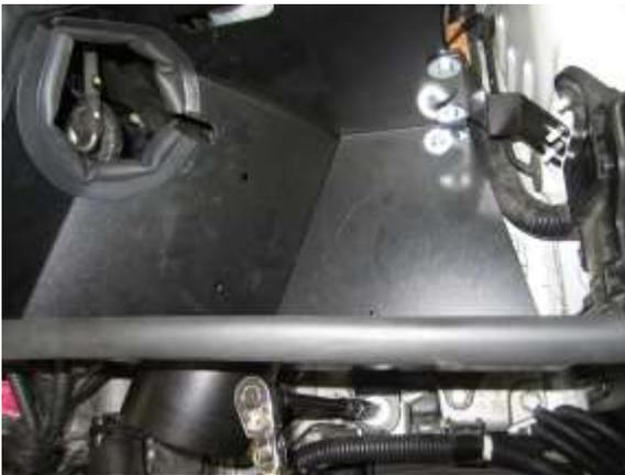
N. Secure the heat shield to the threaded bolt ends with two washers (#5) and two M6 nuts (#4).
