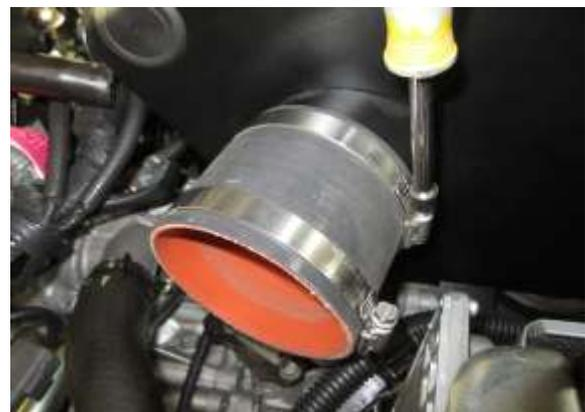
Q. Install the 3.5" coupler (#2) with two #3 hose clamps onto the heat shields inlet, tighten the hose clamp on the heat shield inlet end.
