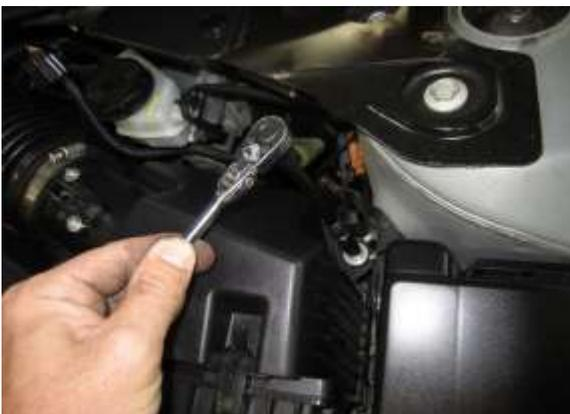
I. Remove the 6MM bolt that secures the lower air box in place.
