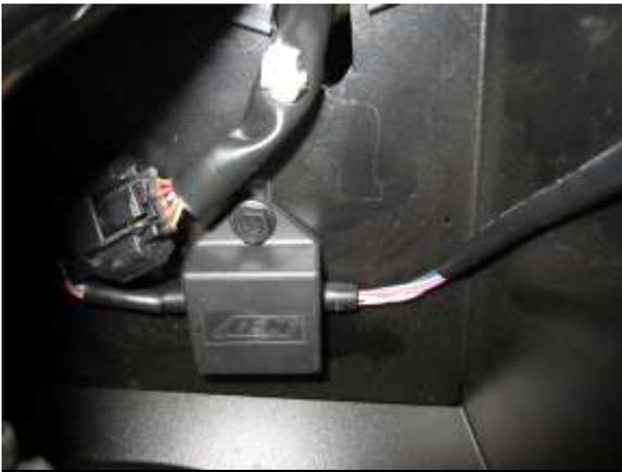
AJ. Mount the ETI using one 6MM bolt (#15) and 6MM nut (#4).
