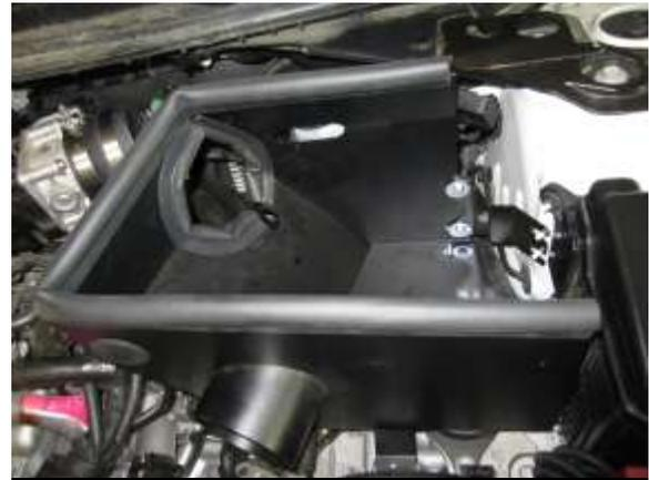
M. Place the heat shield in the vehicle's engine bay, ensuring the threaded ends of the bolts from step G align with the openings on the bottom side of the heat shield.
