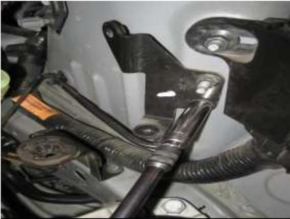
S. Remove the two 6MM bolts securing the factory air box bracket to the inner engine bay wall.
