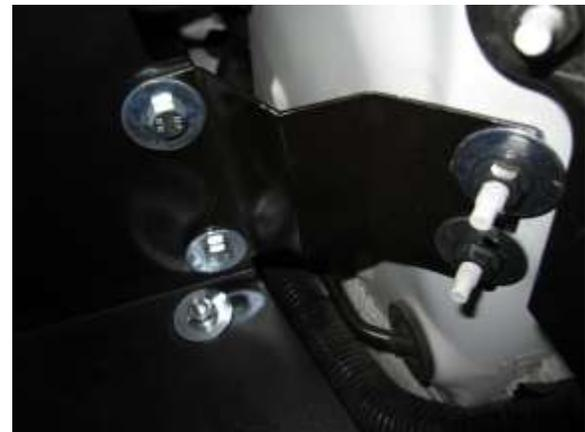
O. Align the heat shield's bracket with the two studs, secure in place using two washers (#5) and the two OEM nuts removed in step 2 S
