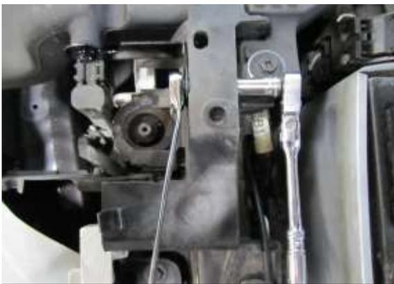
AB. Secure the air inlet scoop's hardware.
