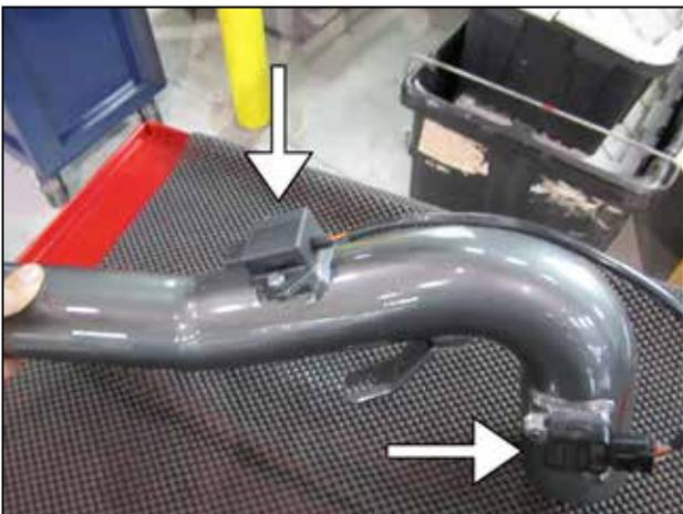
b. Remove the MAF sensor from the stock airbox. Install the MAF sensor and ETI module onto the lower inlet pipe with the provided hardware. Once installed connect the ETI module harness to the MAF sensor as shown.
