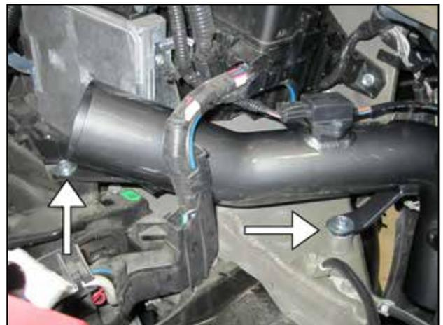
c. Install the lower inlet pipe, securing the inlet pipe brackets with the provided hardware.
