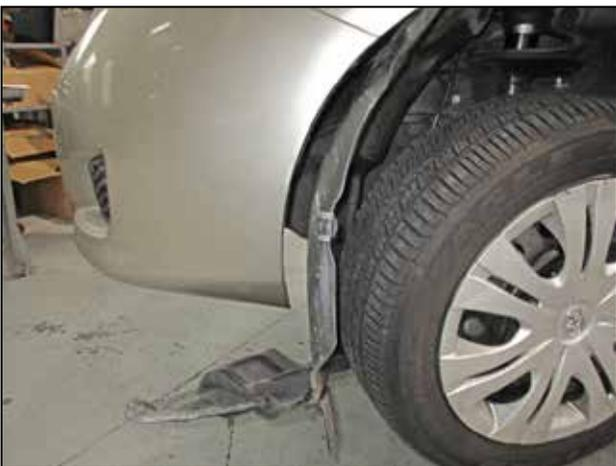
o. Remove the clips securing the wheel well liner to the inner fender allowing it to hang down as shown.
