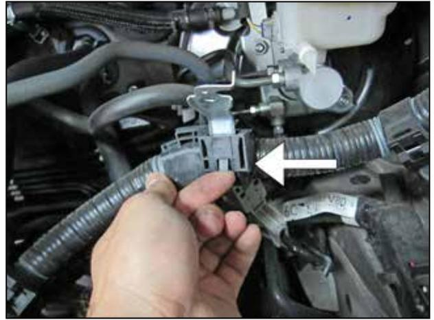
l. Remove the metal bracket from the harness, lift the tab up and remove the bracket as shown.
