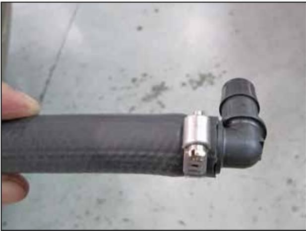
j. Slide the 5/8" hose over the 90° plastic elbow and secure it with the hose clamp (# 99024.032).
