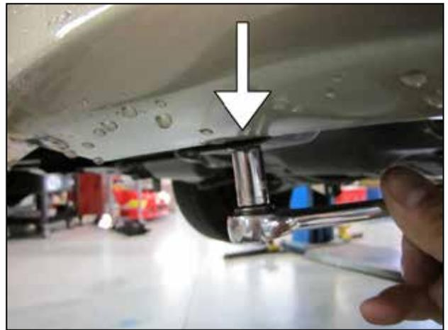
n. Locate the 2 bolts at the bottom of the vehicle that secure the lower portion of the plastic wheel well liner to the front bumper; remove these two bolts.
