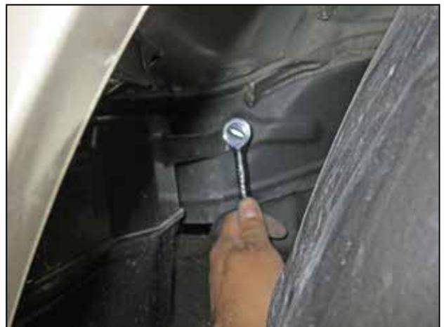
p. Remove the 2 bolts and nut that secure the resonator box to the inner fender well, remove the resonator box from the vehicle.
