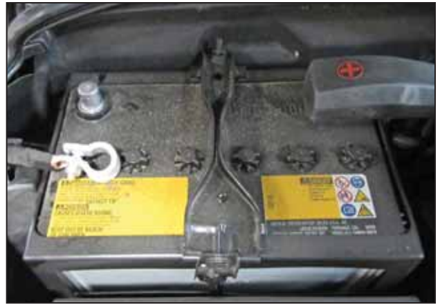
b. Disconnect the negative battery terminal.
