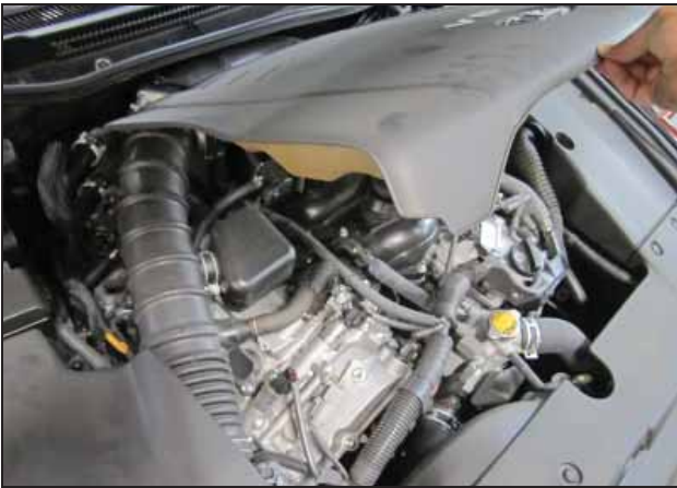
c. Remove the engine cover.
