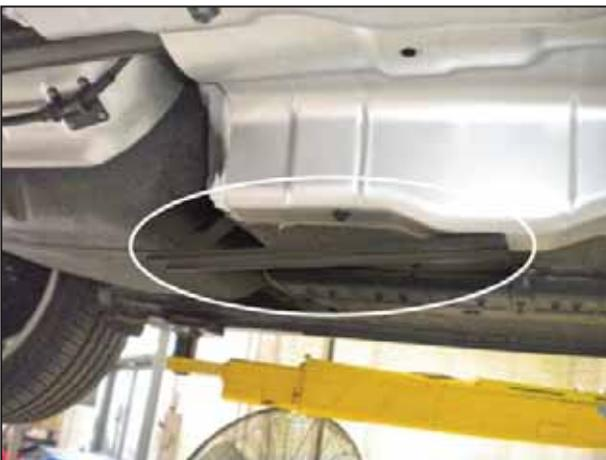
o. Rotate the brace out of the way.
