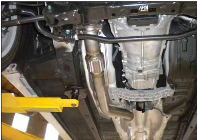
f. Front exhaust pipe installed.
