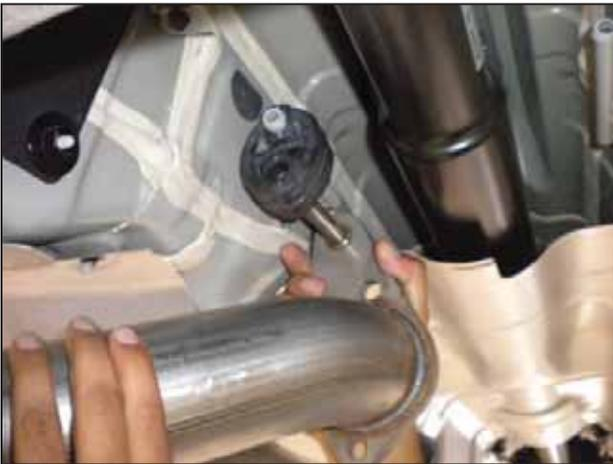
d. Slide the hanger located on the front exhaust pipe into the OEM rubber isolator.
