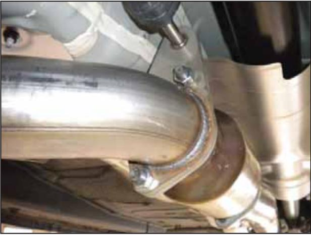
h. Connect the OEM catalytic converter/AEM® middle exhaust pipe assembly to the front AEM® exhaust pipe. Sandwich the OEM metal exhaust gasket between the two pipes and secure using the two supplied nuts (1-1005).
