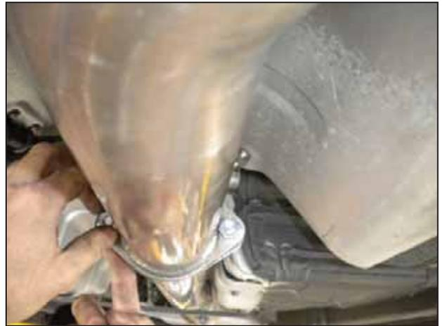
k. Install the two supplied M10 nuts (RHNA-M10X125) on the bolts installed in step 3i.
