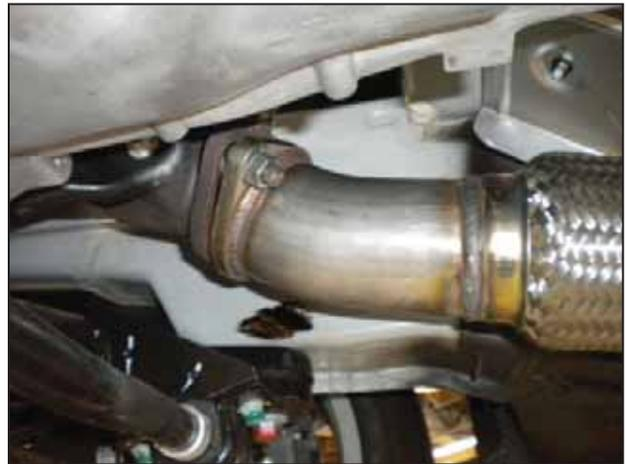
e. Install the two supplied nuts (1-1005) on the studs as shown, keep loose.
