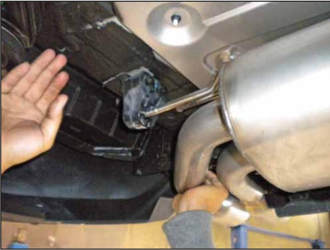
n. Install the passenger side muffer hanger into the rubber isolator.
