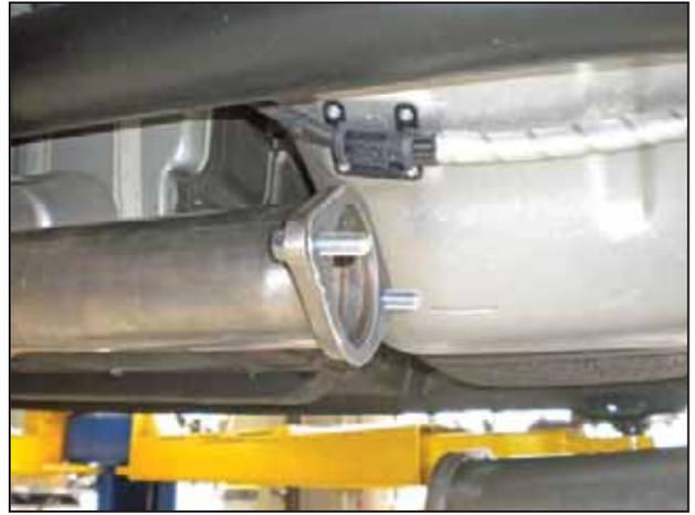
i. Install the supplied M10X1.25X35mm bolts (RHBA-M10X125X35) and the supplied gasket (RM-CB83) as shown.
