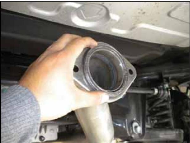
l. Install the supplied gasket (RM-CB81) on the end of the rear exhaust pipe.
