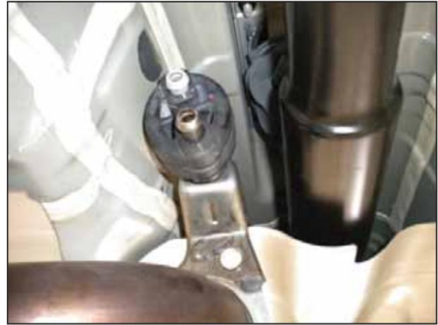
l. Unhook the hanger from the rubber isolator located on the rear flange of the front exhaust pipe.
