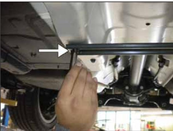
m. Remove the passenger side bolt securing the brace shown.
