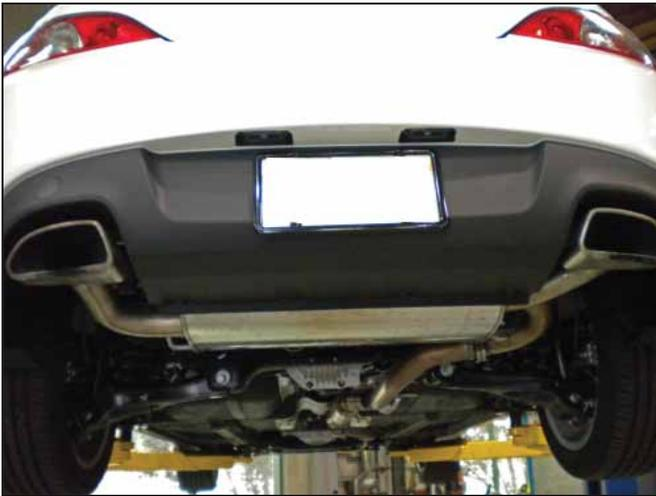
a. Stock exhaust system installed.
