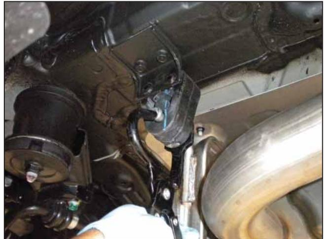
d. Unhook the driver side hanger from the rubber isolator.
