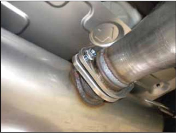
p. Secure the rear exhaust pipe to the muffer using the supplied M10X1.25X25 bolts (RHBA-M10X125X25) and nuts (RHNA-M10X125).
