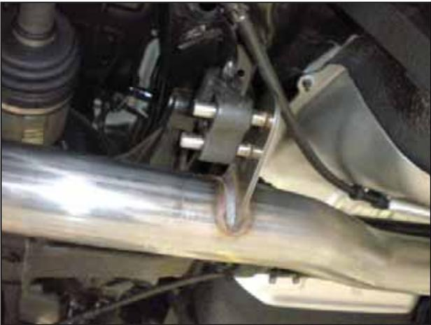
j. Install the rear AEM® exhaust pipe aligning the hanger with the rubber isolator.
