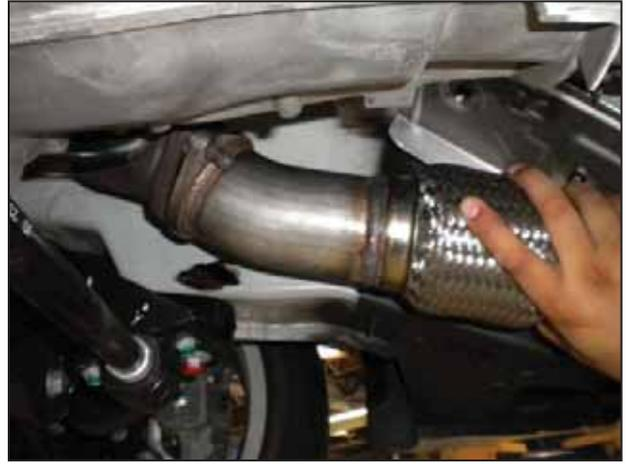
c. Align the front AEM® exhaust pipe with the studs located on the turbo manifold
