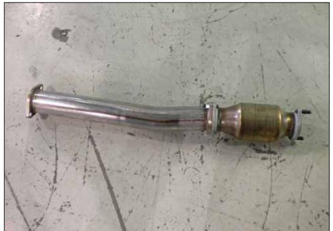
g. Create an assembly outside of the vehicle with the middle AEM® exhaust pipe and the OEM catalytic converter using the two supplied nuts (1-1005) and the OEM metal gasket between the two parts.
