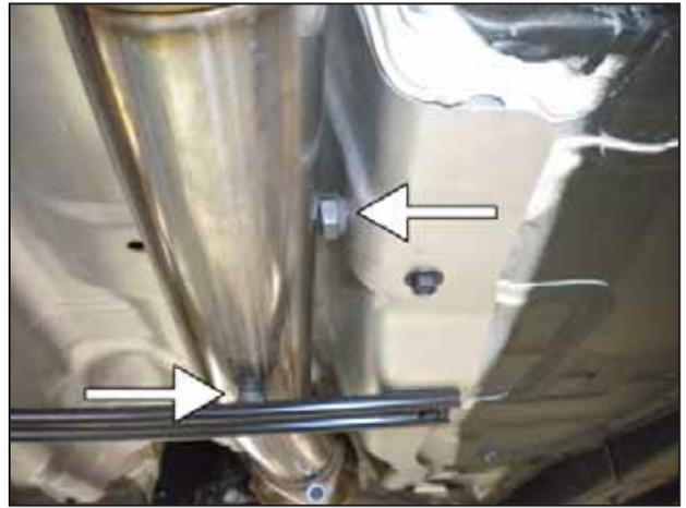
q. Re-install the brace rotated in step 15 of the instructions. Using the OEM nuts space the exhaust as shown. Tighten all of the nuts and bolts associated with the exhaust system.
