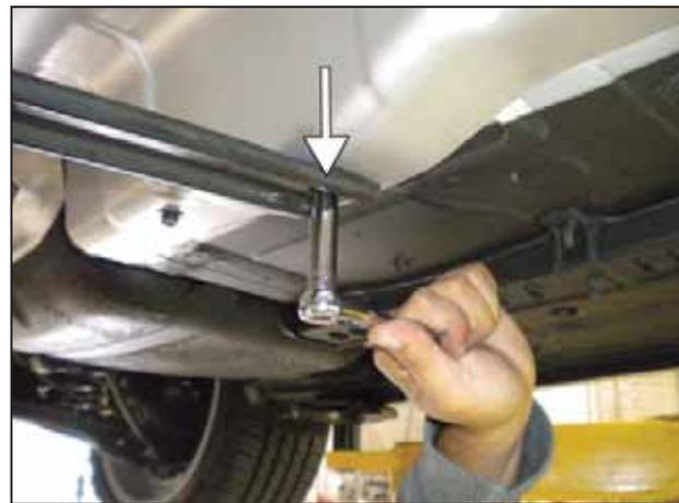
n. Loosen but do not remove the driver side bolt securing the brace.
