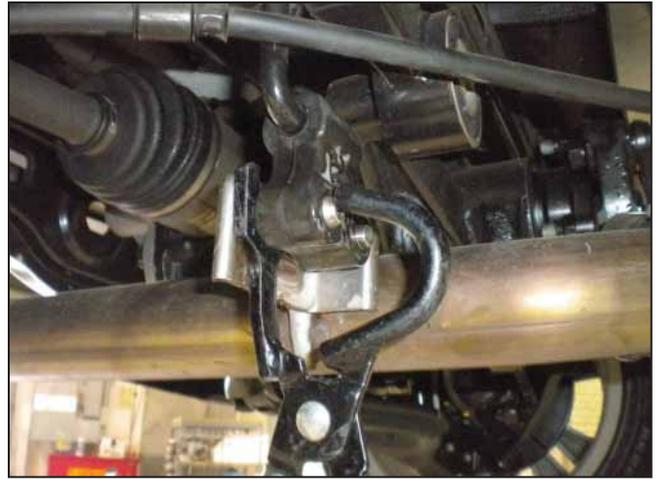
f. Unhook the hanger located on the rear exhaust pipe that was connected directly to the muffler by flipping the rubber isolator up.
