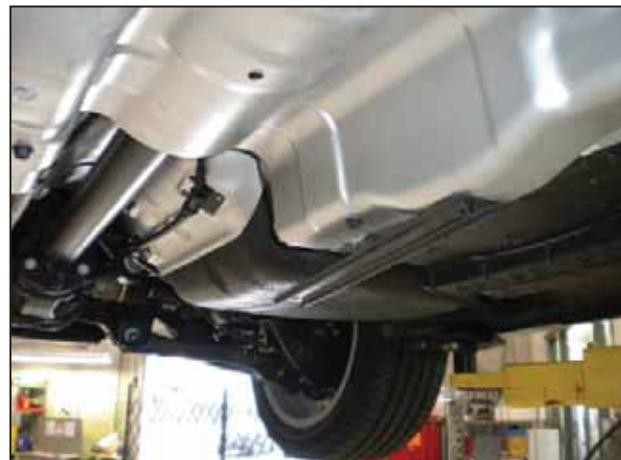
p. OEM exhaust system removed.
