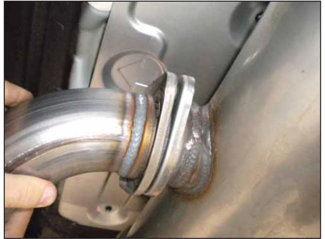
o. Align the muffer with the rear exhaust pipe.
