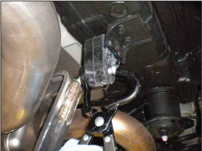
c. Unhook the passenger side hanger from the rubber isolator.
