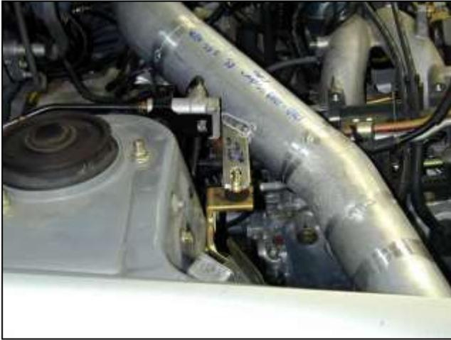
f. Once you line up the bracket to the rubber mount, secure with washer and nylok nut. Refer to the diagram below.
