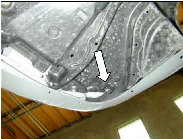
o. Remove the two clips from the underside splash shield. Peel back the splash shield.
