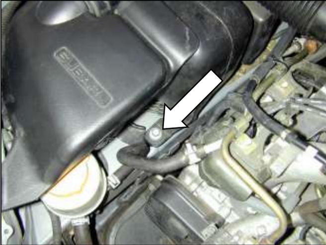
c. Loosen and remove bolt. This bolt will be used with the installation of the AEM® intake system.
