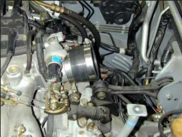
b. Attach the reducer coupler to the throttle body and secure with the provided hose clamp. Loosely attach the second hose clamp to the open end of the coupler.
