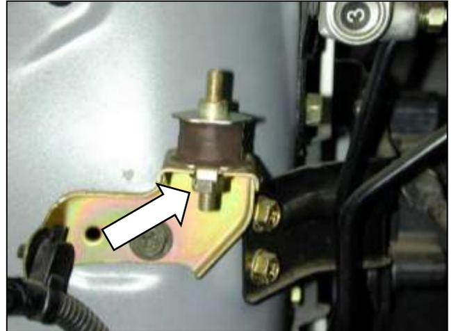
c. Remove the stock rubber mount by loosening and removing the nut underneath the bracket. This mount will be replaced with a new one provided in the kit.
