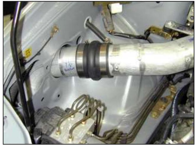
r. Once the lower intake pipe is in place, secure both pipes with the hump hose. Fasten with the provided hose clamps.
