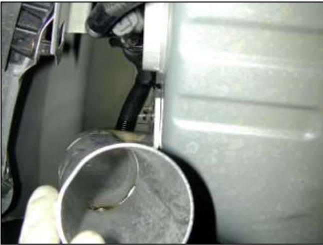
q. Attach the lower intake pipe bracket to the ABS unit's stud that is located in the passenger fender well. Secure with provided washer and original nut.
