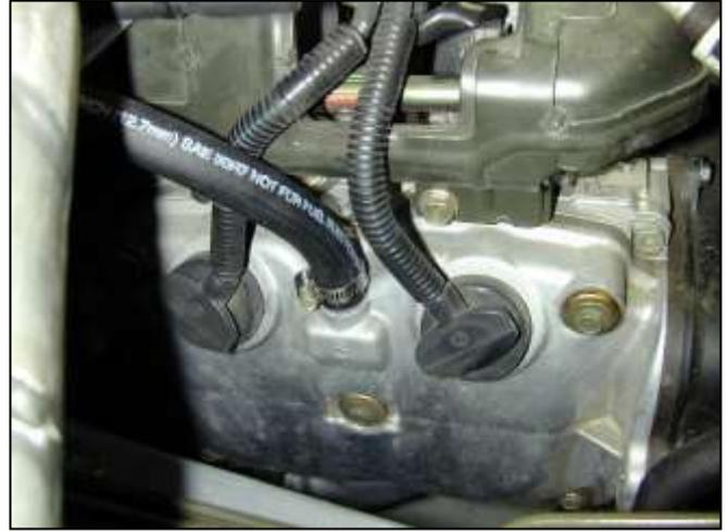
l. Attach the breather hose to the passenger side valve cover and secure with provided hose clamp.
