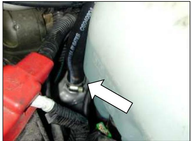
n. Attach the breather hose to the driver's side valve cover and secure with the provided hose clamp.
