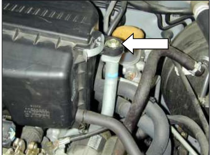
f. Loosen and remove the bolt on the driver's side.
