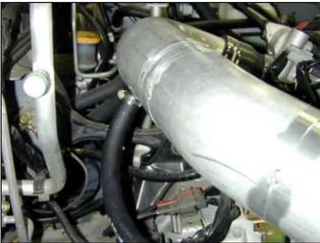
m. Attach the other end of the breather hose to the upper intake pipe and secure with provided hose clamp.
