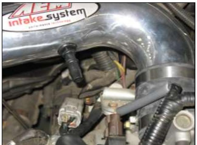
j. Insert 1/2" connector into upper intake pipe.
