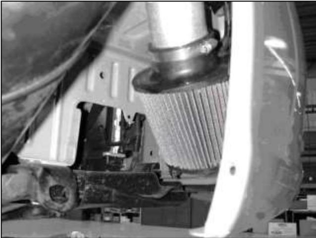
s. Attach the air filter element and secure. Ensure the air filter has proper clearance.
