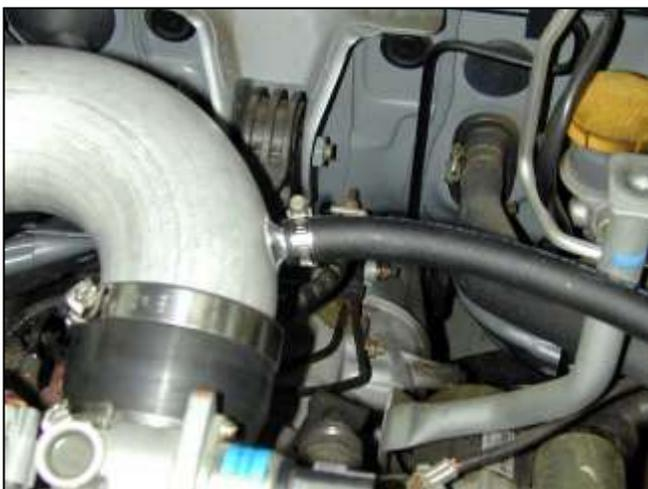
o. Attach the other end of the breather hose to the upper intake pipe and secure with provided hose clamp.
