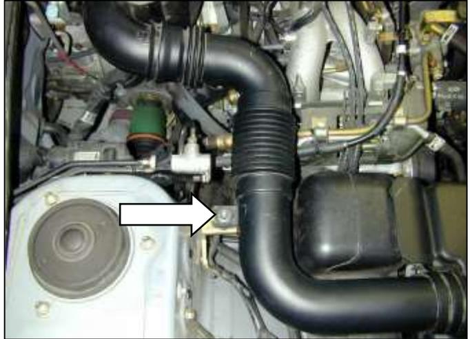
d. Loosen and remove nut.
