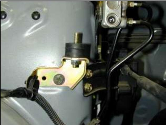
d. Insert the new rubber mount into the bracket. Secure with washer and nylok nut.
