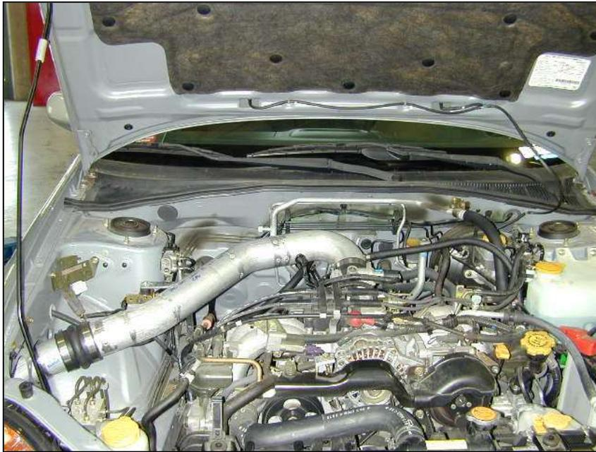
AEM<sup>®</sup> intake system installed
