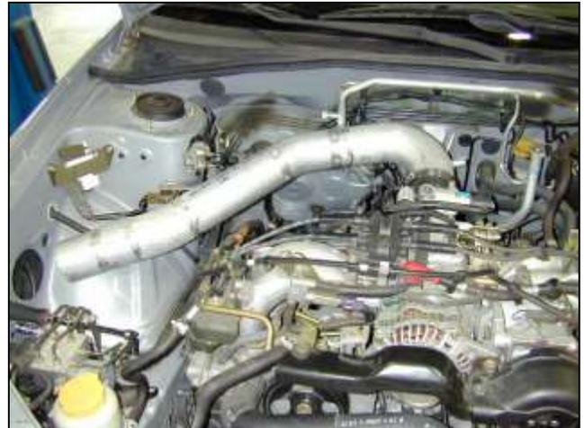
e. Insert the upper intake pipe. Line up the bracket to the newly installed rubber mount.
