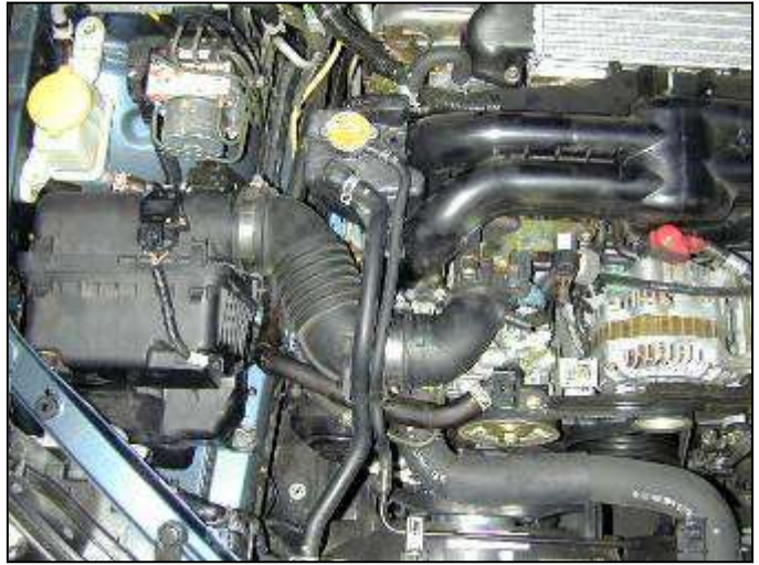
d. Unplug the MAF sensor.
