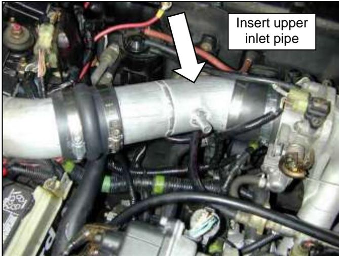
j. Attach the upper inlet pipe as shown. First attach the hump hose to the lower inlet pipe. Then attach the elbow side to the throttle body.
