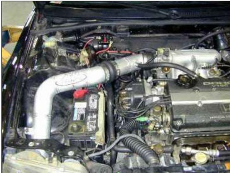
AEM® intake system installed
