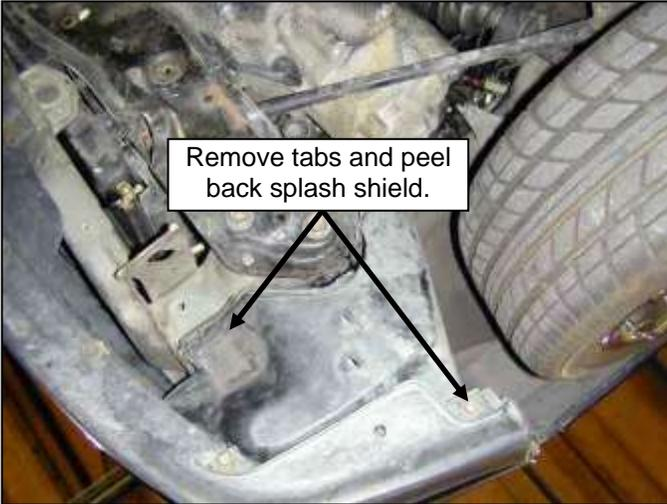
c. Remove the two tabs that secure the lower splash shield. Peel down to gain access to the cavity left by the resonator.
