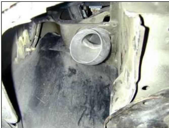
l. Make sure the lower inlet pipe clears the newly widened opening. Attach the air filter element and secure.
