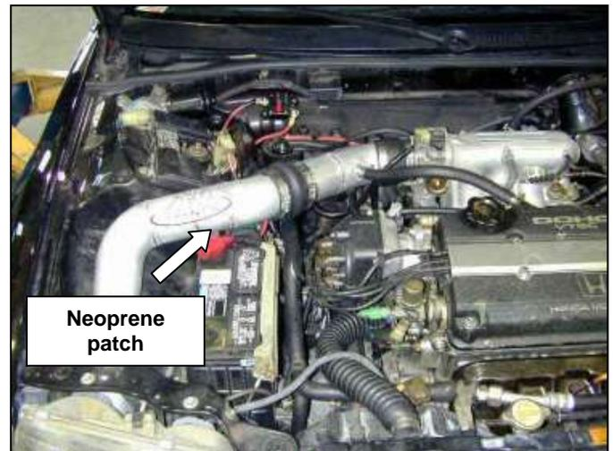
m. Install the neoprene patch onto the intake pipe so it shields the intake pipe from the positive battery terminal.
