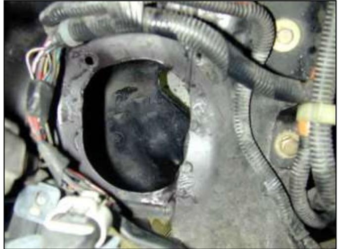
d. The cavity left by the resonator must be enlarged for clearance of the AEM<sup>®</sup> intake pipe. The lower inlet pipe is 3.00" in diameter. You will need to open up the hole to accommodate the pipe diameter. A minimum of at least 3.25" diameter is recommended. The use of a specialized power tool will be needed to cut through the inner fender so the AEM<sup>®</sup> intake pipe is able to clear the inner fender opening. Remove any burrs and line the fender opening with the rubber edge trim.
