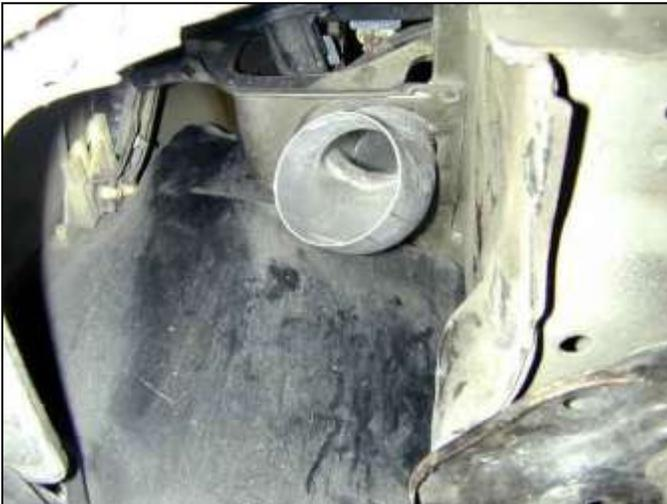
e. Ensure that any rough or sharp edges are smoothed and that the AEM<sup>®</sup> intake pipe is able to clear the opening without touching any part of the inner fender. Test fit the intake pipe to ensure there is adequate clearance.
