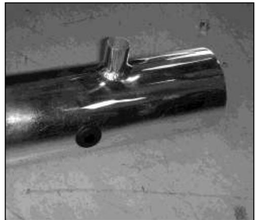
c. Install the supplied grommet into the intake pipe as shown.
