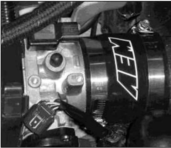
d. Install the hose coupler onto the throttle body. Slide two #48 hose clamps onto the coupler, securing only the hose clamp on the throttle body side.
