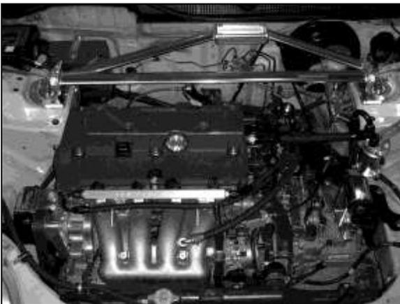
b. Factory airbox system removed from the vehicle.
