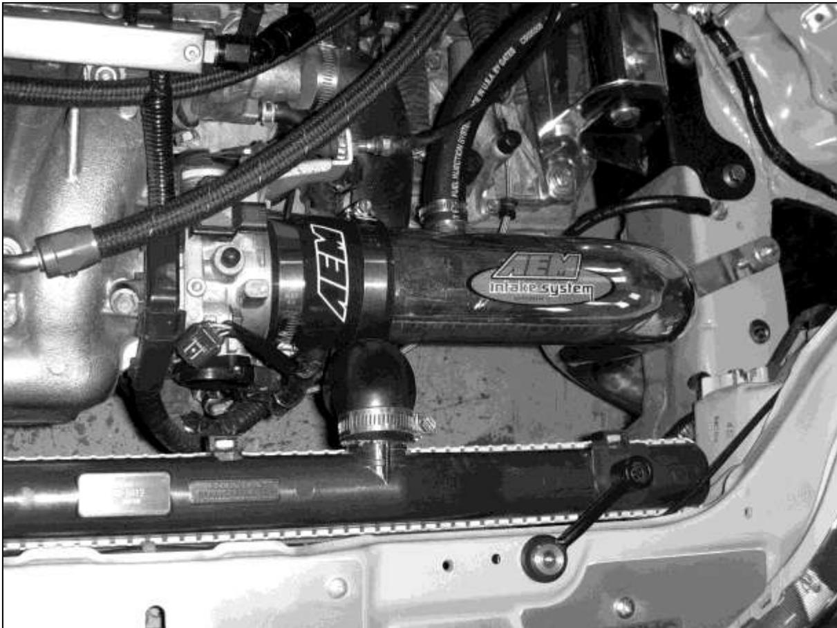
j. Position the intake pipe assembly in the engine bay so that it does not make contact with vehicle. When proper fitment is achieved, tighten all hose clamps and the nut on the rubber mount.
