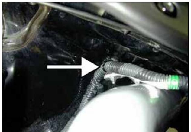
g. Place the intake support bracket behind the washer on the rubber mount as shown. Refer to the diagram on the following page for proper rubber mount assembly.
