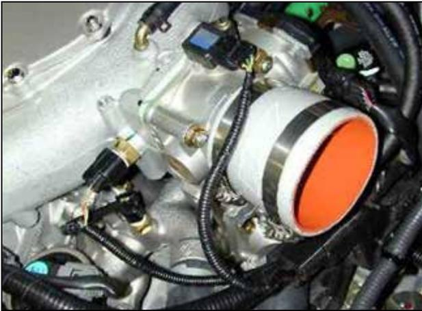
b. Install the coupler onto the throttle body utilizing the supplied hose clamps.
