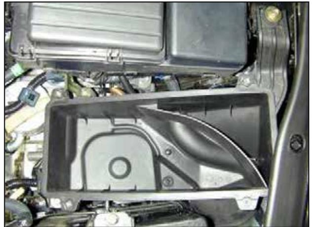
f. Remove the two bolts that hold the lower air box to the chassis. Remove the lower air box from the vehicle.
