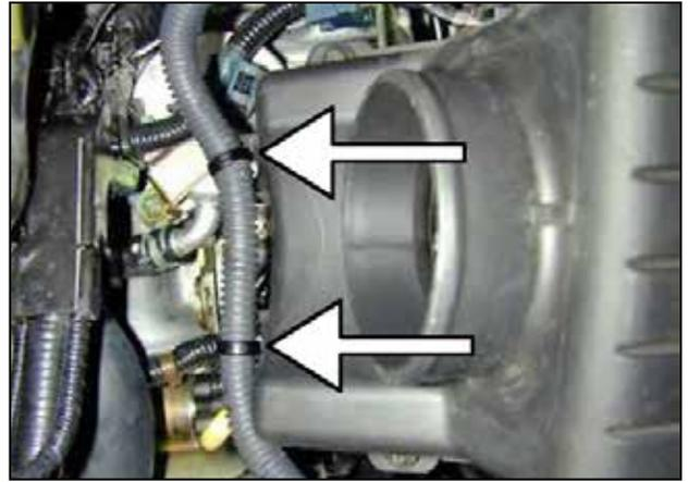
d. Carefully lift the upper air box. Pinch the bottoms of the wire ties with pliers and remove them from the upper air box. Remove the upper air box and air filter from the vehicle.
