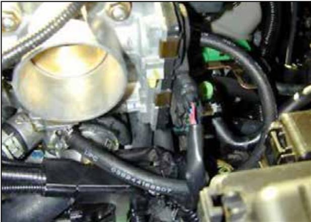
i. Remove the stock breather/coolant hose system. Route the supplied 5/16" ID hose as shown. Secure the hose to both coolant nipples with the supplied 3/4" hose clamps.
