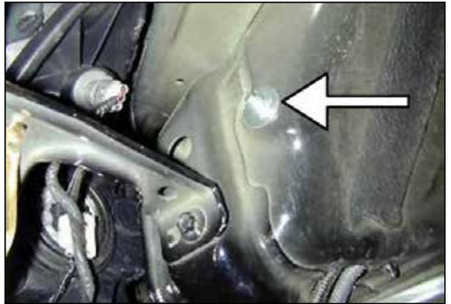
e. Secure the rubber mount stud from the inside of the fender well with the supplied washer and lock nut.
