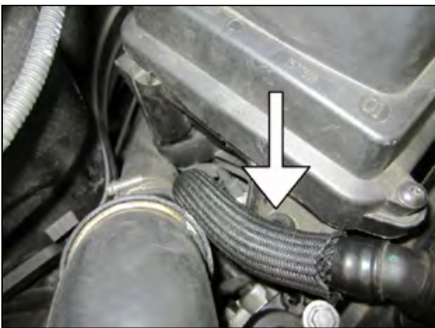
c. Remove the lower Torx screw and plastic grommet insert at the passenger side foot of the stock air box using a T20 Torx bit. Retain the Torx screw for future use.
