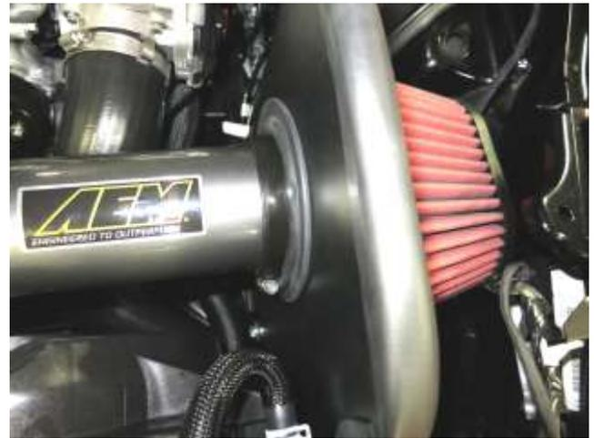
l. Slide the clamp through the heat shield and torque to 30in-lbs ensuring that the clamp is completely engaged beyond the lip at the end of the filter.
