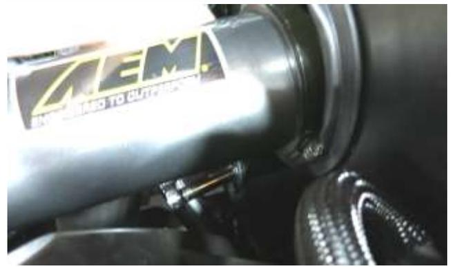
n. Add the nut and washer to the rubber mount under the tube on the heat shield. Position the tube and filter for optimal alignment and tighten this nut and the upper heat shield bolt.
