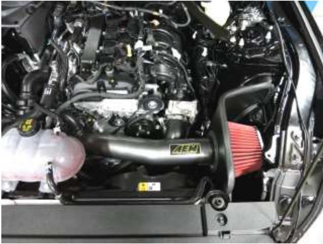
Finished installation of AEM Intake System.
