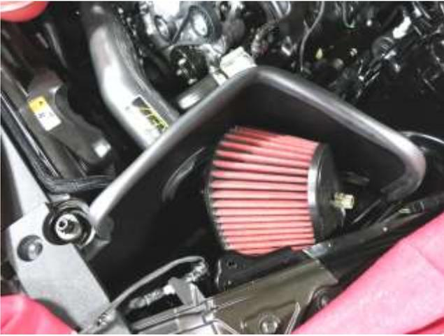
k. Install the included clamp on filter and maneuver the filter into position on the tube as shown.
