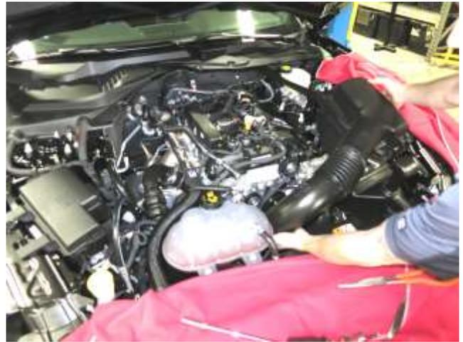
f. Remove the factory intake assembly by lifting out as shown.
