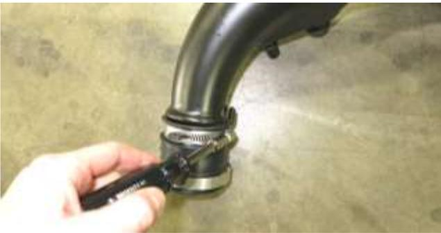
a. Use a 7mm socket to remove the coupler from the factory intake tube.
