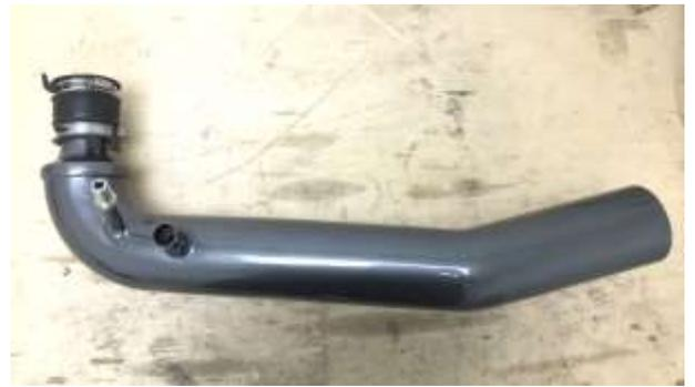
b. Position the coupler on the tube approximately as shown. Install quick disconnect fitting on tube. Torque the clamp to 30in-lbs or until snugly secured to tube.
