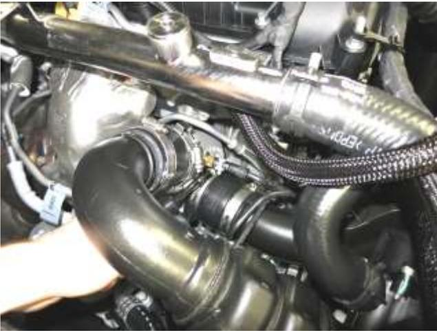
e. Use a 7mm socket to loosen the hose clamp securing the coupler to the turbo compressor inlet and remove the coupler from the turbo.
