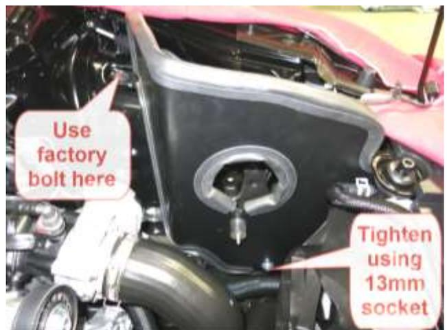
d. Install heat shield assembly and fully tighten lower bolt after starting upper bolt.
