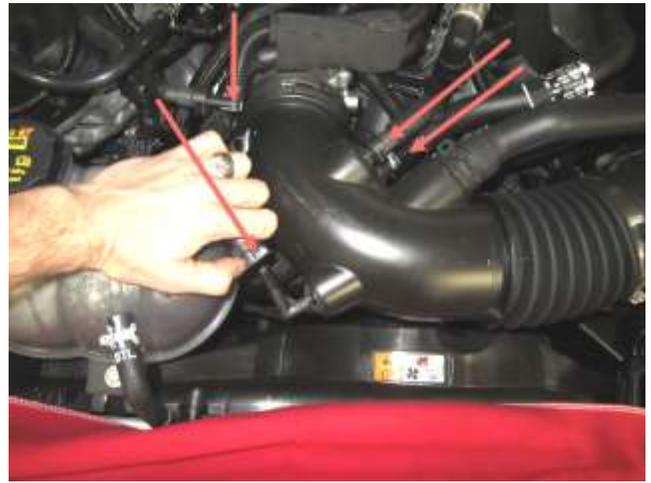
b. Release the three quick disconnect fittings from the factory intake duct and loosen its hose clamp at the throttle body.
