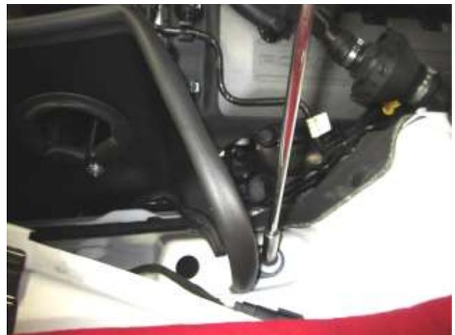
d. Reinstall the factory fastener at the upper mounting tab location of the heat shield.
