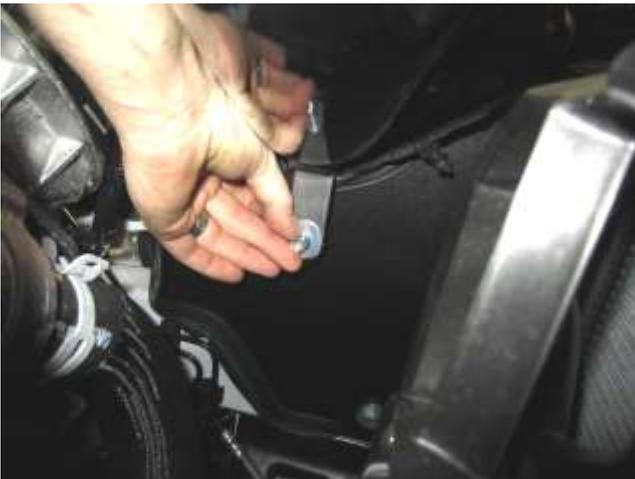
i. Install washer and nut on the bracket on the underside of the intake tube.
