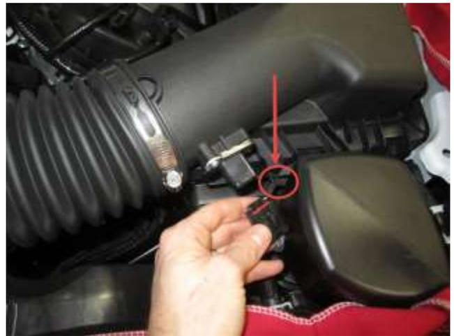
d. Disconnect MAF sensor wiring and use needle nose pliers to pry the retaining clip out of the airbox (circled above). Remove the MAF sensor using the included TORX key and set aside.
