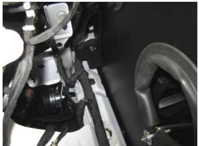
b. Lower the heat shield into the vehicle taking care to align the shield between the fresh air supply and the radiator as shown above.
