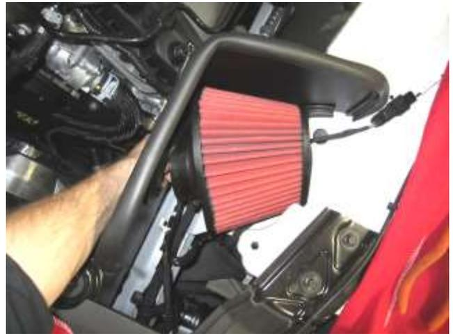
h. Install remaining hose clamp on the filter and lower the filter into the vehicle as shown and twist into place once the flange has started on the end of the tube.
