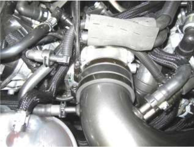
g. Lower the tube into the vehicle aligning the filter end in the heat shield first and then slipping the hose over the throttle body. Push on all lines as shown above until they click on securely. Ensure that wiring harness remains in front of the bracket on the bottom of the tube and reconnect to the MAF sensor.
