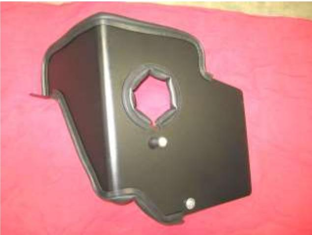
a. Assemble the heat shield according to the exploded view on page 2 of this document as shown including the edge trims & rubber mount below the intake tube hole.
