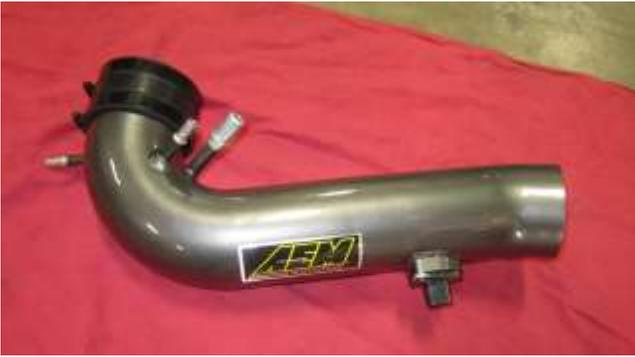
e. Assemble the intake tube components as shown above including the hose, clamps, and MAF sensor.
