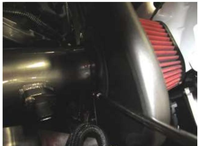
j. Slide filter clamp through the heat shield hole and tighten on the engine side of the shield ensuring that the clamp remains fully engaged on the filter.
