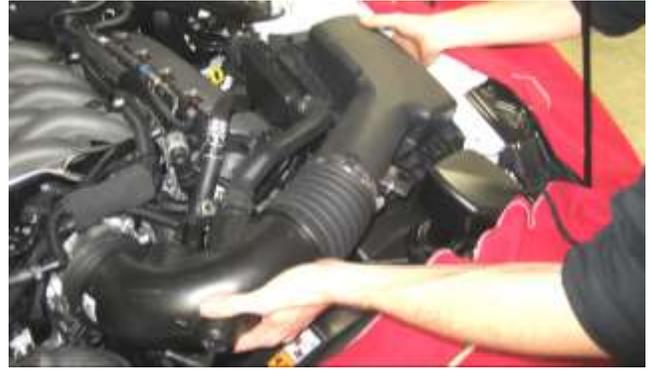
f. Pull the intake duct off the throttle body and lift out the factory intake assembly including the sound tube.
