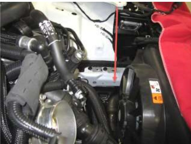
c. Using the bolt & washer assembly as shown on page 2, start the bolt into the threaded hole in the chassis as shown above.
