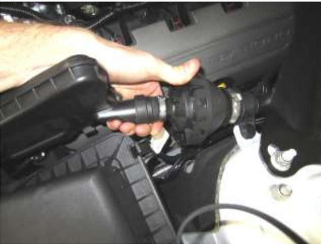
c. Disconnect the sound transfer tube where shown above by pulling the hose off or cutting off its clamp. Use the cap in the kit to cover the hole.
