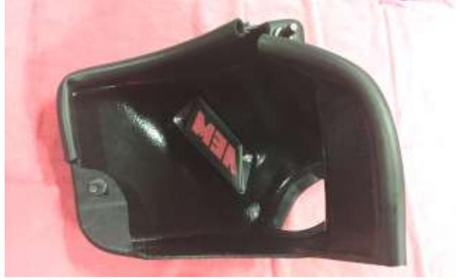
b. Assemble the heat shield components as shown above according to the diagram on pg2. Trim the edge trim as needed.
