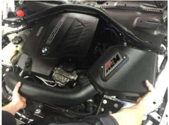
d. Lower the assembled system into the engine bay. Seat the airbox into its two corresponding rubber mounts taking care to ensure that the factory wiring is oriented in such a way that it will not be stressed.
