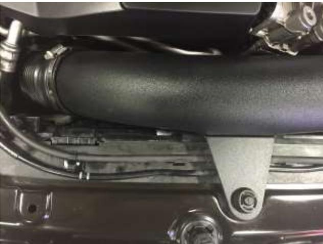
e. Install the intake tube into the turbo inlet hose, then push the plate bracket rubber mount down over its post. Torque the inlet hose clamp to 30 in-lbs.
