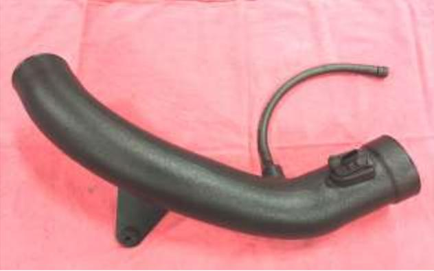
a. Assemble the intake tube according to the diagram on pg2. Reuse the factory MAF sensor screws and rubber grommet in the plate bracket. Trim the hose as needed.
