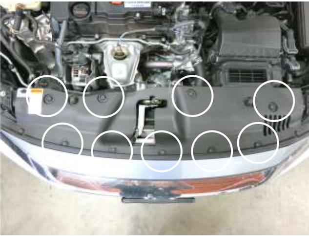
a. Remove the nine push-in clips, and remove the front shroud cover.
