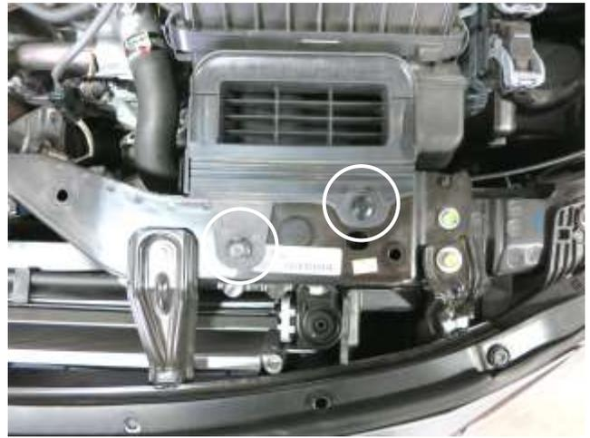
b. Remove the two push-in clips that secure the air box to the core support.
