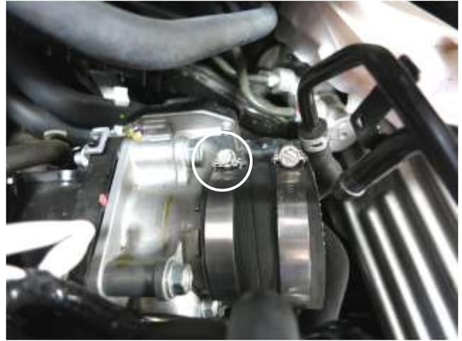
b. Install the provided coupler and hose clamps onto the throttle body. Tighten the circled hose clamp (30 in. lb.) at this time.
