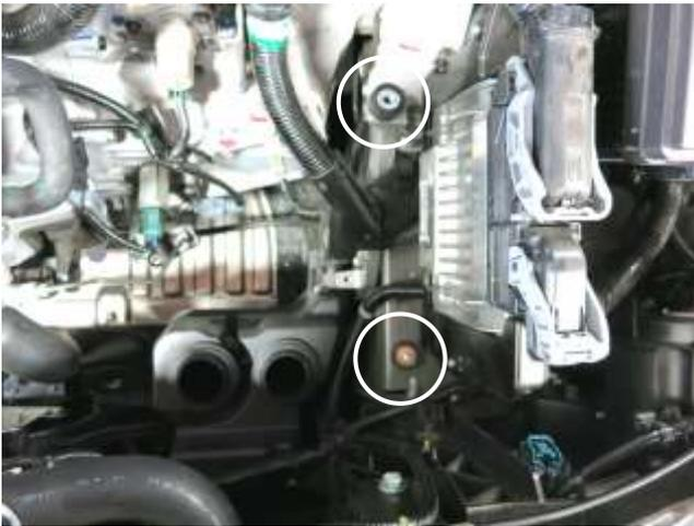
a. Install the two rubber mounts into the vehicle as shown.
