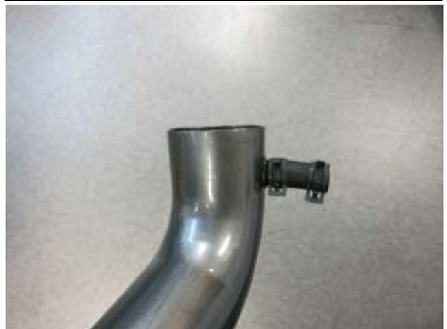
d. Install the provided hose and spring clamps onto the AEM intake tube. Trimming to 1.5" may be necessary.
