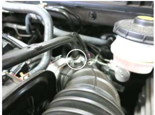
d. Squeeze the spring clamp on the vent line and remove the vent line from the stock intake tube.
