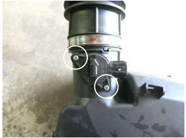
l. Remove the two screws and pull the MAF sensor from the stock upper air box. They will be reused in step 3c.
