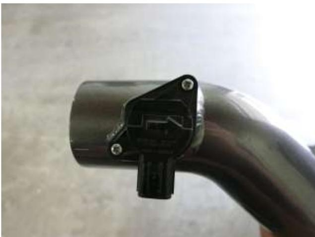
c. Install the MAF sensor into the AEM tube with the hardware that was removed in step 2l.
