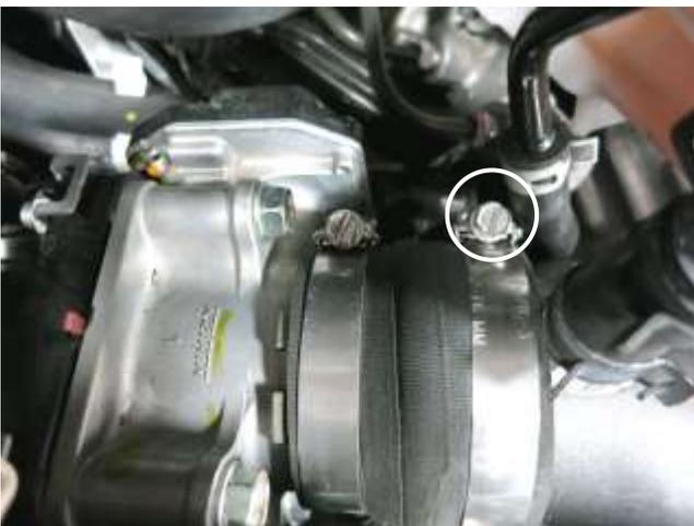
o. Once the AEM intake tube is properly aligned with the coupler and the heat shield, tighten the circled hose clamp (30 in. lb.).
