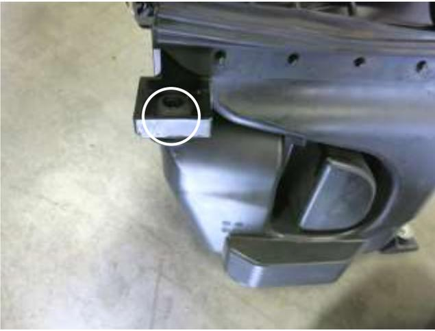
k. Remove the grommet from the lower air box. This will be reused in step 3f.
