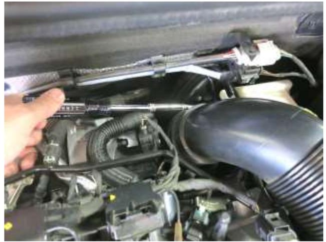
b. Loosen the hose clamp at the turbocharger and disengage the intake hose from the turbo inlet.
