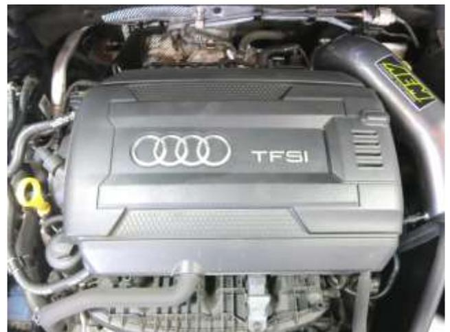
h. Reinstall the plastic engine cover by lining up the grommets with the posts and pressing down gently.
