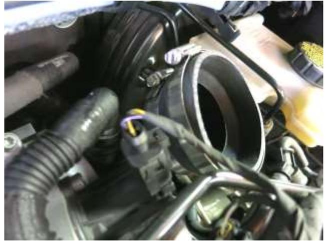
b. Install the provided coupler and hose clamps onto the turbo with the small end towards the turbo inlet. Tighten the turbo-side hose clamp to 30in-lb at this time.
