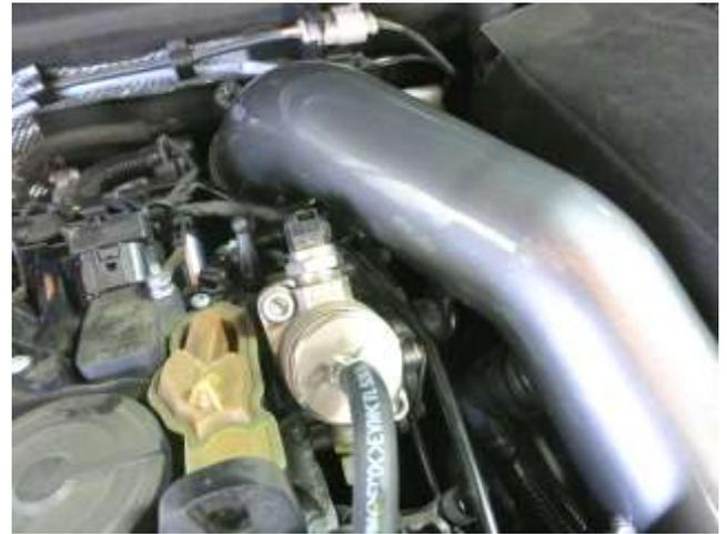
f. Lower the AEM intake tube bracket onto the rubber mount, between the washer and rubber mount, and insert the tube into the coupler. Do not tighten the mount or coupler at this time.
