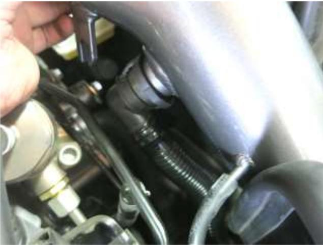
e. Position the AEM intake tube in the engine bay and connect the small vacuum hose to the small nipple. Move the large air injection hose behind the AEM heat shield and connect it to the AEM intake tube. Soapy water should be used to help installation. Note: Not all models have this large hose. Install the included blind plug (8-215) in its place.
