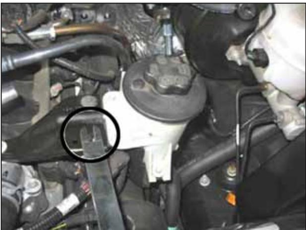
r. Align the top bracket over the threaded hole in the steering pump fluid reservoir bracket.
