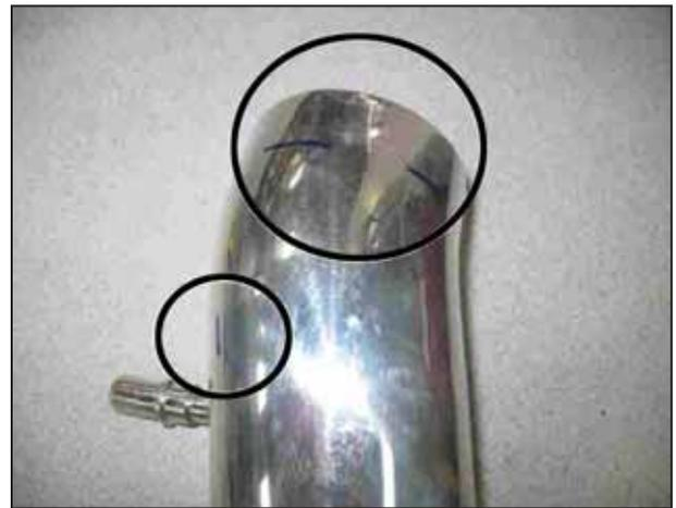
k. Mark a line 1" from the end of the inlet tube and 2" from the nipple, on the outside of the bend.
