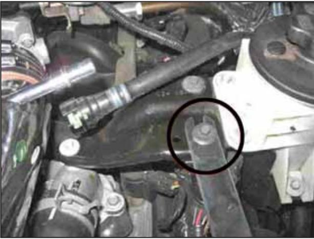
t. Loosely secure the top bracket with the bolt removed in 3o.
