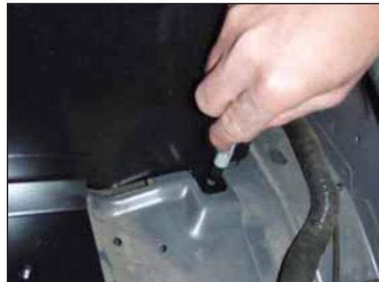
e. Place the heatshield into the engine bay aligning the two holes located on the bottom face of the heat shield with the two bolts installed in step 3d. With a marker, mark the location of the third hole.
