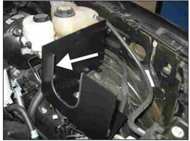
i. Install the rubber edge trim on the pipe opening on the heatshield.
