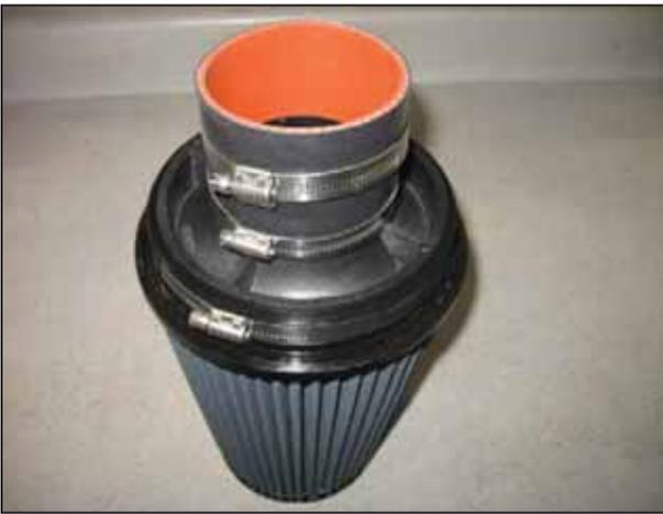
v. Attach the 5-350 hose to the air horn and secure with #56 hose clamp. Place another #56 hose clamp on the other side of the hose.
