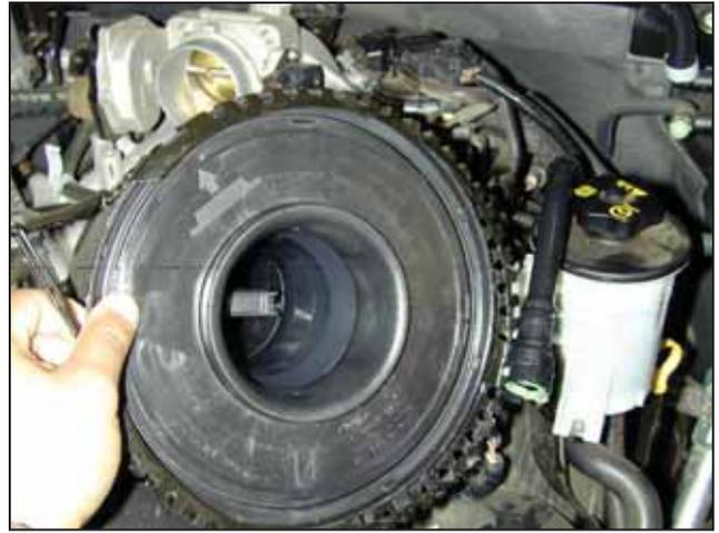
f. Gently pry open the housing at the any one of the tabs. Be careful not to damage the MAF sensor.
