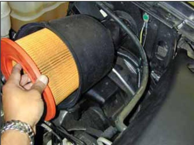
i. Remove filter element and housing. Gently pull up on the housing to remove.
