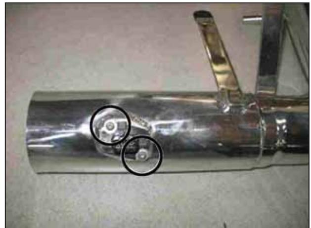
m. Install the mass airflow sensor into the straight section of the inlet pipe. Use the two factory torx bolts to secure the sensor.
