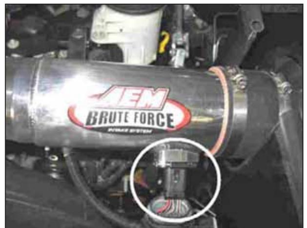
y. Reconnect the mass airflow sensor harness to the mass airflow sensor and lock it.
