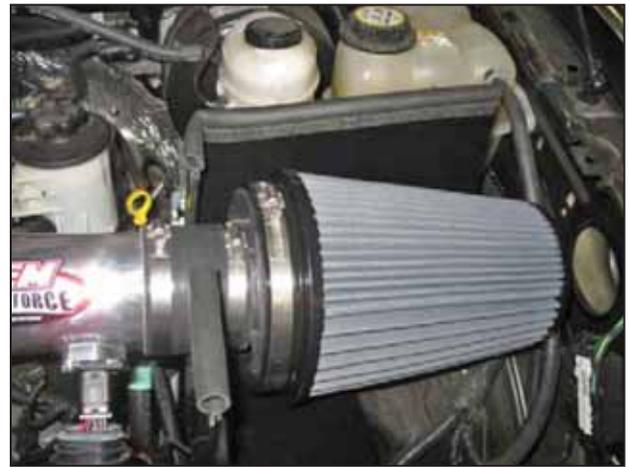
w. From inside the heat shield, slide the filter assembly over the inlet pipe and loosely secure with #56 hose clamp.
