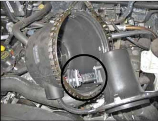
g. Disconnect the MAF sensor connector from the MAF sensor. Be careful not to damage MAF sensor harness.
