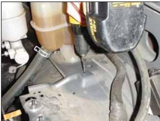
f. Remove the heatshield and drill a 1/8" pilot hole where you marked the engine bay in step 2e.
