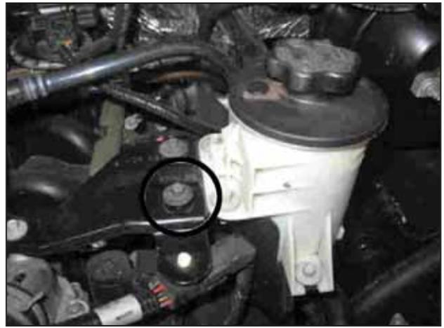
o. Remove the front bolt from steering pump fluid reservoir bracket.
