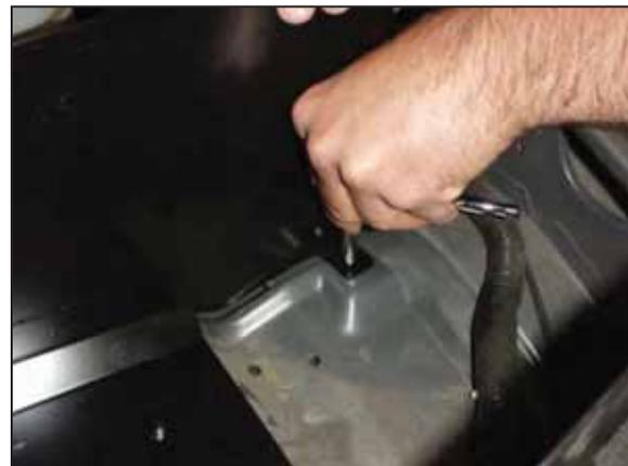
g. Place the heatshield in the engine bay and screw in the supplied self tapping screw.
