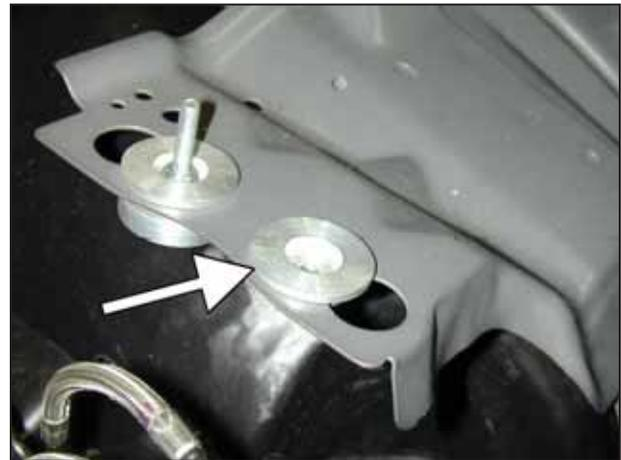
c. On the left is a fully assembled anchor for the heat shield. On the right, insert the upper spacer into the stock housing mounting surface.
