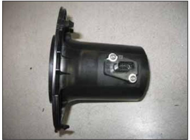
h. Remove the mass airflow sensor from the air box using the supplied torx tool (Be sure to keep the sensor in a safe place to be used later).
