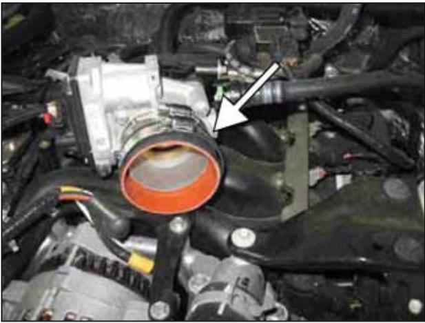
n. Attach the 5-326 hose to the throttle body and loosely secure with hose clamp #52. Place another #52 hose clamp on the other side of the hose loosely.
