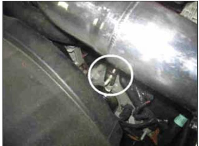
q. Align the bottom bracket over the stud protruding from the left hand cylinder head.
