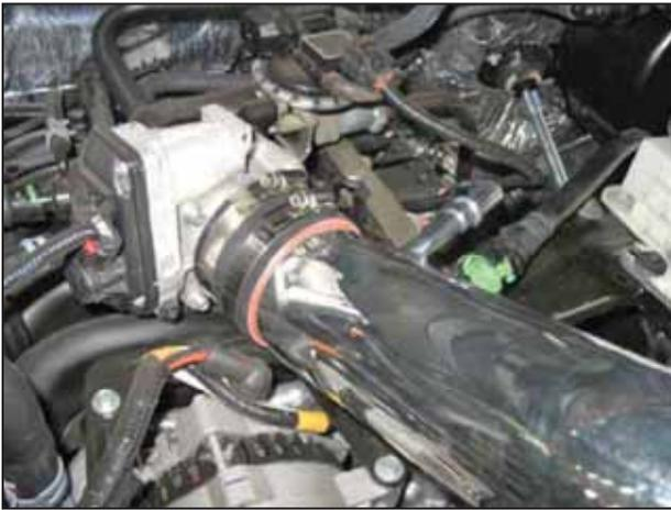
p. Insert the inlet pipe (patch end) into the 5-326 hose and loosely secure with #52 hose clamp.
