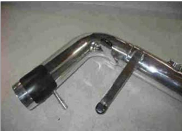
l. Apply rubber patch from the line marked in 3k. on the outside of the bend. Make sure to place the patch on the underside of the tube.
