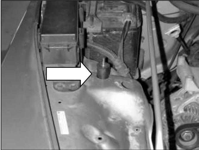
b. Install the rubber soft mount in the fender well using the supplied washer and M8 locknut.
