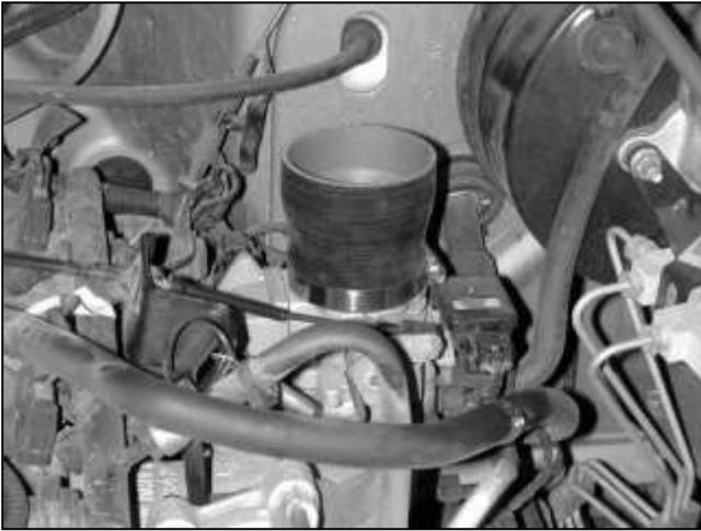
f. Install the small end of the silicone coupler on to the throttle body and secure with the #40 hose clamp. Insert the AEM<sup>®</sup> inlet tube in to the silicone coupler and loosely secure with the #48 hose clamp.
