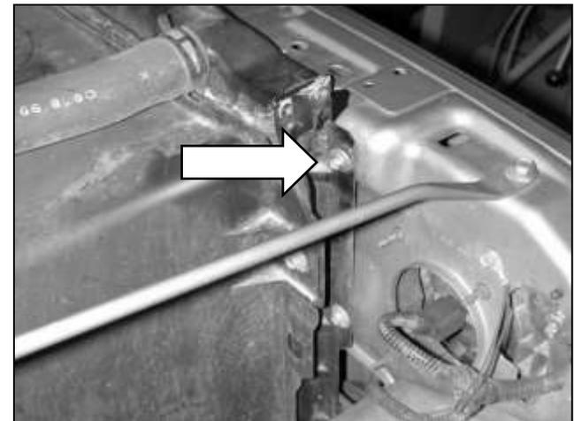
h. Remove the upper, passenger-side radiator mounting bolt. This bolt will be reused to mount the AEM® heat shield.
