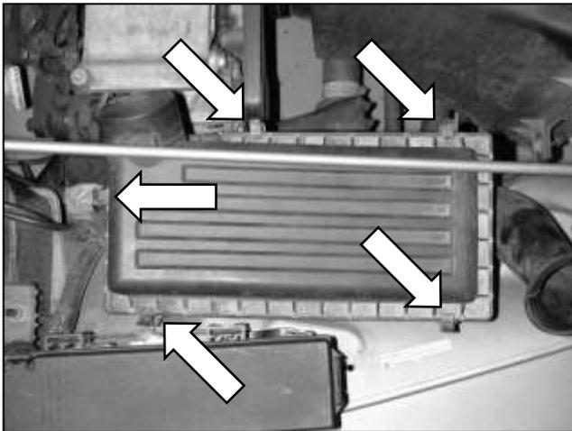
e. Remove five metal clips securing the top of the filter box to the lower filter box. Remove the filter box top from the vehicle.
