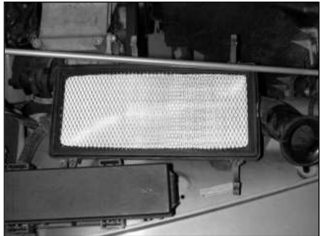
f. Remove the air filter element from the lower filter box.
