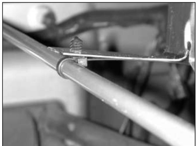
e. Use the supplied mounting zip tie to secure the upper heat shield tab to the radiator support rod. Make sure the locking head of the zip tie is on the engine side of the support rod.
