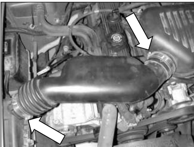
a. Loosen the hose clamps on both sides of the air inlet tube. Remove the tube from the vehicle.
