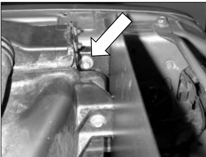
d. The front mounting tab will line up with the radiator mounting bolt removed in step 2h. Use the original bolt to secure heat shield.
