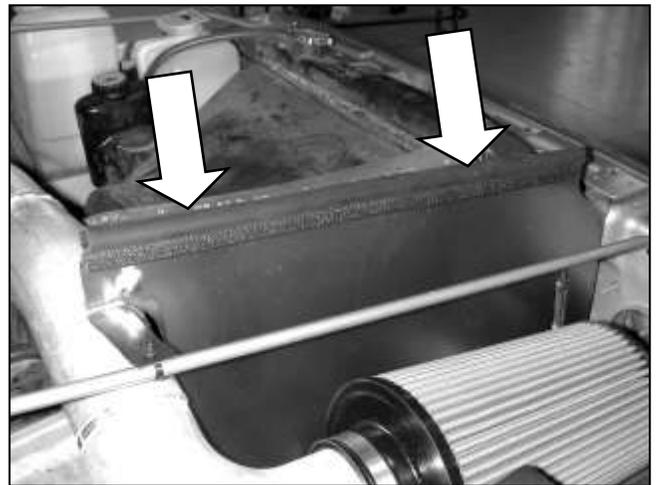
i. Install the supplied rubber gasket material to the top of the AEM<sup>®</sup> heat shield. The material may need to be trimmed to length for proper fitment.
