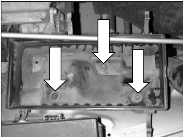
g. Remove the three bolts securing the lower filter box. It may be necessary to hold the nuts on the tire side of the fender to prevent them from turning. Remove the lower filter box and retaining nuts from vehicle.
