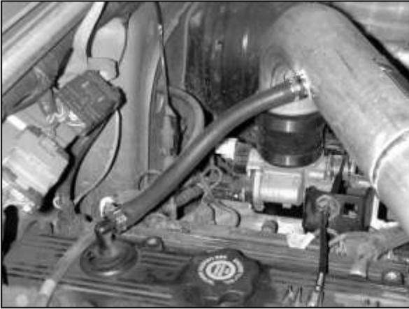
j. Install the supplied breather hose between the valve cover and the AEM® inlet tube. Secure the hose with the two supplied hose clamps.
