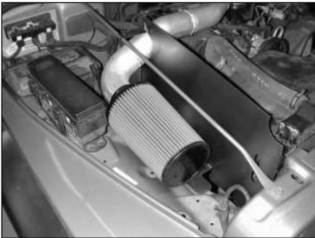
h. Install the AEM<sup>®</sup> air filter on to the end of the AEM<sup>®</sup> inlet tube. Secure with the supplied hose clamp.
