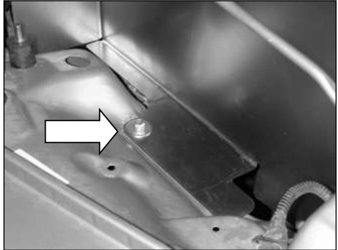
c. Install the AEM<sup>®</sup> heat shield and loosely secure using the supplied M8 bolt, locknut and two washers.
