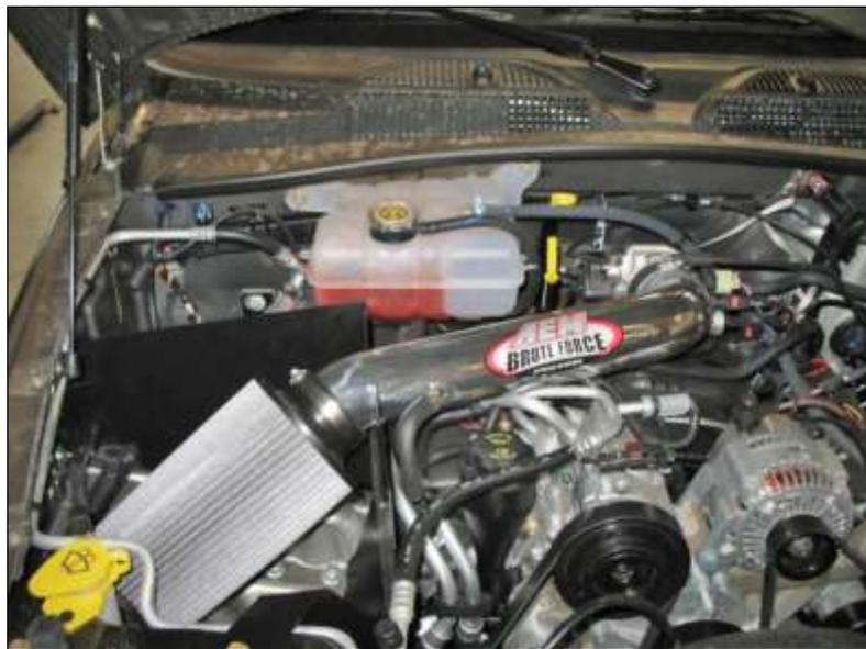
AEM® intake system installed
