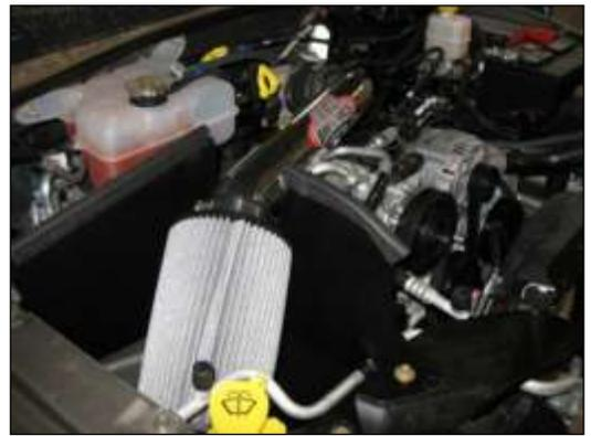
m. Attach the air filter and secure with a hose clamp once properly aligned. Attach the rubber edge trim to the top of the heat shield as shown.
