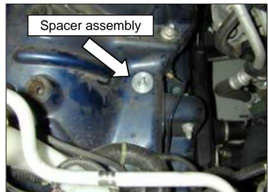
c. Mount the spacer assembly in the lower rubber mount left by the bottom of the airbox. The spacer assembly consists of the following: bolt, washer, spacers and nuts. Refer to the diagram on next page.
