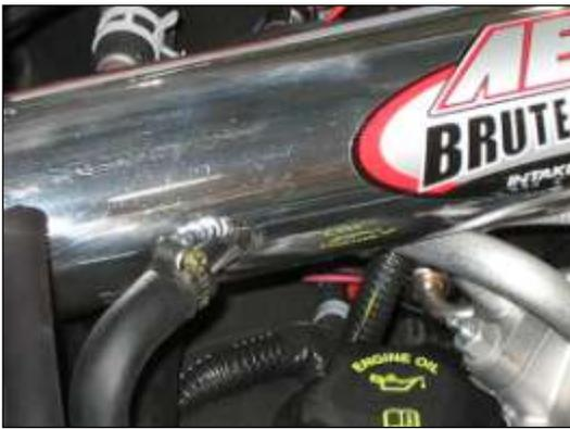
l. Rotate the breather hose 90° clockwise. Reattach the crankcase breather hose. Secure with the provided hose clamp.
