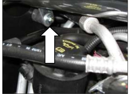
k. Secure the inlet pipe bracket to the rubber mount with a 8mm washer and a nut.
