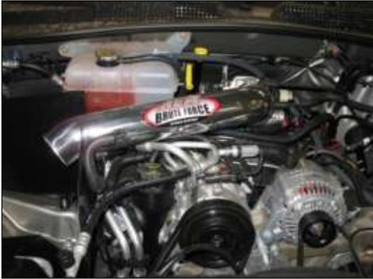
j. Insert the inlet pipe as shown. Align the mounting bracket with the rubber mount on the heat shield.
