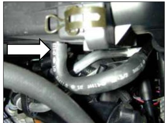
b. Disconnect the crankcase breather hose from the airbox. Remove the airbox by pulling straight up.
