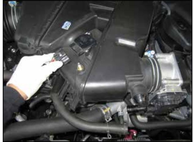
b. Loosen spring clamp to disconnect breather hose from plastic elbow. Disconnect MAF sensor harness from sensor.
