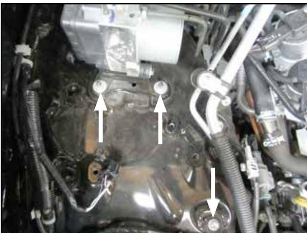
i. Remove the two nuts and one bolt indicated. Set aside for use later with AEM heat shield.
