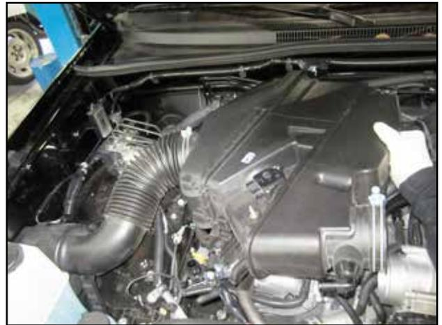
h. Disconnect air box from throttle and carefully remove stock assembly from the engine bay.
