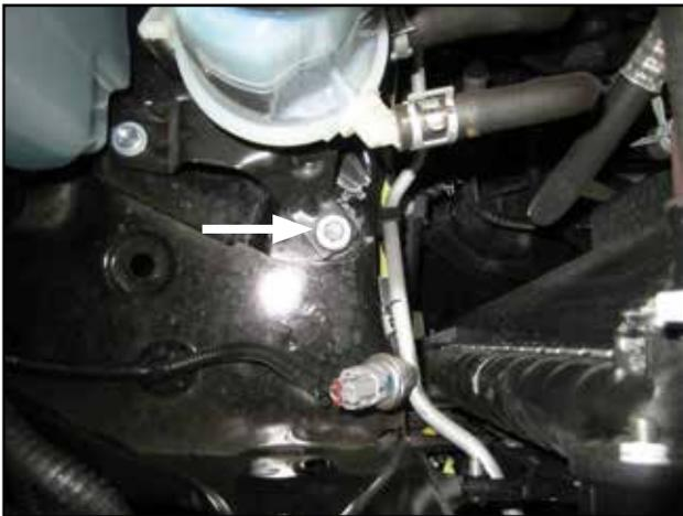
h. Remove the bolt indicated above on the power steering reservoir bracket and set aside for use in the next step.
