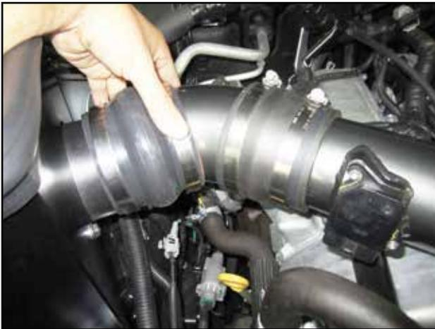
q. Slide transition coupler(K) end onto upper tube and tighten hose clamp. Position and slide hump hose over air horn collar as shown.
