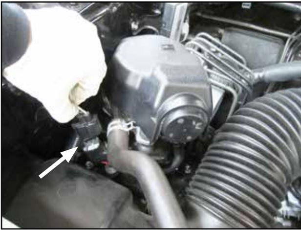
e. Disconnect harness on air pump bracket. Remove the three M6 bolts securing the air pump bracket and set assembly aside.
