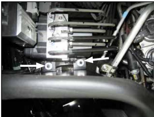
n. Secure rear tabs using the stock nuts from removal Step 2-i.
