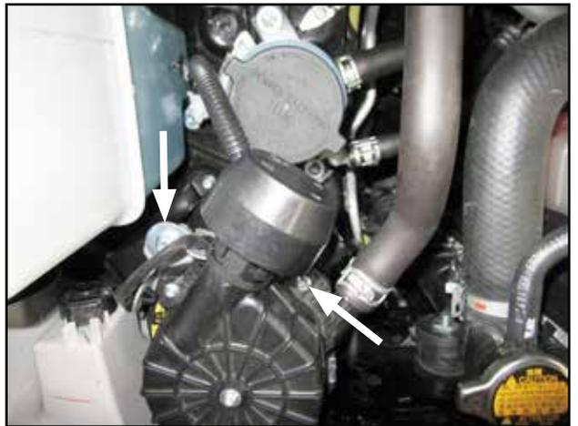
i. Re-install bolt removed in previous step to secure air pump bracket on right. Line up left bracket to inner fender hole and insert provided bolt(H) through bracket hole.
