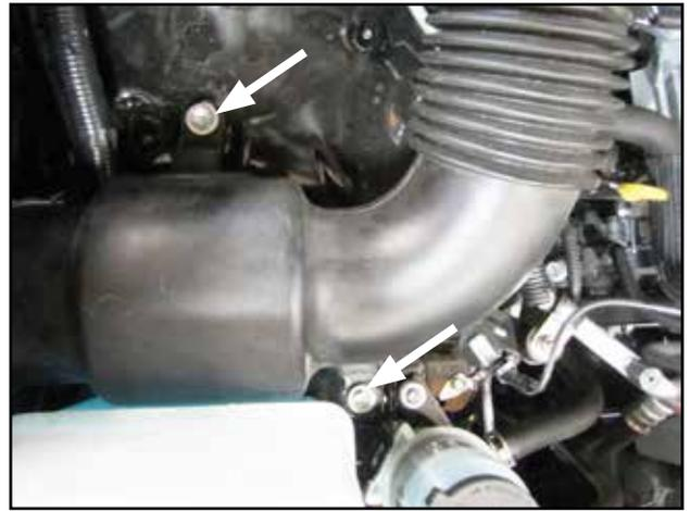
f. Remove the two bolts securing the stock intake inlet tube down.
