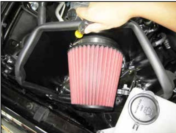
s. Install filter(U) onto air horn and secure with the provided hose clamp(A).
