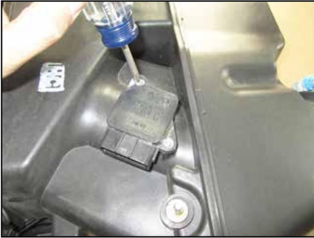
k. Remove the MAF sensor from the stock airbox and set aside for use with the AEM upper tube.
