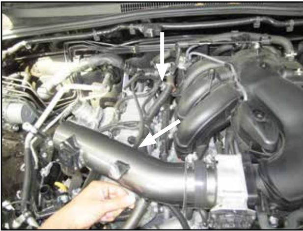
f. Replace fuel pressure regulator hose with the longer hose(V) provided and connect other end to the AEM tube(T) as shown. Reconnect crank case vent hose to the nipple and fasten with stock spring clamp.
