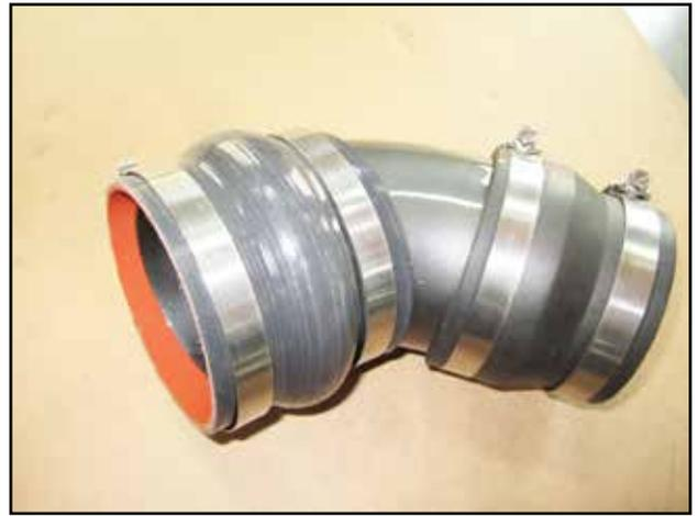
p. Assemble lower tube(S) using components provided(L,B,K,C). Use a soap/water mixture to slide hump hose(L) closer to bend.
