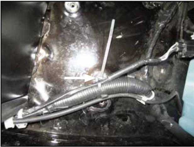
o. Provide adequate slack to pump harness and use zip tie(W) to secure harness to inner fender as shown. Trim excess end of zip tie.
