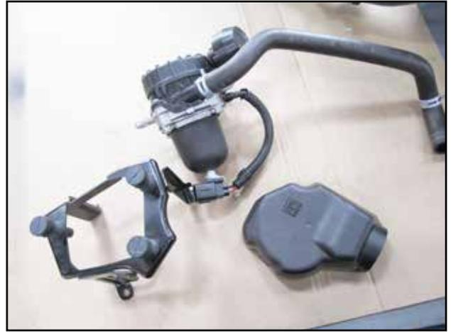
l. Remove air pump cover. Disconnect wire harness from bracket. Slide off rubber grommets to separate pump from bracket.
