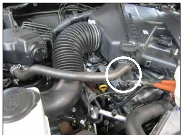
d. Loosen spring clamp and disconnect air pump hose as shown.
