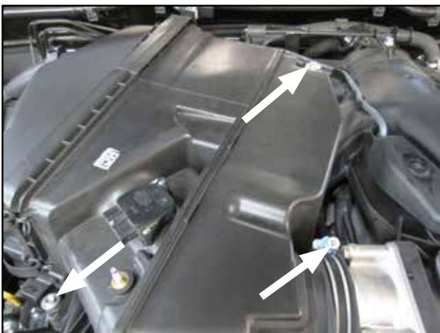
c. Loosen and remove the two 10mm bolts securing the airbox. Loosen the hose clamp on throttle body.
