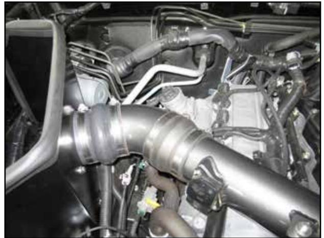
r. Ensure that hump hose is seated against heat shield and rotate lower tube into position. Tighten all four hose clamps.
