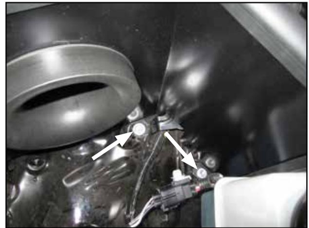
m. Carefully install heat shield and line up tabs to holes exposed in removal Step 2-i. Fasten lower tab near air horn using stock bolt from removal Step 2-f. Fasten tab near washer reservoir using bolt from removal Step 2-i. Reconnect air pump harness.
