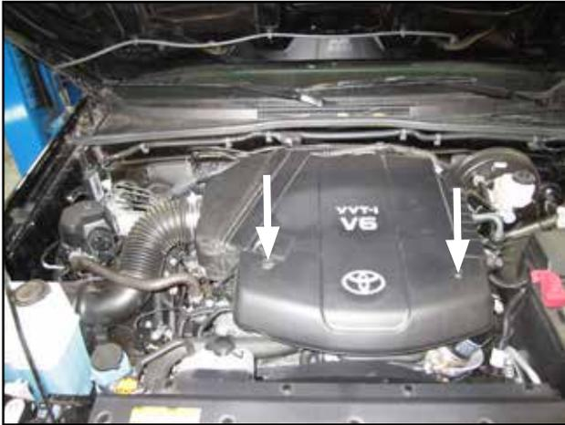
a. Stock intake system. Loosen the two nuts indicated to remove the engine cover.
