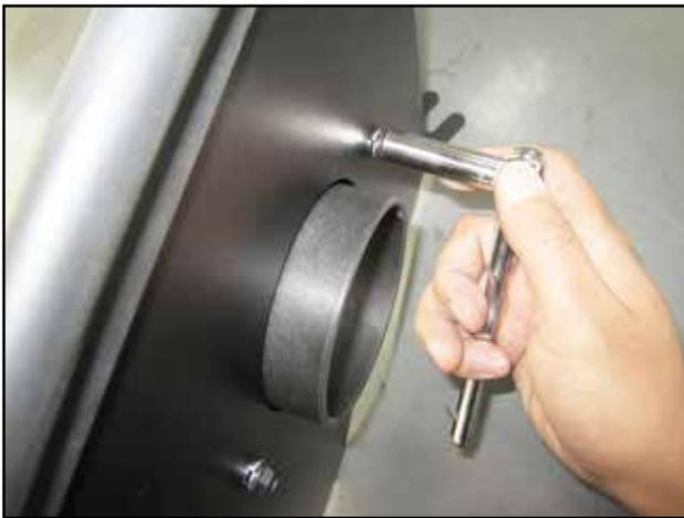
l. Mount air horn adapter(R) onto heat shield and secure with lock washers(E) and bolts(F) provided.
