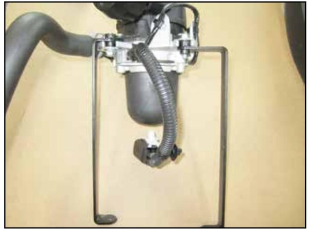
g. Loosely mount brackets(N,O) onto air pump as shown using provided bolts(H) and washers(J). Note: Short armed bracket is mounted on left side near hose as shown with bolt pointed upward.
