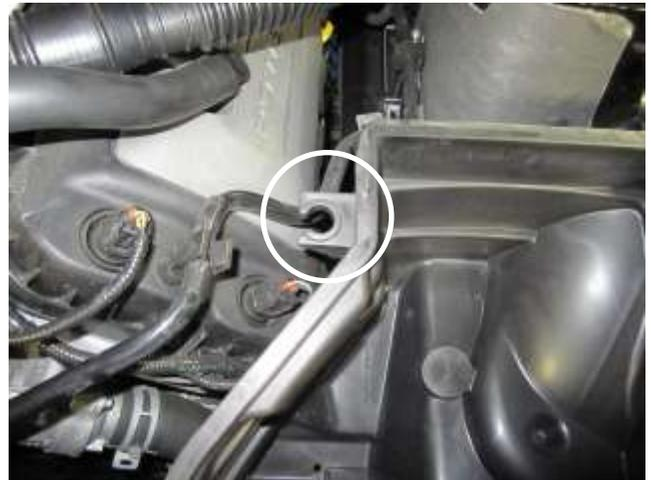
h) Remove the engine pulse sound tube rubber clamp from the air box by gently sliding it out of the "C" clip. **Note:** This will not be reused.
