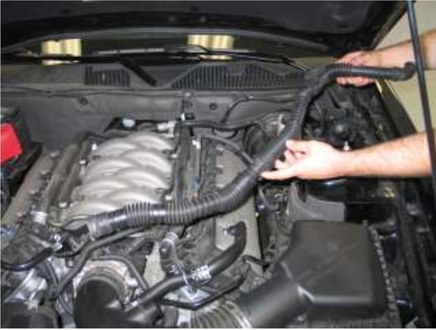
e) Remove the engine pulse hose from the vehicle. This will not be reinstalled. **Note:** Do not discard any of your stock equipment.
