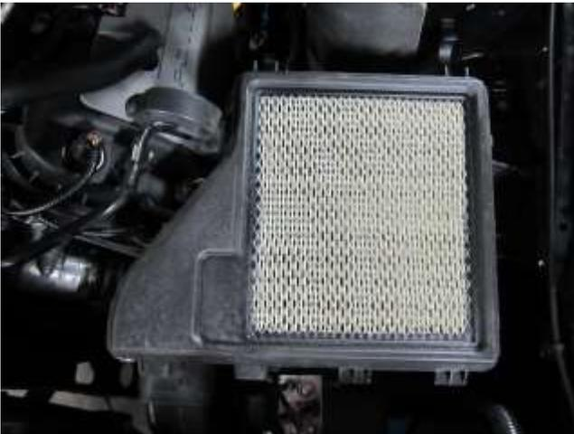
g) Remove the stock filter from the air box.
