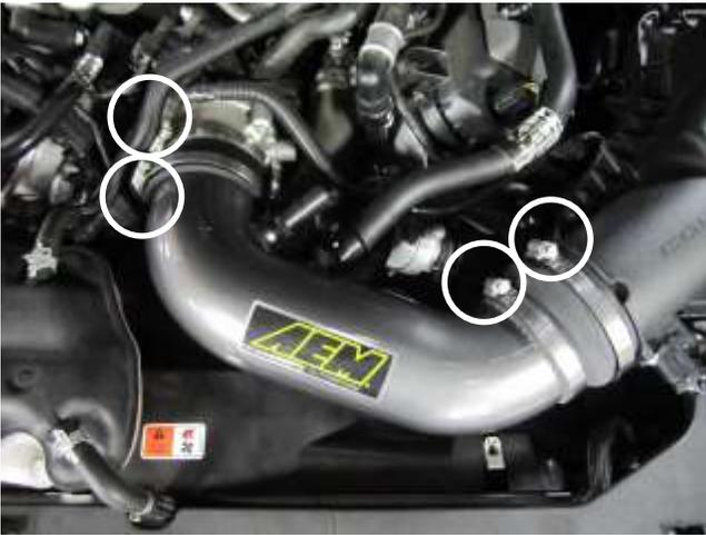
e) Install the AEM tube with the proper fittings into the couplers. Tighten all four hose clamps at this time.
