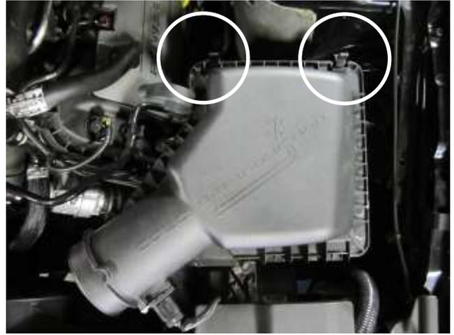
f) Un-clip the hinges on the air box and access the filter.
