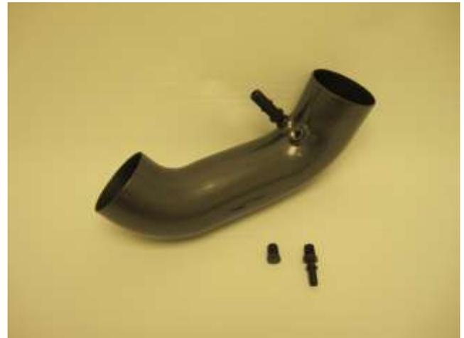
d) Screw in the fitting (082628) into the top port. For the bottom port reference your transmission below:
