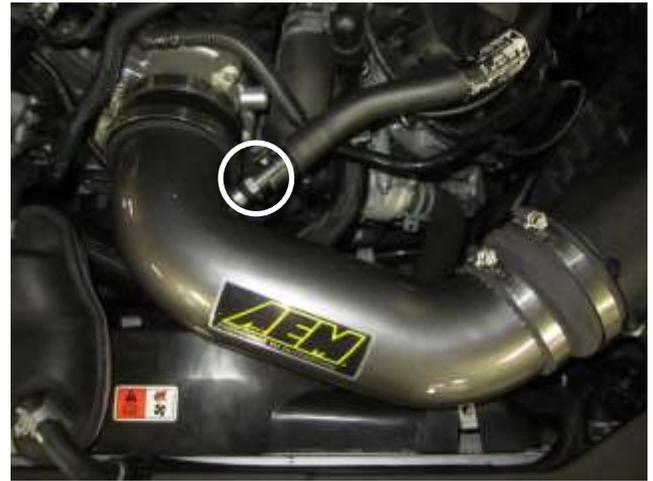
f) Attach the valve cover breather hose by sliding it over the fitting. On automatic transmissions also attach the second hose removed in 2b) to the lower fitting. **Note:** Make sure you hear it click as it attaches to the fitting.
