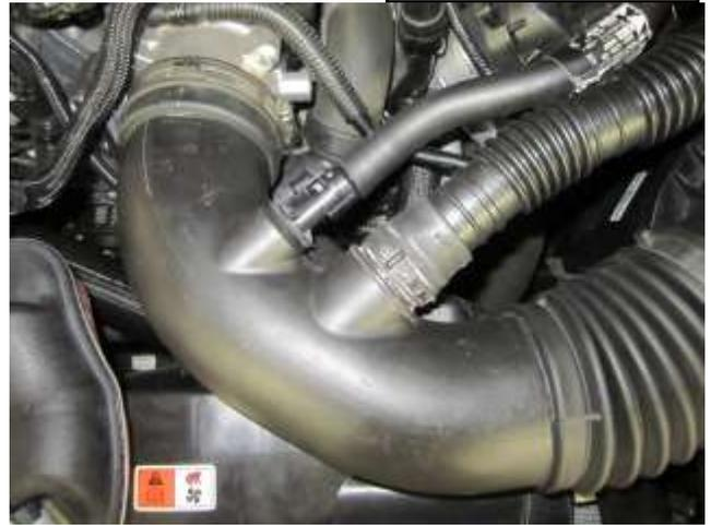
b) Disconnect the engine pulse tube by squeezing the clamp and sliding it off the intake tube. Slide the grey indicator on the valve cover breather hose and detach it from the intake. **Note:** On automatic transmission vehicles, there will be an additional vent line. Depress the yellow tab and slide the line off.
