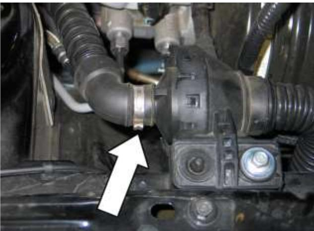
c) Cut the clamp that secures the engine pulse hose to the drum and disconnect the hose from the drum.
