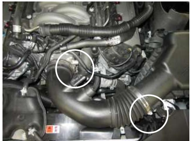
d) Loosen the two hose clamps at the air box and throttle body and remove the stock intake tube. **Note:** Do not discard any of your stock equipment.
