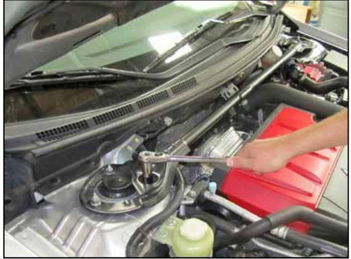
b. With the car on the ground, Use a 14mm socket to remove the (6) strut top nuts
