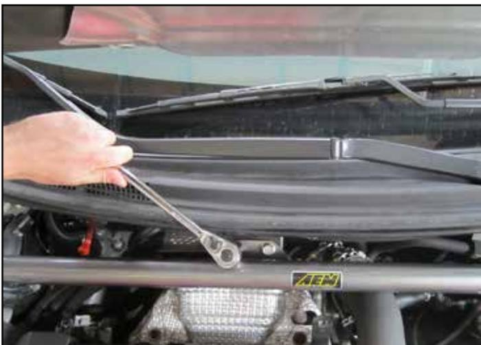
c. Using a 14mm socket, replace the firewall bolts
