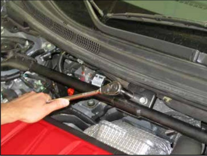
a. Using a 14mm socket, remove the (2) bolts holding the stock strut bar to the firewall bracket
