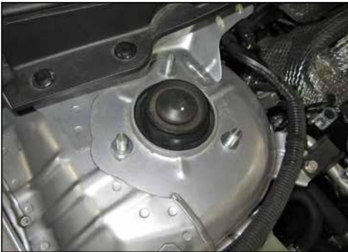
a. Place the (6) washers over the strut top studs
