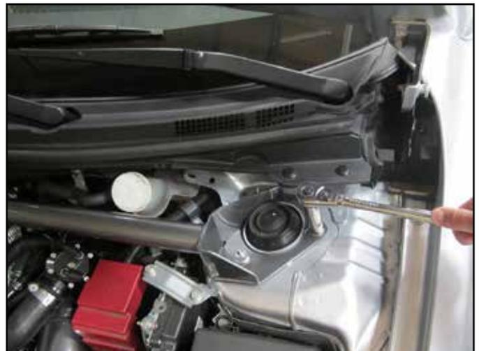
d. Using a 14mm socket, replace the strut tower nuts
