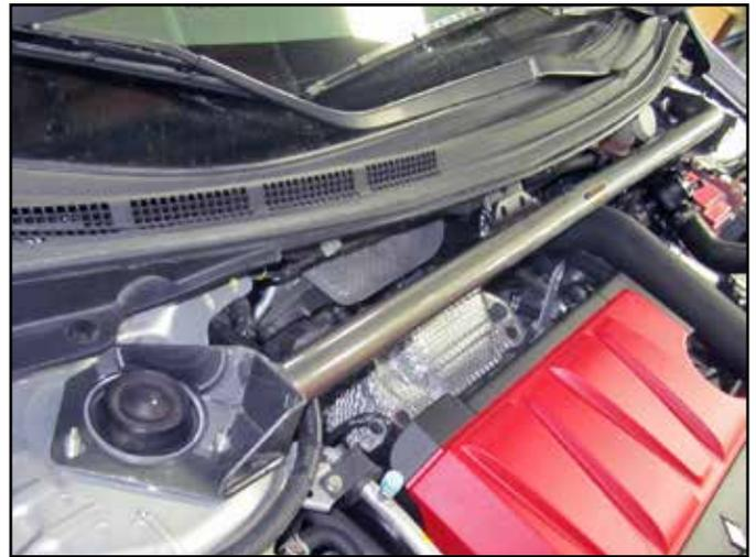
b. Place the AEM strut tower over the strut tower studs
