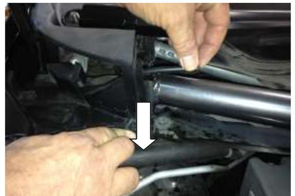
d. Make sure the windshield washer tubing is not pinched between the finisher and the strut tower bar.
