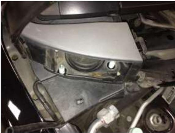
e. Using a 14mm socket, remove the (2) strut tower bolts, as shown.
