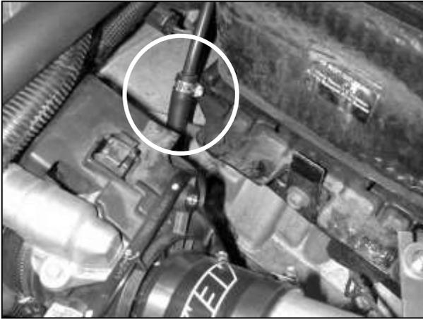
j. Remove the rubber elbow from the breather hose removed in step 2e. Replace it with the supplied breather hose. Install the breather hose and secure it with a hose clamp as shown.
