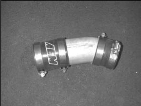
b. Install the 2.50" x 2.00" silicone hose on the shorter leg of the short AEM® intake pipe. Install one of the 2.50" x 3.00" silicone hoses on the longer leg of the same pipe. Loosely install two 2.50" hose clamps onto each silicone hose.
