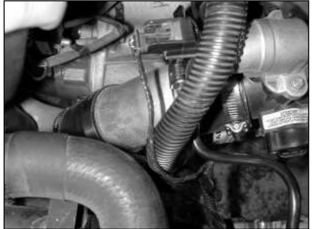
c. Install the short AEM® intake pipe between the intake manifold and the throttle body. The longer leg attaches to the intake manifold and the shorter leg attaches to the throttle body. Loosely tighten the hose clamps to hold the pipe in place, but do not fully tighten, as further adjustment may be needed.
