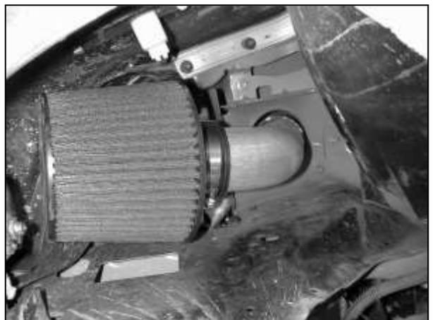
i. Install the AEM<sup>®</sup> air filter from the fender well of the vehicle. Position the air filter so that it is not in contact with any part of the vehicle, then tighten the hose clamp so it is secured to the intake pipe. Install the IAT sensor into the grommet installed in step 3f.
