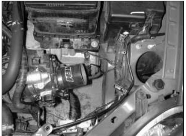
e. Install a 2.50" x 3.00" silicone hose on the throttle body and loosely secure with the remaining 2.50" hose clamps.
