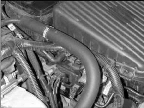
e. Remove the breather hose from the lower airbox. Remove the lower airbox from the vehicle.
