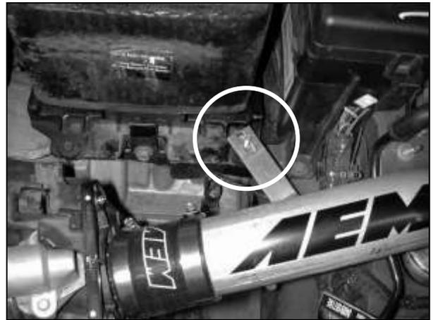
g. Install the lower intake pipe into the vehicle. Insert the intake pipe into the silicone hose on the throttle body. Loosely secure the hose clamps to secure the intake pipe in place. The bracket of the intake pipe should line up with the rubber mount installed in step 3d. Install the supplied washer and lock nut onto the rubber mount. Refer to the following diagram for proper installation of the assembly.
