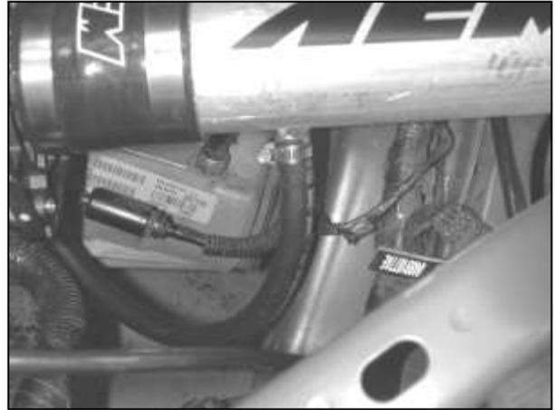
k. Connect the other end of the breather hose to the nipple on the AEM® intake pipe, secure in place with the remaining hose clamp. Route the hose carefully to prevent the hose from kinking.
