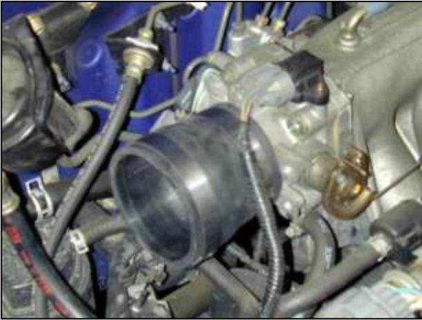
e. Install the reducing coupler onto the throttle body and secure using the #44 hose clamp.
