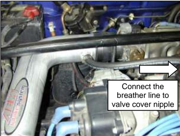
g. Install the AEM® inlet pipe into the vehicle and secure to the throttle body using a #48 hose clamp. Attach the supplied breather hose to the intake pipe's nipple; connect the opposite end to the valve cover's inlet. Secure each end of the breather hose in place with the two supplied hose clamps.
