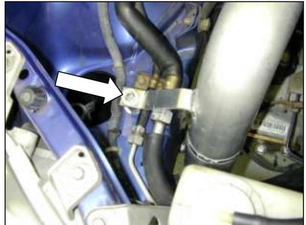
h. The intake pipe's mounting bracket will line up with the rubber mount installed earlier. Use the supplied serrated nut and washer to secure in place. See the diagram below for proper installation of the rubber mount.
