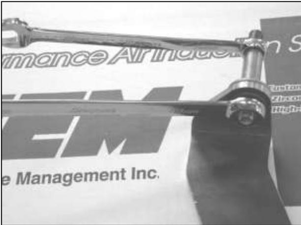
c. Install the factory mounting stud removed in step #3b through the supplied engine mount bracket. Secure in place with the provided nylock nut and washer.
