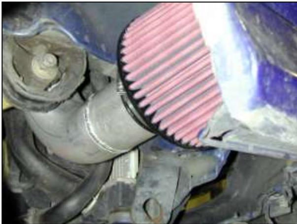
j. Install the AEM® air filter onto the inlet pipe. Once proper fitment is achieved, secure the air filter in place with the supplied hose clamp.
