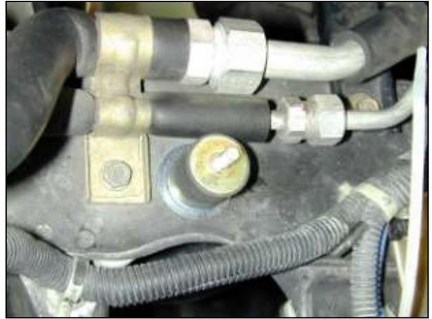
f. Install the supplied 1/4" spacer and rubber mount over the threaded hole located near the A/C line behind the passenger headlight. The 1/4" spacer should sit between the rubber mount and the body of the vehicle.
